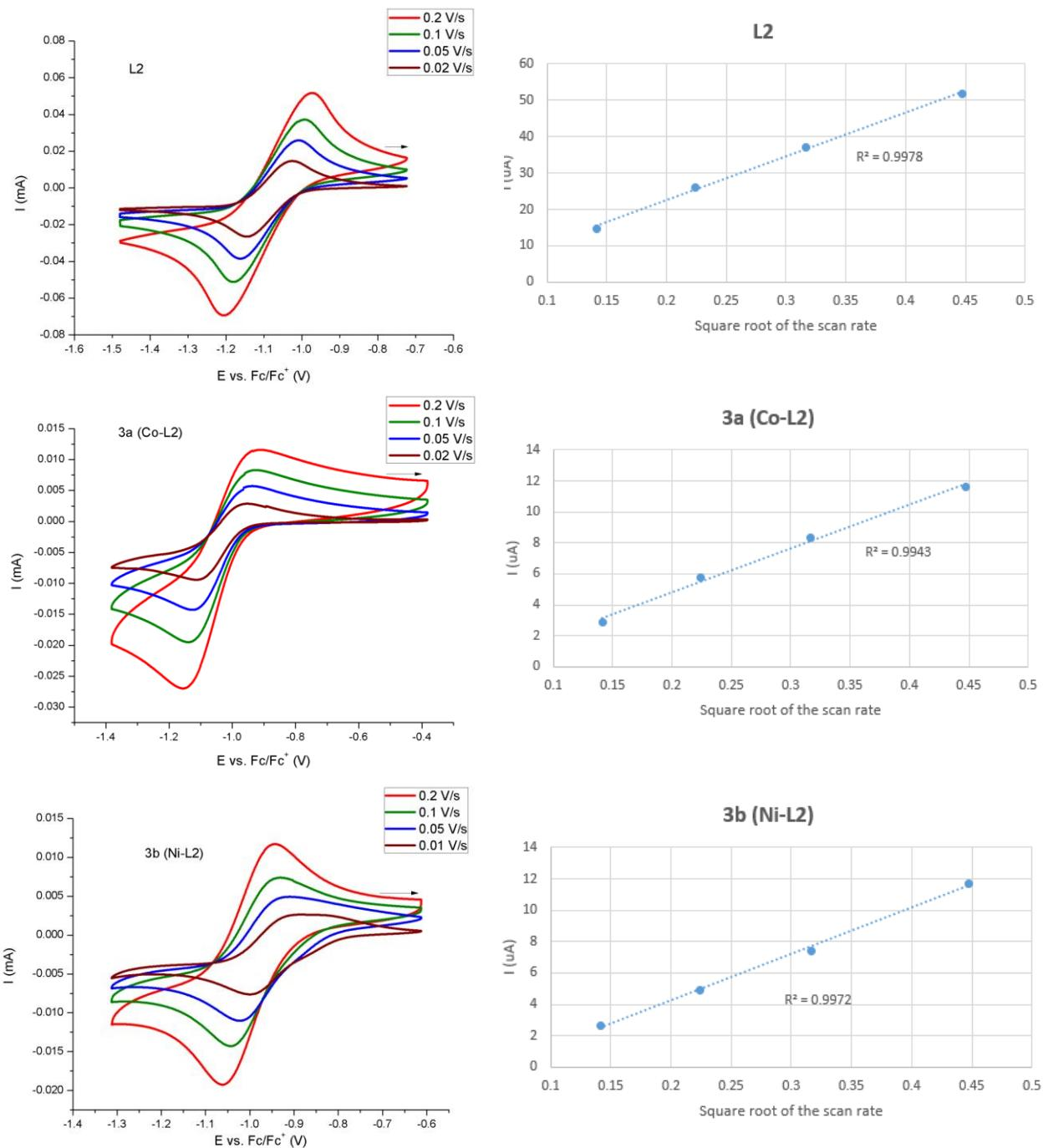
**Figure S7** CV curves of ligand **L2** (3 mM), complex **3a** (2 mM) and **3b** (1 mM) in DCM ([TBA][PF<sub>6</sub>] 0.1 M) solutions recorded at a glassy carbon working electrode with different scan rate and the corresponding reversibility plots of square root of the scan rate and current. E vs the Fc/Fc<sup>+</sup> redox couple.
