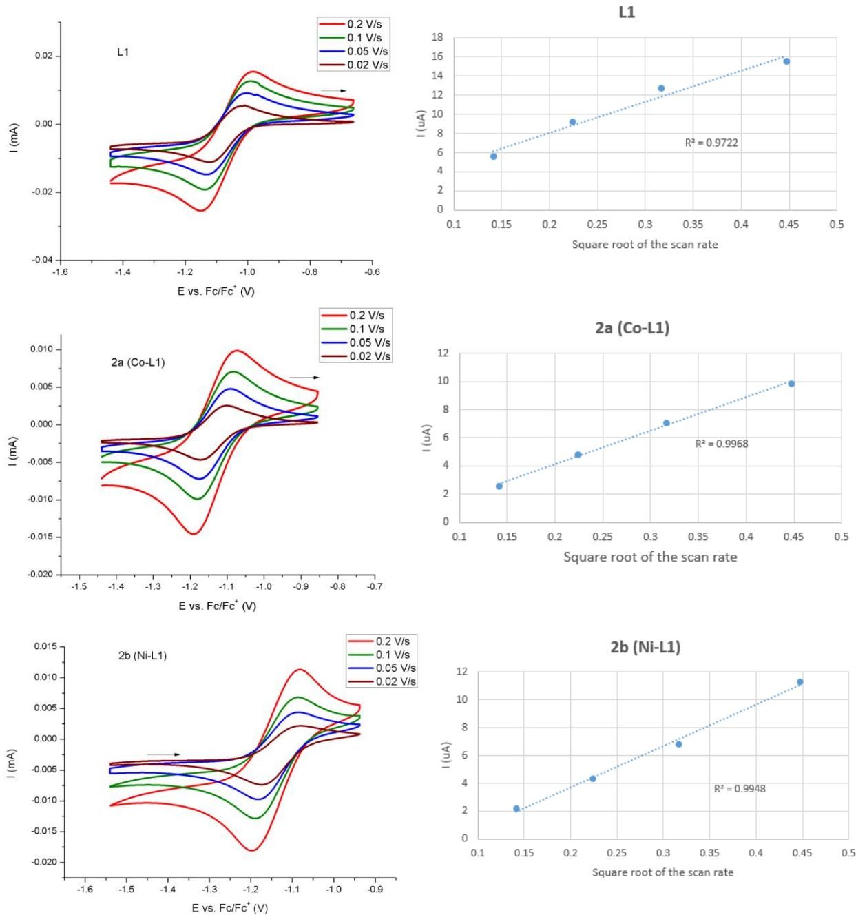
**Figure S6** CV curves of ligand **L1** (2 mM) and complexes **2** (1 mM) in DCM ([TBA][PF<sub>6</sub>] 0.1 M) solutions recorded at a glassy carbon working electrode with different scan rate and the corresponding reversibility plots of square root of the scan rate and current. E vs the Fc/Fc<sup>+</sup> redox couple.
