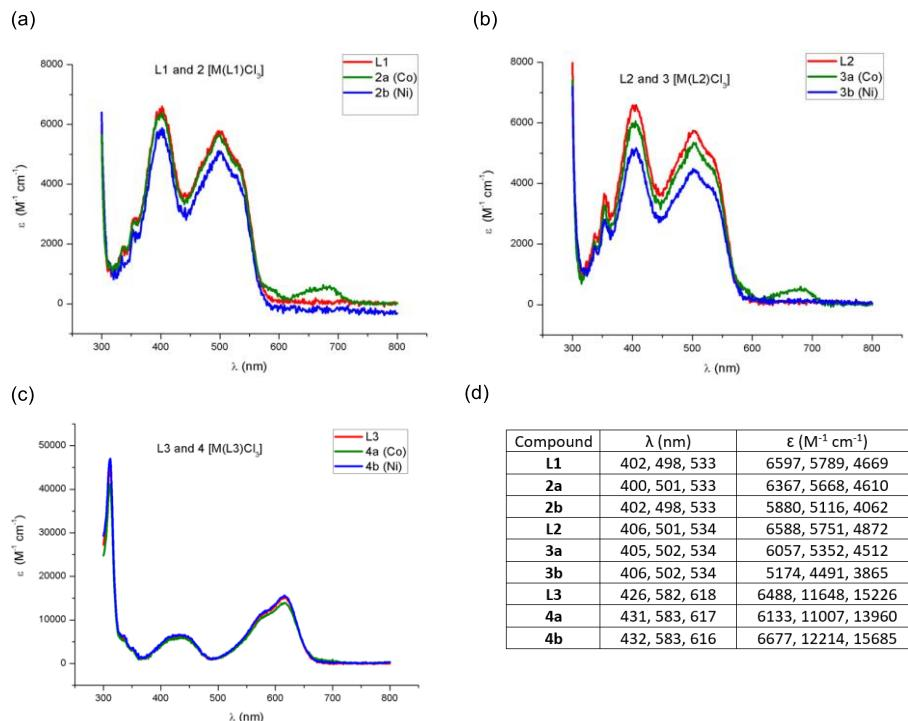
**Figure S9.** (a-c) Overlapped absorption spectra in MeCN (a) ligand **L1** and complex **2**, (b) **L2** and **3**, (c) **L3** and **4**, (d) photophysical properties of ligands **L1-L3** and complexes **2-4** in MeCN.
