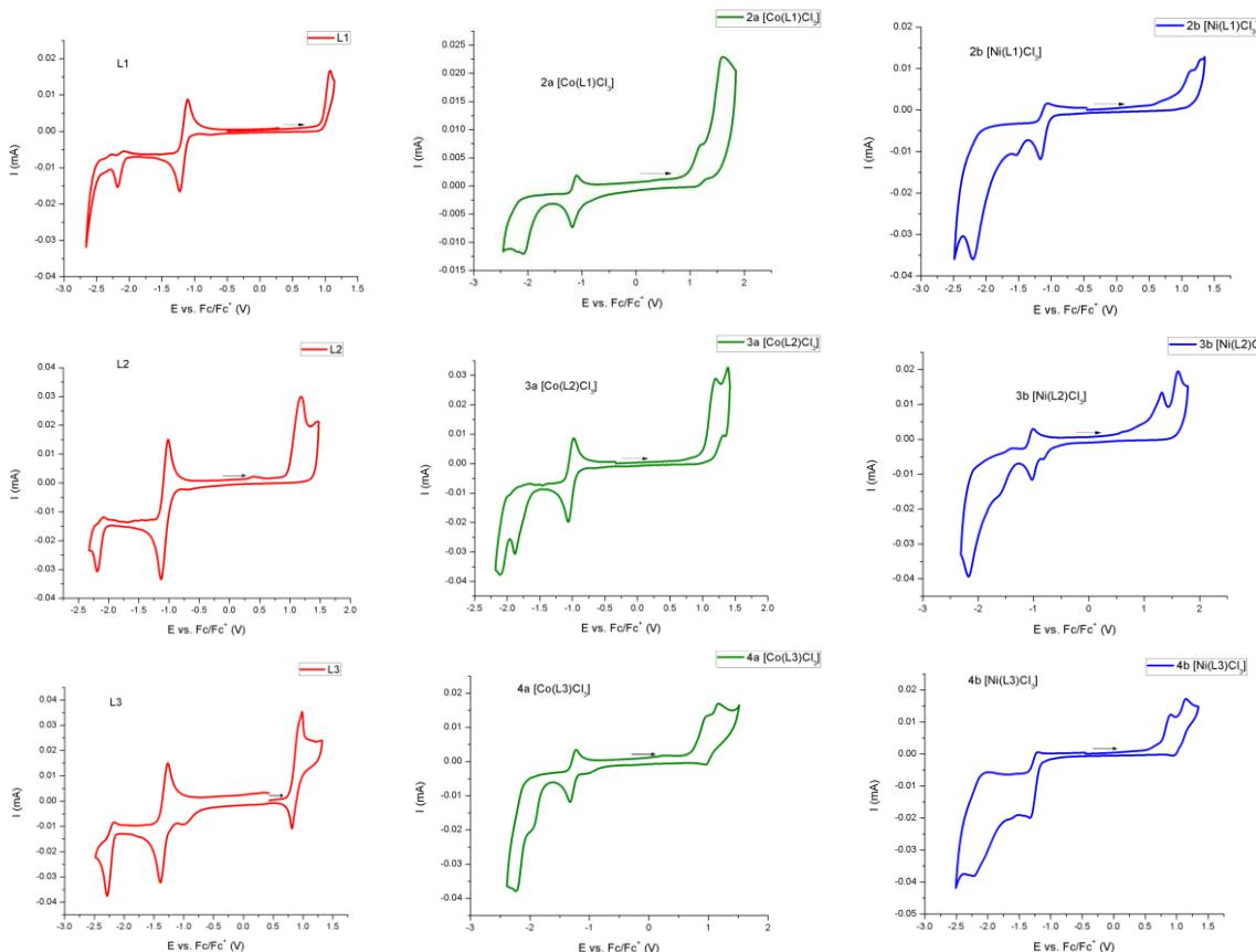
**Figure S5** Individual CV curve of ligand **L1** (2 mM), **L2-L3** (3 mM) and complexes **2-4** (1 mM) [2 mM for **3a**] in DCM ([TBA][PF<sub>6</sub>] 0.1 M) solutions recorded at a glassy carbon working electrode ( $v = 0.02$  V/s).
