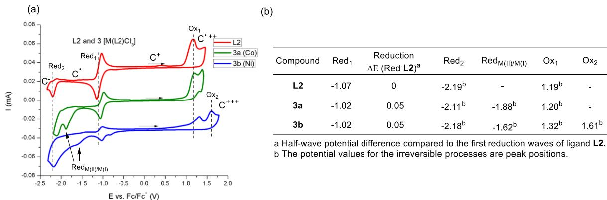
**Figure S4** (a) Selected CV curves of **L2** (3 mM) and complexes **3a** (2 mM) and **3b** (1 mM) in DCM ([TBA][PF<sub>6</sub>] 0.1 M) solutions recorded at a glassy carbon working electrode ( $v = 0.02$  V/s). (b) Oxidation and reduction half-wave potential values [V] measured by CV for **L2** and **3**,  $E$  vs. the ferrocene/ferrocenium redox couple ( $\text{Fc}/\text{Fc}^+$ ).
