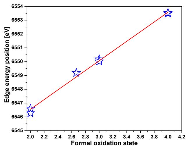
Fig. S6 Mn *K*-edge XANES of Mn<sup>II</sup>O, Mn<sup>II</sup>CO<sub>3</sub>, Mn<sub>3</sub>O<sub>4</sub>, Mn<sup>III</sup><sub>2</sub>O<sub>3</sub>, α-Mn<sup>III</sup><sub>2</sub>O<sub>3</sub>, Mn<sup>IV</sup>O<sub>2</sub> and β-Mn<sup>IV</sup>O<sub>2</sub> were measured as a reference to determine the oxidation state of **1** (initial compound) and after operation.
