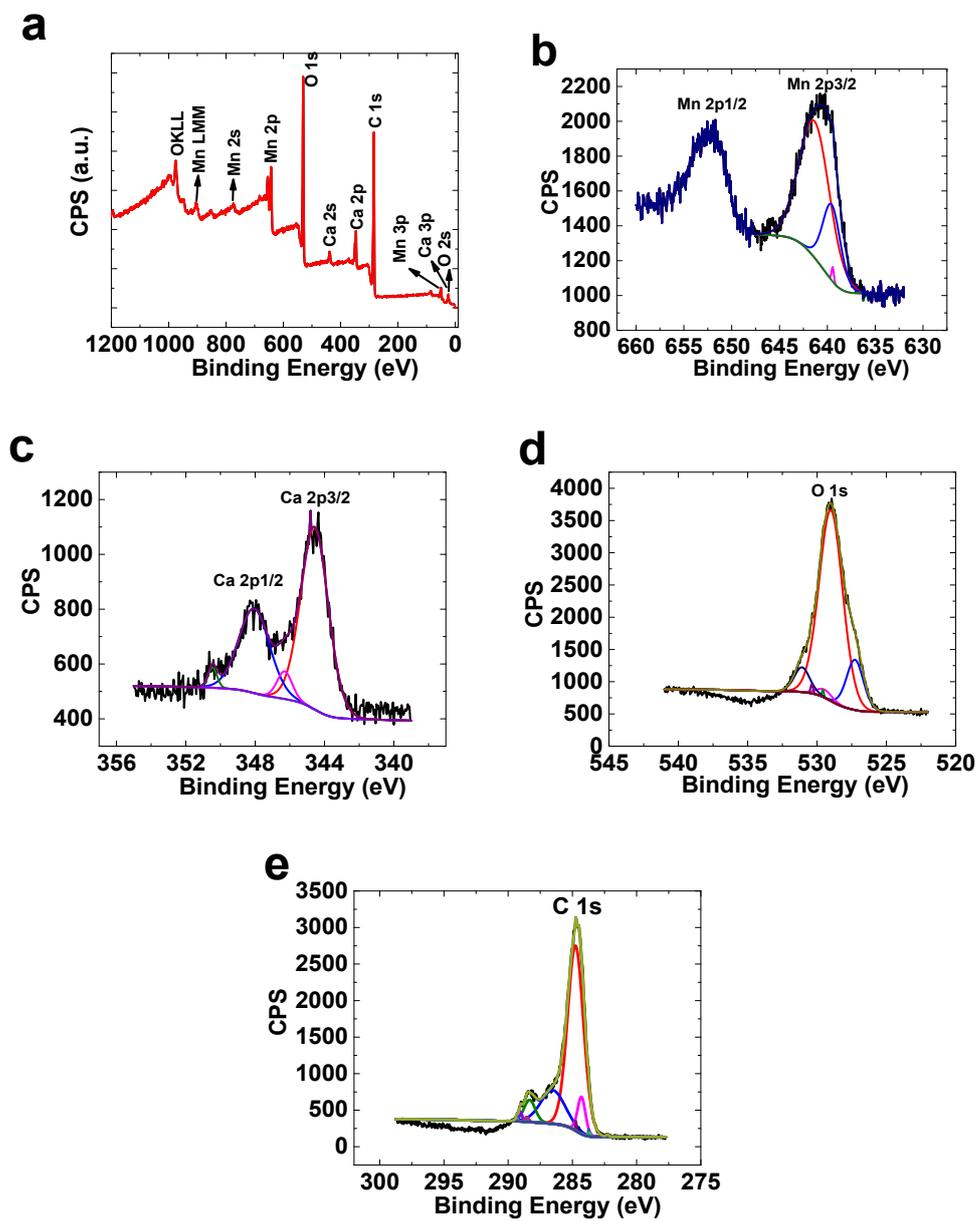
Fig. S3 XPS for **1** before water oxidation.
