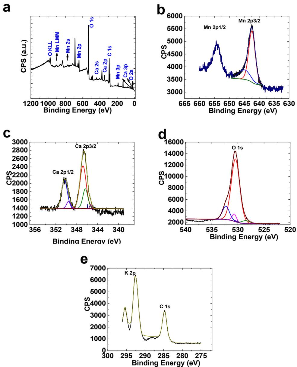
Fig. S4 XPS for **1** after the water-oxidation reaction. The amperometry was performed in the presence of **1** at 1.8 V in 25.0 mL of the phosphate buffer (1.0 M, pH=11.0).
