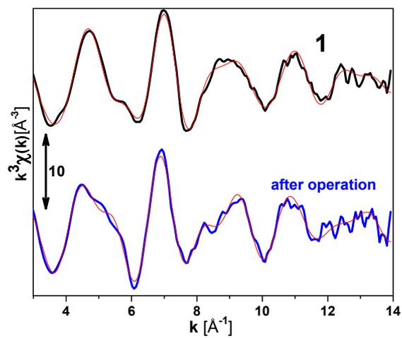
Fig. S7  $k^3$ -weighted  $\chi(k)$  of EXAFS spectra of **1** (black) and the obtained compound at 1.8 V the phosphate buffer (1.0 M, pH=11.0; blue). The thick lines and the thin red lines show the experimental data and simulations, respectively. The fit parameters for the simulations are given in Table S3. Phase shift not corrected.
