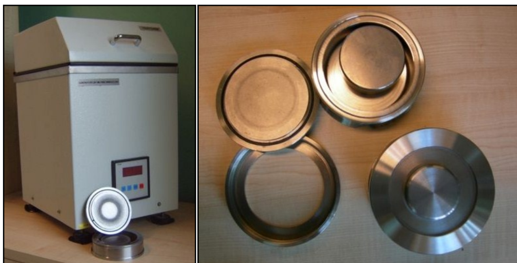
Figure S2. The LMW-S vibrational mill (left) and a stainless steel disc bowls (right) used for mechanochemical synthesis.
