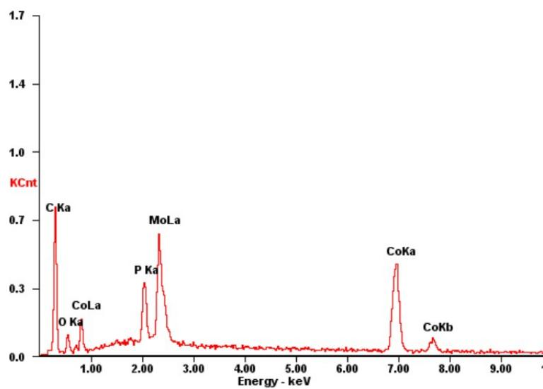
Figure S4. Typical EDS spectrum of Mo-CoP<sub>3</sub>-2@CC.
