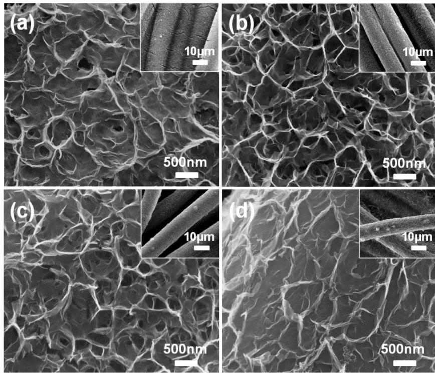
Figure S3. SEM images of (a) Mo-CoP<sub>3</sub>-1@CC, (b) Mo-CoP<sub>3</sub>-2@CC, (c) Mo-CoP<sub>3</sub>-3@CC, and (d) Mo-CoP<sub>3</sub>-4@CC.
