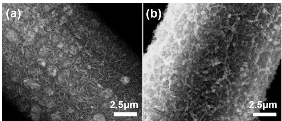
Figure S6. SEM images of the Mo-CoP<sub>3</sub>-2@CC: (a) after HER stability test; (b) after OER stability test.
