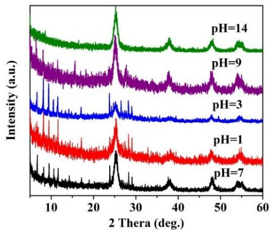
**Fig. S16.** PXRD patterns of 6.82%Ag/VPO@ $\text{TiO}_2$  composites after soaking for one day at pH = 1, 3, 9, 14 respectively.
