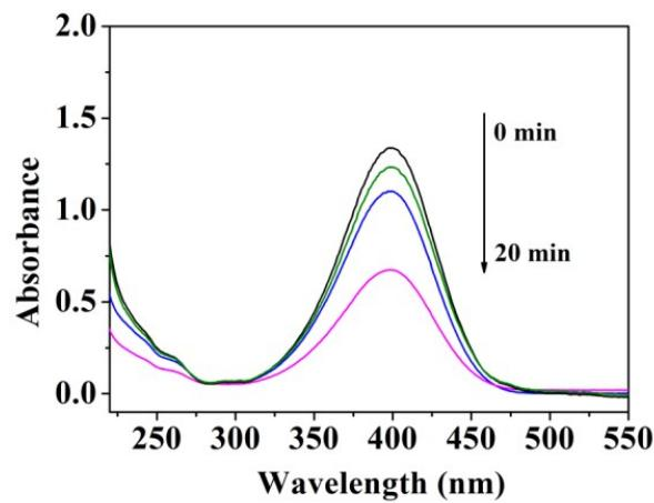
**Fig. S15.** UV-Vis absorption spectra of p-nitrophenol with  $\text{VPO}@\text{TiO}_2$  as catalyst.
