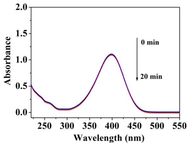
**Fig. S14.** UV-Vis absorption spectra of 4-NP with  $\text{TiO}_2$  as a catalyst.
