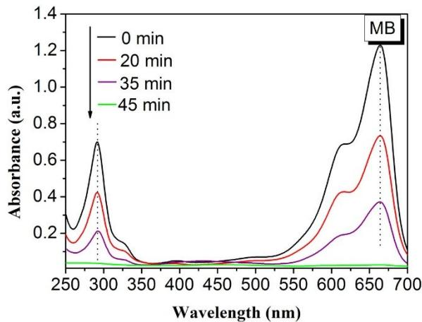
**Fig. S9.** Photocatalytic degradation profiles of MB for 6.82%Ag/VPO@TiO<sub>2</sub> composite under visible light irradiation.
