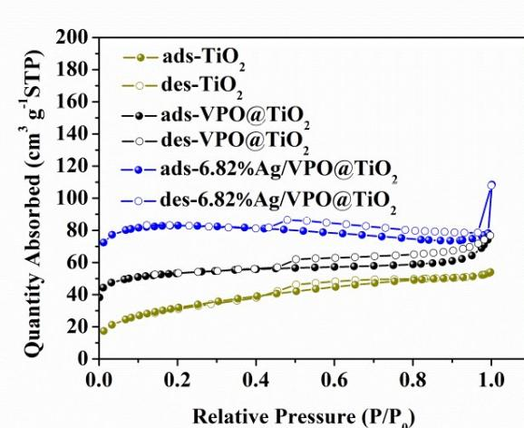
**Fig. S8.** N<sub>2</sub> adsorption-desorption isotherms of TiO<sub>2</sub>, VPO@TiO<sub>2</sub> and 6.82%Ag/VPO@TiO<sub>2</sub>, respectively.
