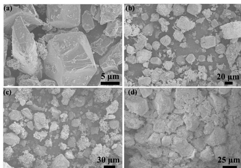
**Fig. S2.** SEM images of prepared VPO@TiO<sub>2</sub> composites at amount of (a) 60 μl TBT (b) 100 μl TBT (c) 200 μl TBT (d) 400 μl TBT.
