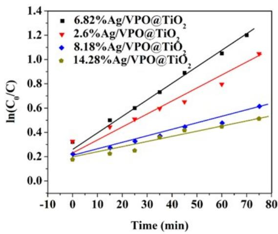
**Fig. S11** First-order kinetic plots for the photodegradation of MB by different samples.
