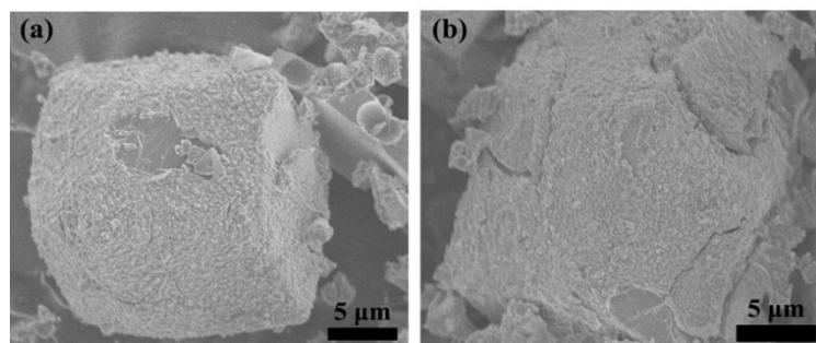
**Fig. S10.** (a) SEM images of 8.18%Ag/VPO@TiO<sub>2</sub>; (b) SEM images of 14.28%Ag/VPO@TiO<sub>2</sub>.
