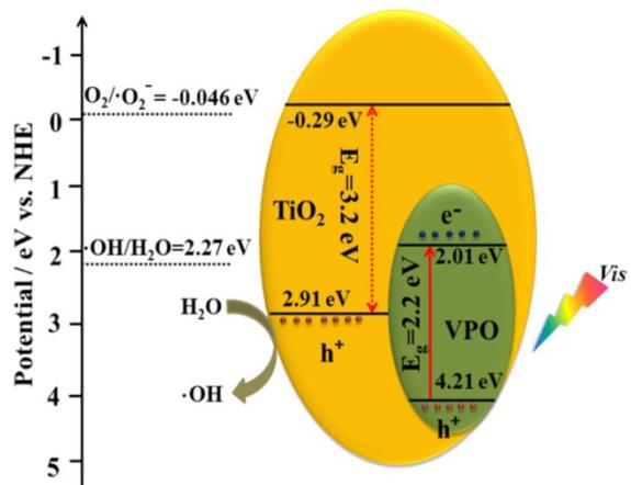
**Fig. S18.** The photodegraded mechanism of MB molecules by the VPO@TiO<sub>2</sub> composite under visible light irradiation.
