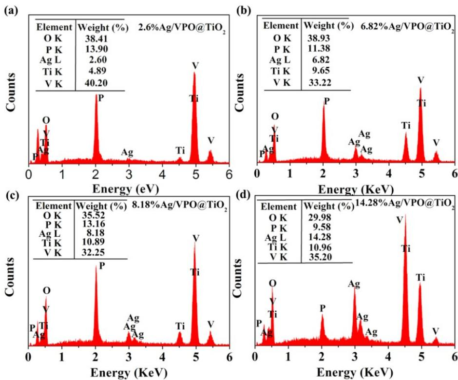
**Fig. S4.** EDX of (a) 2.6%Ag/VPO@TiO<sub>2</sub>; (b) 6.82%Ag/VPO@TiO<sub>2</sub>; (c) 8.18%Ag/VPO@TiO<sub>2</sub>; (d) 14.28%Ag/VPO@TiO<sub>2</sub>, respectively.
