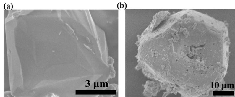
**Fig. S5.** (a) SEM images of pure VPO; (b) SEM images of Ag/VPO composite.
