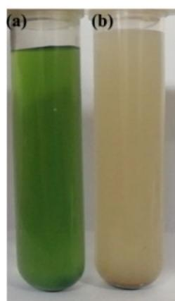
**Fig. S3.** The physical map of (a) single VPO water-soluble and (b) the prepared VPO@TiO<sub>2</sub> composite.
