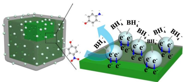
**Fig. S20.** Schematic illustration for the catalytic reduction of 4-NP molecules with the 6.82%Ag/VPO@TiO<sub>2</sub> composite.
