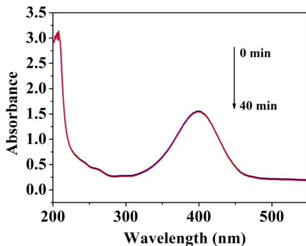
**Fig. S13.** UV-Vis absorption spectra of 4-NP with only the addition of NaBH<sub>4</sub> for 40 min.
