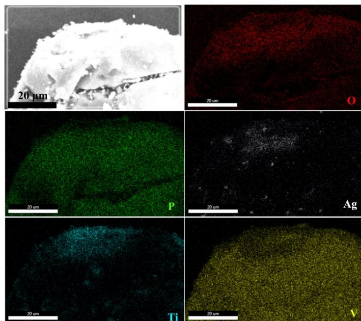
**Fig. S7.** Elemental mapping of 6.82%Ag/VPO@TiO<sub>2</sub>.
