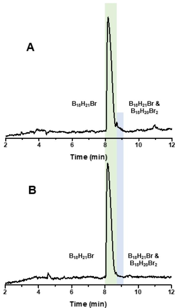
**Figure S6** A) LC trace of the material isolated from a single HPLC purification. B) LC trace of the material isolated after a second HPLC purification. The peak highlighted in green represents  $B_{18}H_{21}Br$ , and the peak highlighted in blue represents a mixture of  $B_{18}H_{21}Br$  and  $B_{18}H_{20}Br_2$ .
