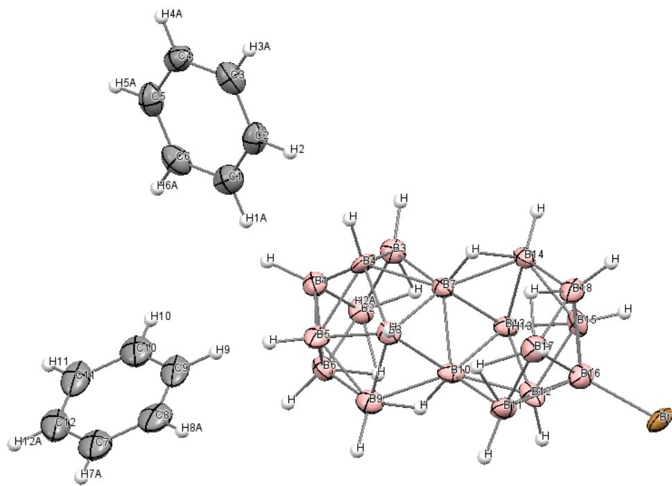
**Figure S7** 4-Br-*anti*-B<sub>18</sub>H<sub>21</sub> single crystal X-ray structure with two co-crystallized benzene solvent molecules.
