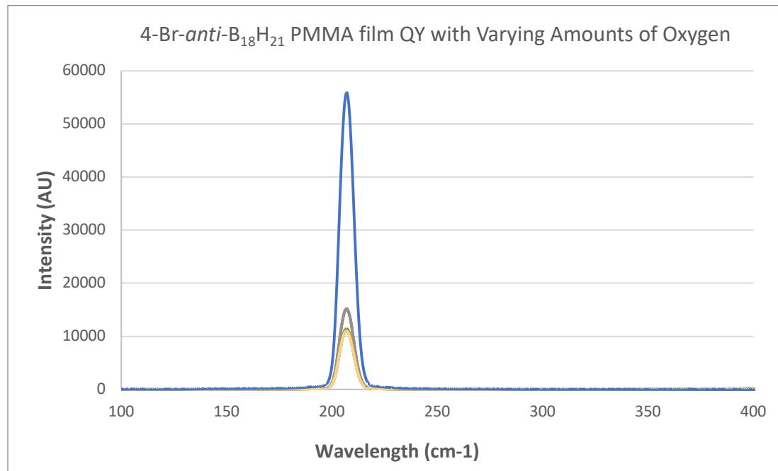
**Figure S8:** Quantum yield graph of a 4-Br-*anti*-B<sub>18</sub>H<sub>21</sub> containing PMMA film taken over time under increasing amounts of oxygen. The baseline from a quartz plate was first measured (blue), then the sample was measured under ambient conditions (gray). The system was placed under the flow of oxygen and measurements were taken over 35 min until the system reached an equilibrium (yellow).
