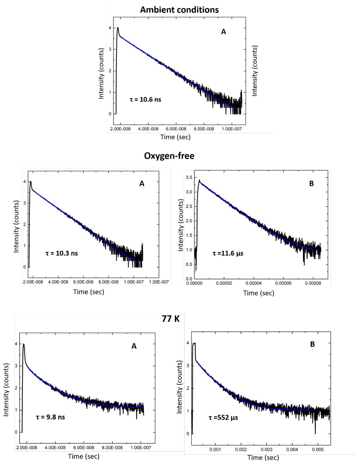
**Figure S11:** Luminescence decay curves (black) and fits (blue) for 4-Br-*anti*-B<sub>18</sub>H<sub>21</sub> in cyclohexane at 298 K under ambient conditions (top) at 298 K under oxygen-free conditions (middle) at 77 K (bottom). A) Observed at 410 nm, excitation at 331 nm. B) Observed at 525 nm, excitation at 372 nm.
