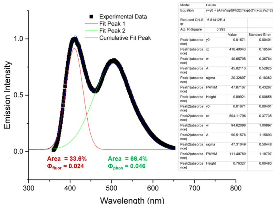
**Figure S10:** Deconvoluted emission spectrum of a cyclohexane solution of 4-Br-*anti*-B<sub>18</sub>H<sub>21</sub> under oxygen-free conditions. Peak percent as a function of area for each signal is listed, as well as the contribution to the overall quantum yield. QY contribution was calculated by multiplying peak percent by
