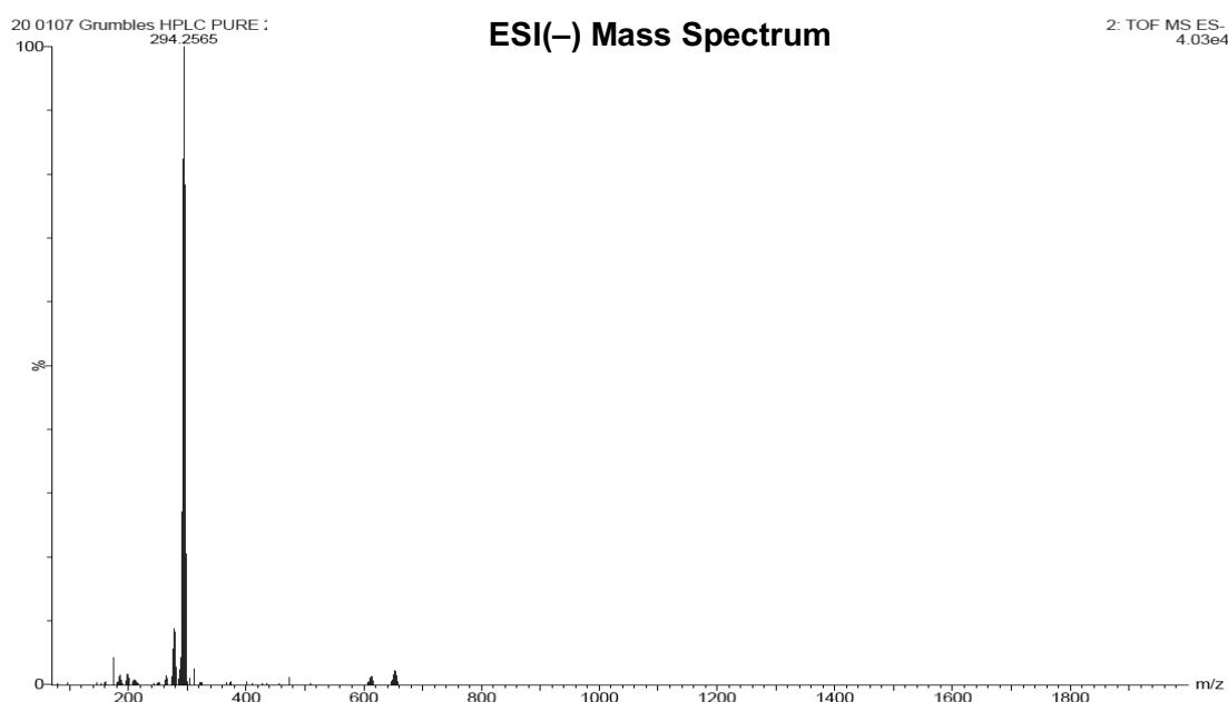
**Figure S1** ESI mass spectrum of 4-Br-*anti*-B<sub>18</sub>H<sub>21</sub> observed in negative mode.
