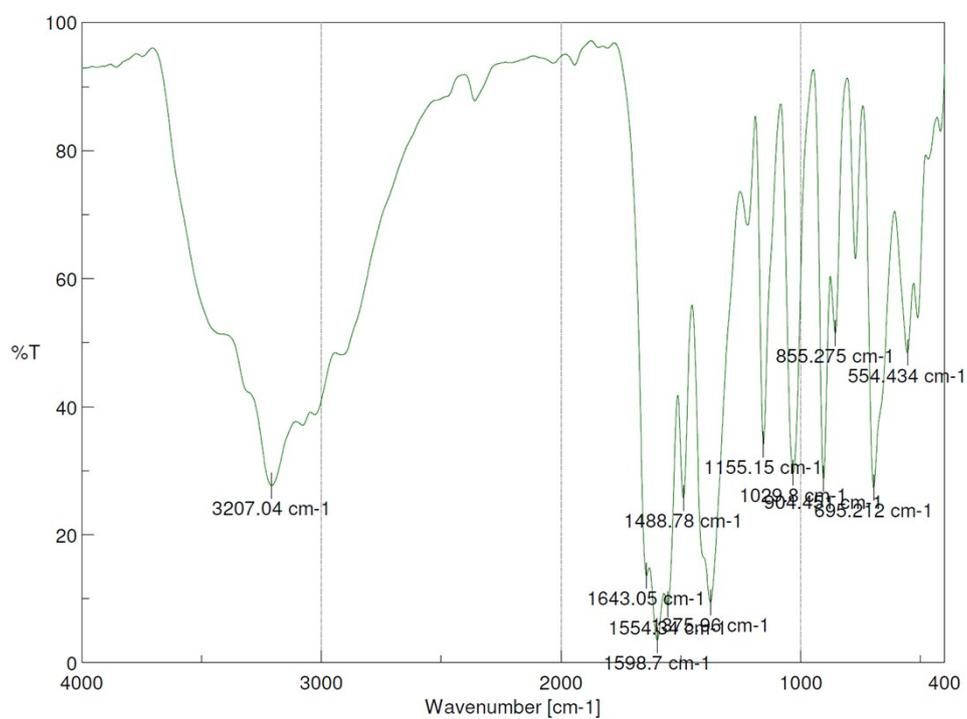
**Fig S5** FT-IR spectrum of MOF-1.
