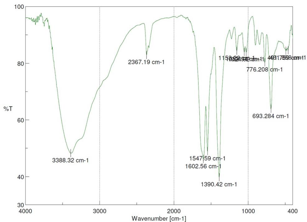
**Fig S6** FT-IR spectrum of MOF-2.
