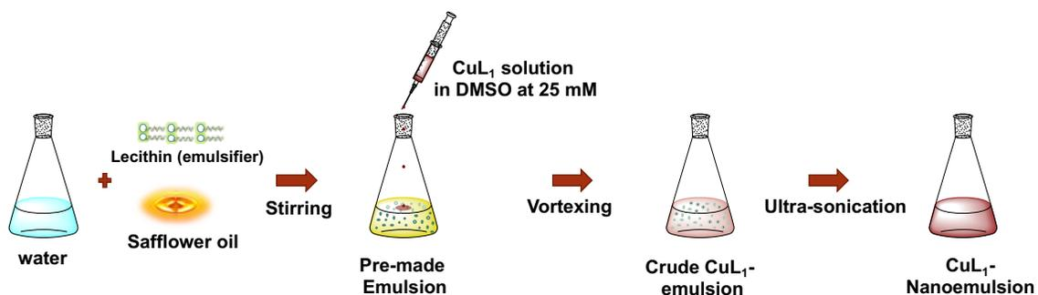
**Scheme S2.** Preparation of all nanoemulsions, using **CuL<sub>1</sub>** as an example.
