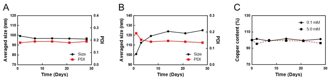
**Figure S4.** Stability of **NE CuL<sub>1</sub>** monitored over 4 weeks. (A, B) The change of size distribution of **NE CuL<sub>1</sub>** at (A) 0.1 mM and (B) 5.0 mM, assessed by dynamic light scattering. (C) The loss of copper content from **NE CuL<sub>1</sub>** determined by inductively coupled plasma optical emission spectroscopy.
