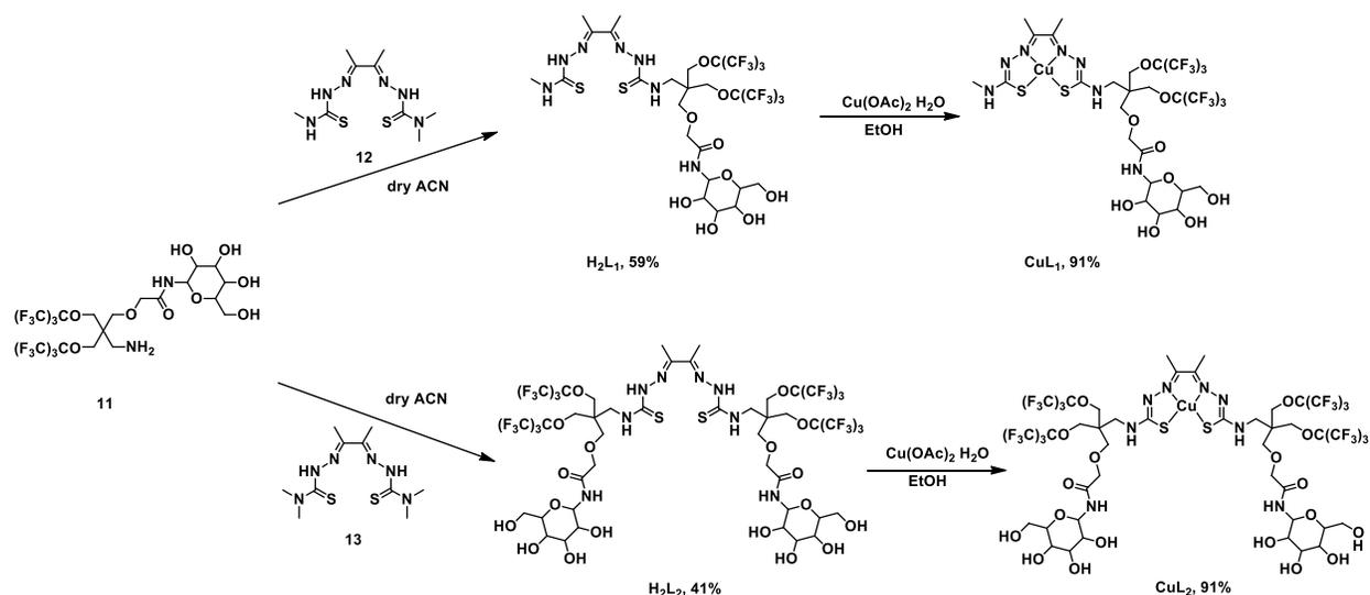
**Scheme S1.** Synthetic route for **H<sub>2</sub>L<sub>1</sub>**, **CuL<sub>1</sub>**, **H<sub>2</sub>L<sub>2</sub>**, and **CuL<sub>2</sub>**. Ligands **1** and **2**<sup>12</sup> and fluorinated tag **3**<sup>13</sup> were synthesized from previously reported literature.
