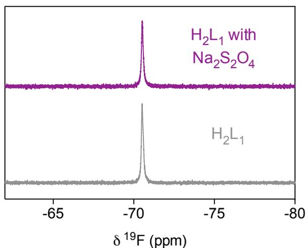
**Figure S6.** Control <sup>19</sup>F NMR of 1 mM **NE H<sub>2</sub>L<sub>1</sub>** with and without the addition of excess Na<sub>2</sub>S<sub>2</sub>O<sub>4</sub>.
