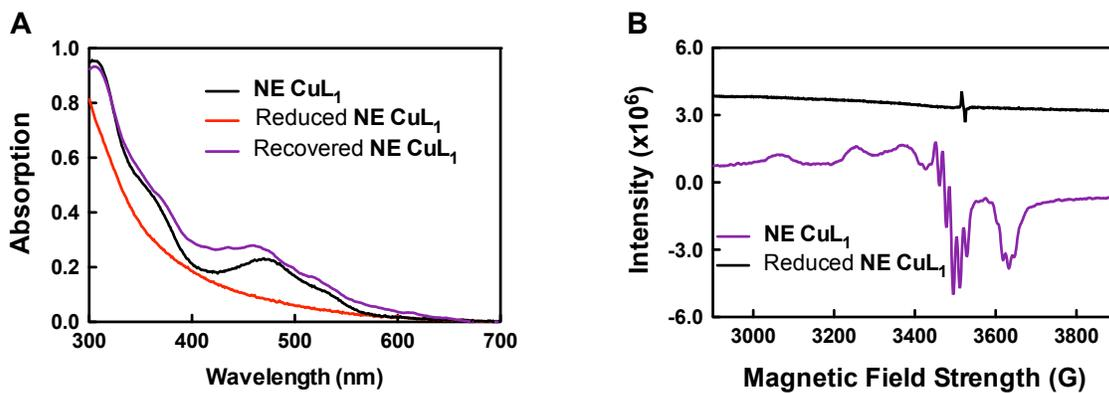
**Figure S7.** Reduction of **NE CuL<sub>1</sub>** and reformation of **NE CuL<sub>1</sub>** illustrated by (A) UV-vis absorption and (B) EPR spectroscopy.
