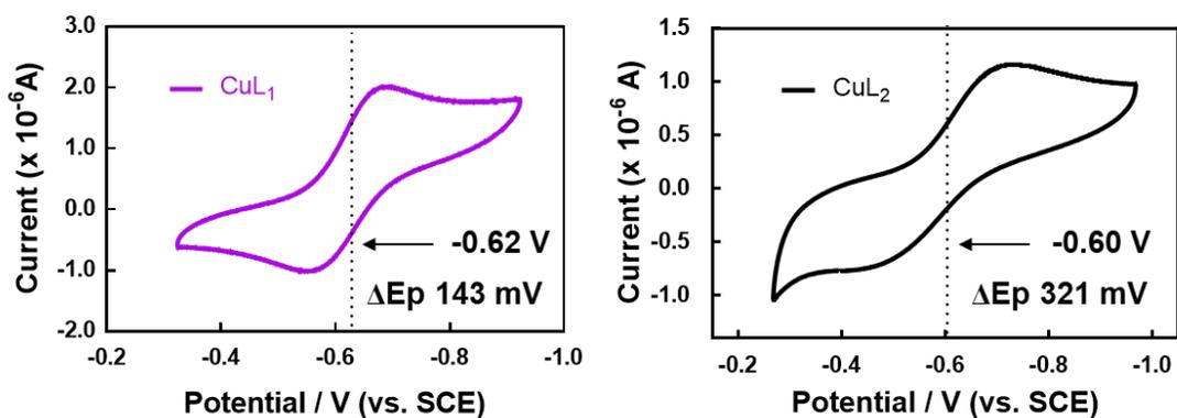
**Figure S3.** Cyclic voltammograms of  $\text{CuL}_1$  and  $\text{CuL}_2$  (vs. SCE in DMF).
