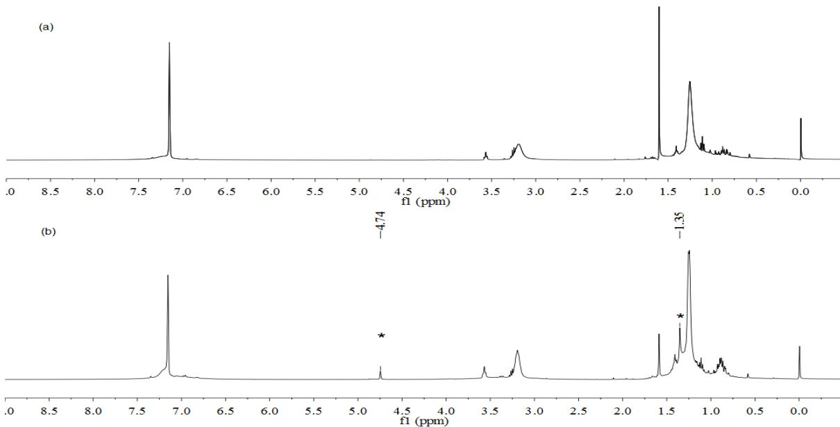
**Figure S13.** (a)  $^1\text{H}$  NMR spectrum of **1** and 2-Iodo-2-methylpropane in  $\text{C}_6\text{D}_6$ ; (b) After heating the NMR tube at  $80^\circ\text{C}$  for 4 hours. \*Indicating the formation of isobutene.
