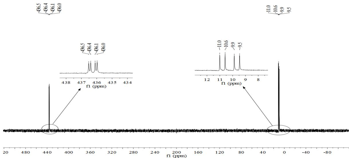
**Figure S38.**  $^{31}\text{P}$  NMR spectrum of **10** in  $\text{CD}_2\text{Cl}_2$ .
