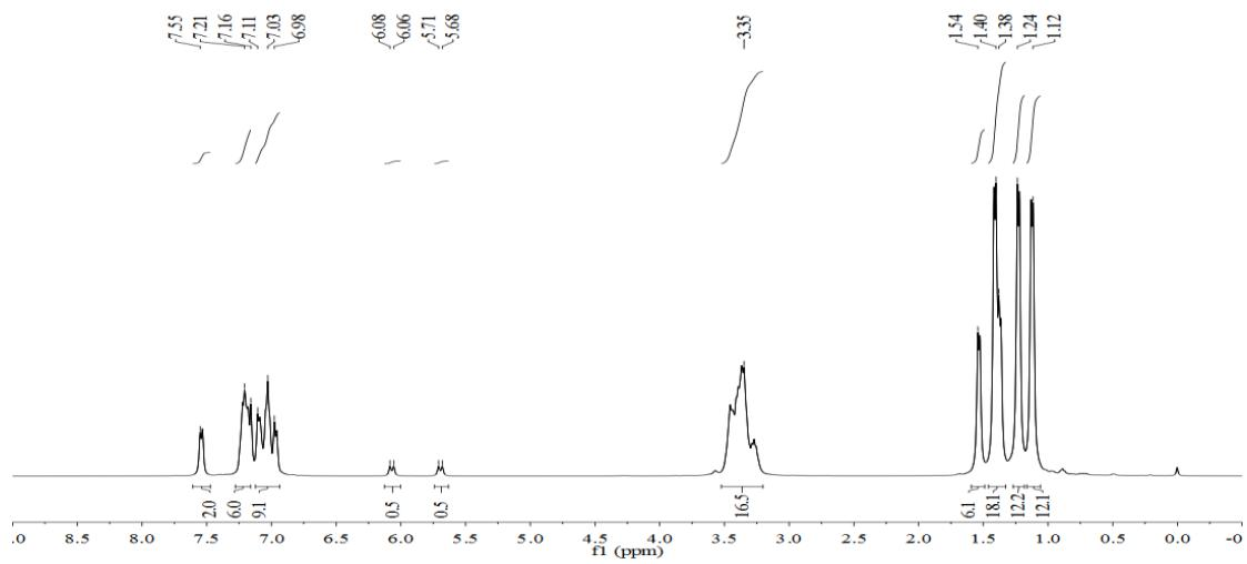
**Figure S1.**  $^1\text{H}$  NMR spectrum of **2** in  $\text{C}_6\text{D}_6$ .
