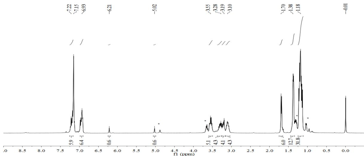
**Figure S24.** <sup>1</sup>H NMR spectrum of **9** in C<sub>6</sub>D<sub>6</sub>. \*Small amount of impurity.
