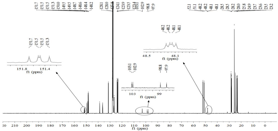
**Figure S2.**  $^{13}\text{C}\{^1\text{H}\}$  NMR spectrum of **2** in  $\text{C}_6\text{D}_6$ .
