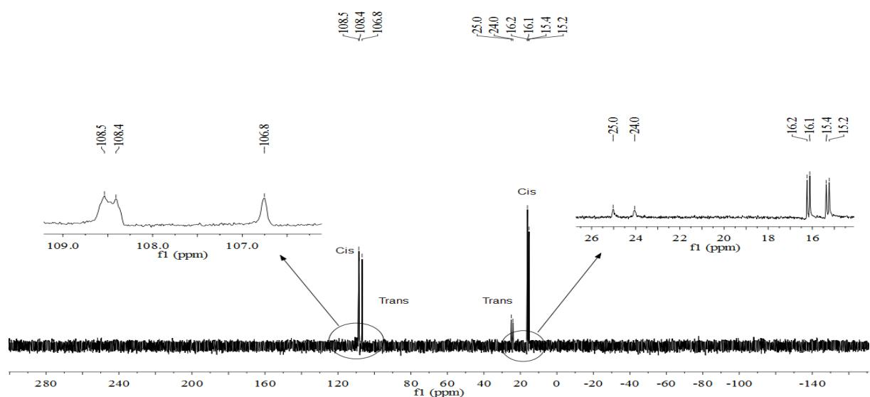
**Figure S19.**  $^{31}\text{P}$  NMR spectrum of **6** in  $\text{C}_6\text{D}_6$ .
