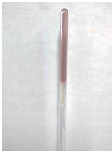
Figure S15. Solution of 2c in THF in an inverted NMR tube showing gel formation by catalytic ring-opening polymerization of the solvent.
