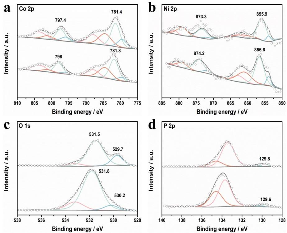
**Figure S3.** XPS high-resolution spectra of (a) Co 2p, (b) Ni 2p, (c) O 1s and (d) P 2p for multi-shelled  $\text{Co}_{0.9}\text{Ni}_{0.1}$  oxide/phosphide (upper), and multi-shelled  $\text{Co}_{0.5}\text{Ni}_{0.5}$  oxide/phosphide (bottom).
