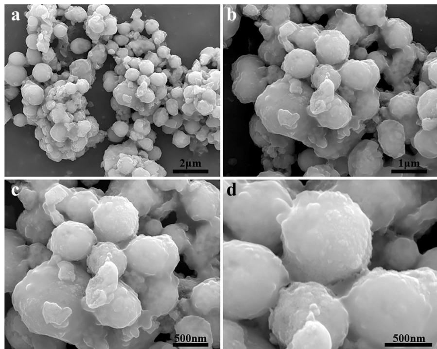
**Figure S7.** FESEM images of multi-shelled  $\text{Co}_{0.5}\text{Ni}_{0.5}$  oxide/phosphide after OER test under different magnifications.
