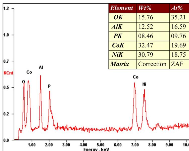
**Figure S1.** The energy dispersive X-ray spectrum for the multi-shelled Co<sub>0.5</sub>Ni<sub>0.5</sub> oxide/phosphide. The signal of Al in the EDX spectrum was derived from the conductive aluminum foil substrate used for the FESEM measurement.
