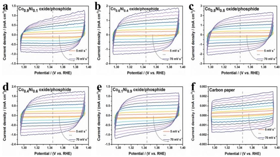
**Figure S4.** Cyclic voltammetry (CV) curves for (a)  $\text{Co}_{0.9}\text{Ni}_{0.1}$  oxide/phosphide, (b)  $\text{Co}_{0.6}\text{Ni}_{0.4}$  oxide/phosphide, (c)  $\text{Co}_{0.5}\text{Ni}_{0.5}$  oxide/phosphide, (d)  $\text{Co}_{0.4}\text{Ni}_{0.6}$  oxide/phosphide, (e)  $\text{Co}_{0.1}\text{Ni}_{0.9}$  oxide/phosphide and (f) bare carbon paper at incremental scan rates in the potential range of 1.3 - 1.4 V vs RHE.
