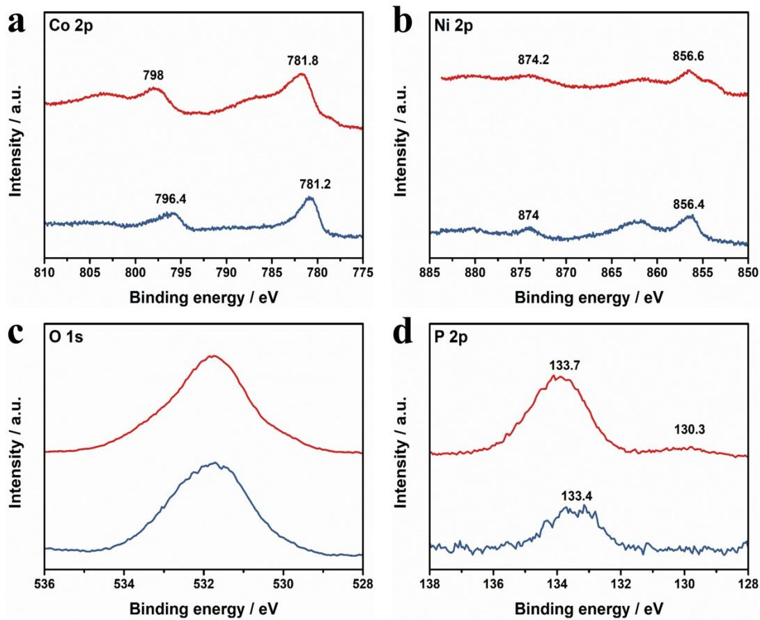
**Figure S8.** XPS high-resolution spectra of (a) Co 2p, (b) Ni 2p, (c) O 1s and (d) P 2p for multi-shelled  $\text{Co}_{0.5}\text{Ni}_{0.5}$  oxide/phosphide before (upper) and after (bottom) OER test.
