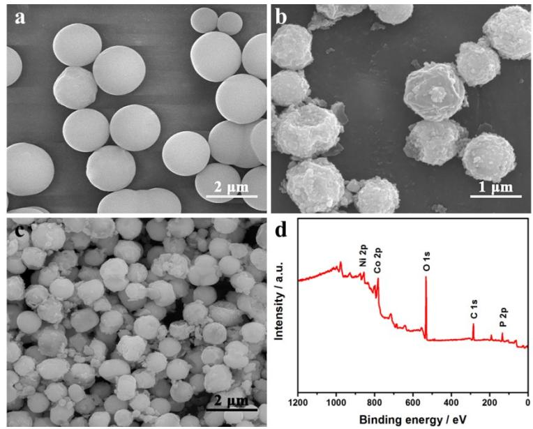
**Figure S2.** FESEM images of (a)  $\text{Co}_{0.5}\text{Ni}_{0.5}$  CPS, (b) multi-shelled  $\text{Co}_{0.5}\text{Ni}_{0.5}$  oxide and (c) multi-shelled  $\text{Co}_{0.5}\text{Ni}_{0.5}$  oxide/phosphide. (d) XPS spectrum of elements surveys for multi-shelled  $\text{Co}_{0.5}\text{Ni}_{0.5}$  oxide/phosphide.
