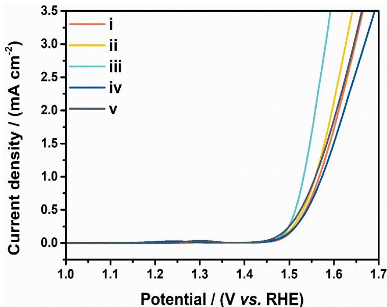
**Figure S5.** Polarization curves after being normalized by ECSA for multi-shelled  $\text{Co}_x\text{Ni}_{1-x}$  oxide/phosphide electrocatalysts. (i)  $\text{Co}_{0.9}\text{Ni}_{0.1}$  oxide/phosphide, (ii)  $\text{Co}_{0.6}\text{Ni}_{0.4}$  oxide/phosphide, (iii)  $\text{Co}_{0.5}\text{Ni}_{0.5}$  oxide/phosphide, (iv)  $\text{Co}_{0.4}\text{Ni}_{0.6}$  oxide/phosphide and (v)  $\text{Co}_{0.1}\text{Ni}_{0.9}$  oxide/phosphide.
