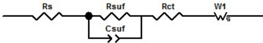
Fig. S3 Equivalent circuit of battery contained \text{Co}_{3-x}\text{Mn}_x\text{O}_4/\text{C}/\text{S} electrodes at 5 C.
