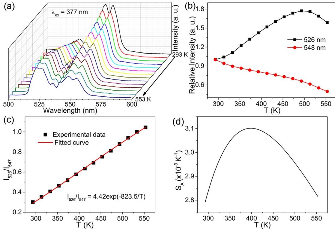
Fig. S4 (a) Emission spectra of GSO:10%Yb<sup>3+</sup>, 1%Er<sup>3+</sup> excited at 377 nm under various temperatures; (b) relative intensities of 526 and 548 nm emissions of Er<sup>3+</sup> as a function of temperature; (c) dependences of  $I_{526}/I_{548}$  on absolute temperature; (d) absolute and relative sensitivities of GSO:10%Yb<sup>3+</sup>, 1%Er<sup>3+</sup> as a function of absolute temperature
