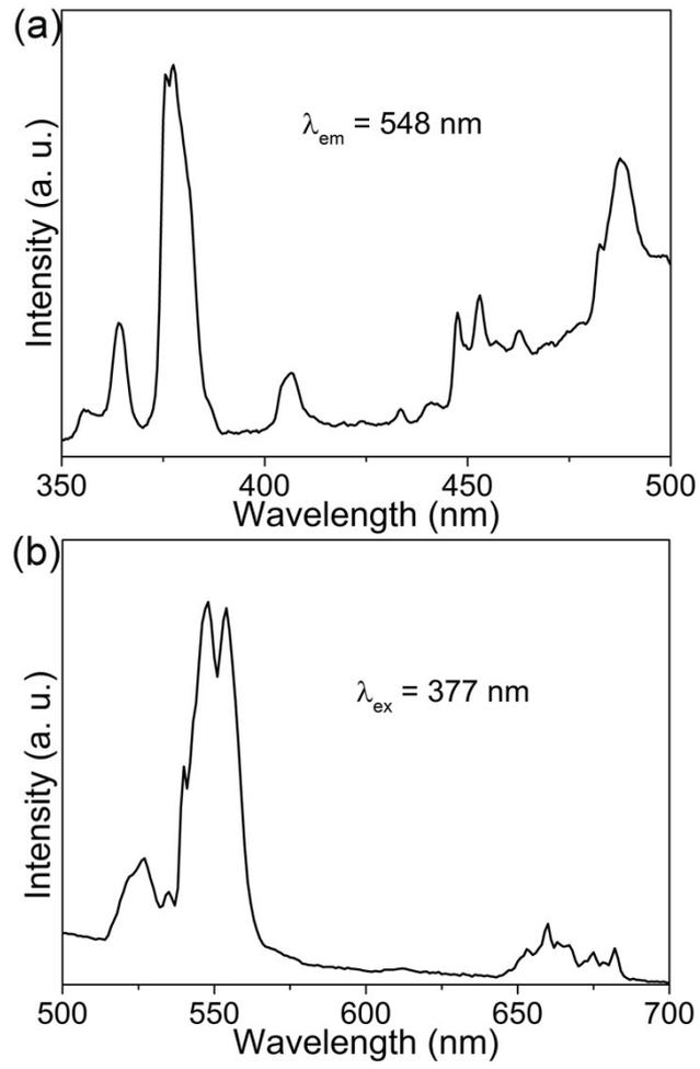
Fig. S3 (a) Excitation and (b) emission spectra of GSO:10%Yb<sup>3+</sup>,1%Er<sup>3+</sup>
