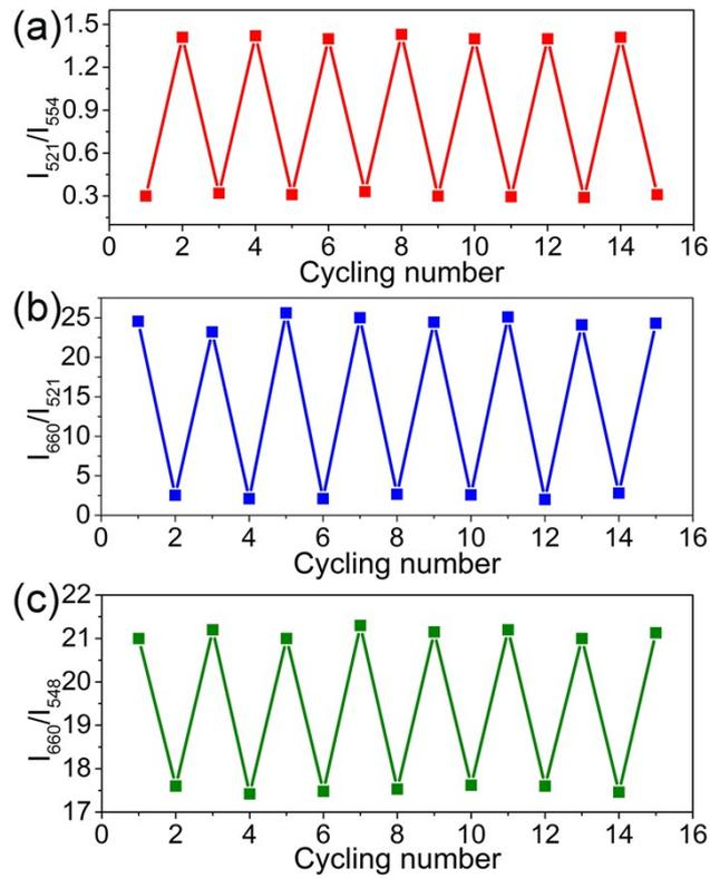
Fig. S2 Temperature-induced switching of (a)  $I_{521}/I_{554}$  and (b)  $I_{660}/I_{521}$  for GSO:10%Yb<sup>3+</sup>,1%Er<sup>3+</sup> as well as (c)  $I_{660}/I_{548}$  for GSO:10%Yb<sup>3+</sup>,0.25%Ho<sup>3+</sup>
