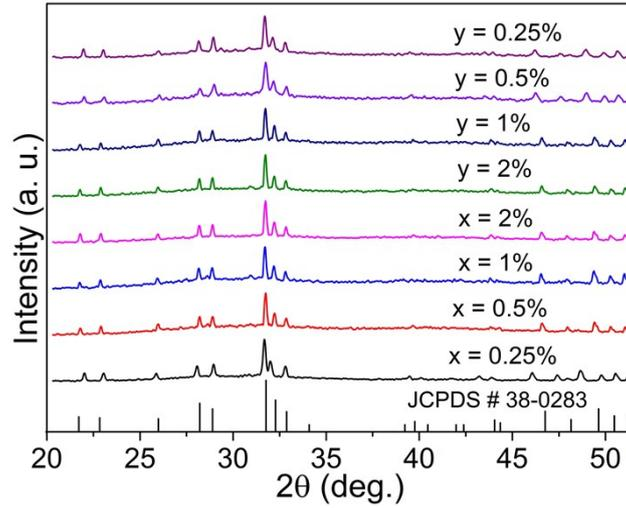
Fig. S1 XRD patterns of GSO:10%Yb<sup>3+</sup>,xEr<sup>3+</sup> (0.25% ≤ x ≤ 2%) and
