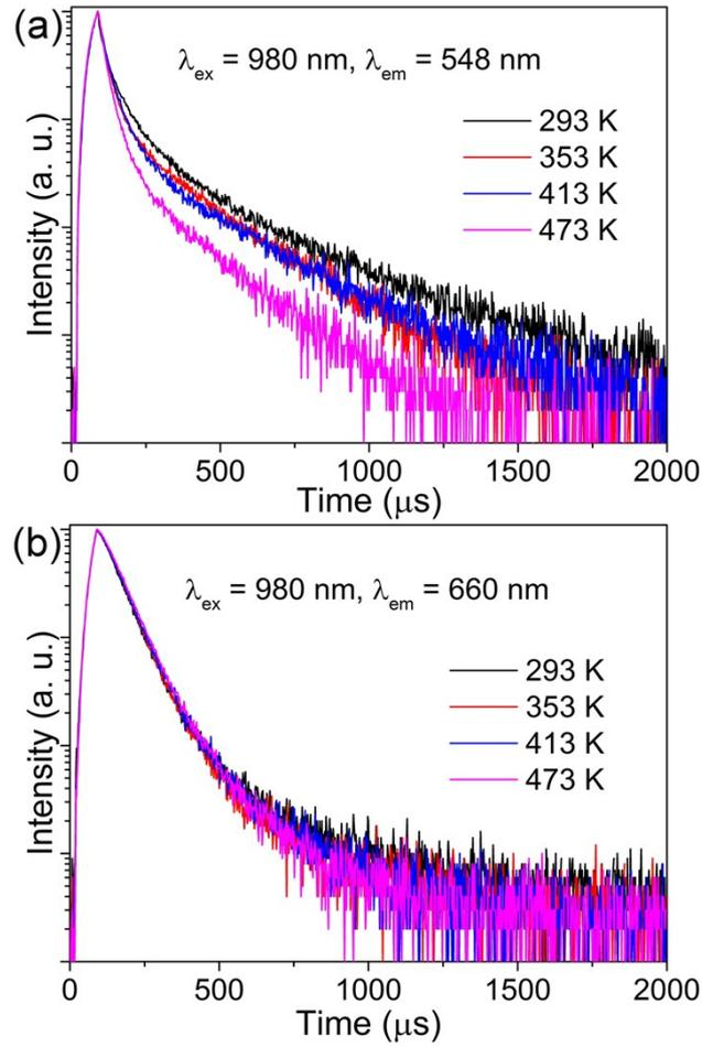
Fig. S5 Decay curves of GSO:10%Yb<sup>3+</sup>,0.25%Ho<sup>3+</sup> under different temperatures by monitoring (a) 548 nm and (b) 660 nm
