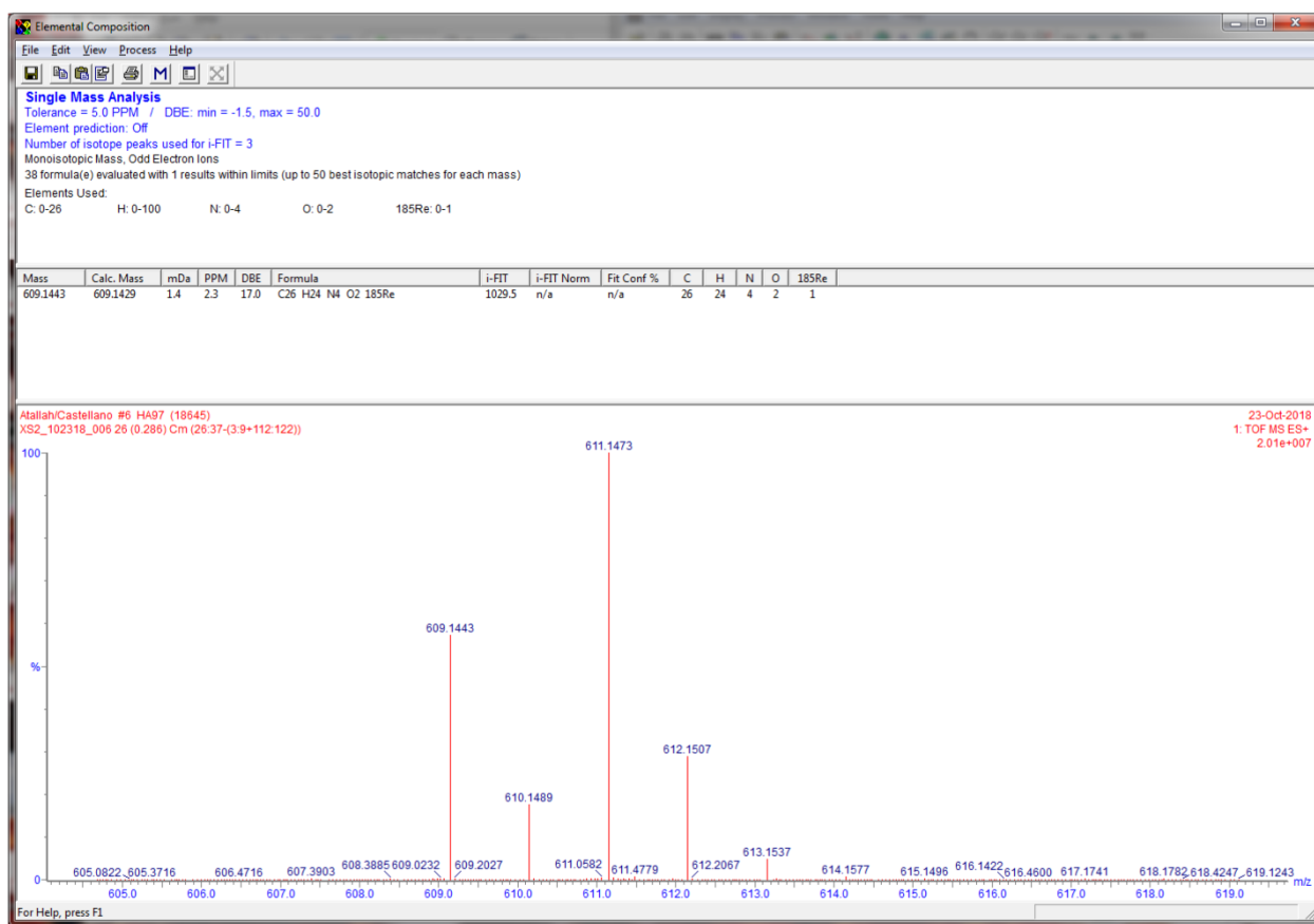
Figure S21. HRMS spectrum of cis -[Re(4,4'-Me 2 bpy) 2 (CO) 2 ]PF 6 ( 9 ).
