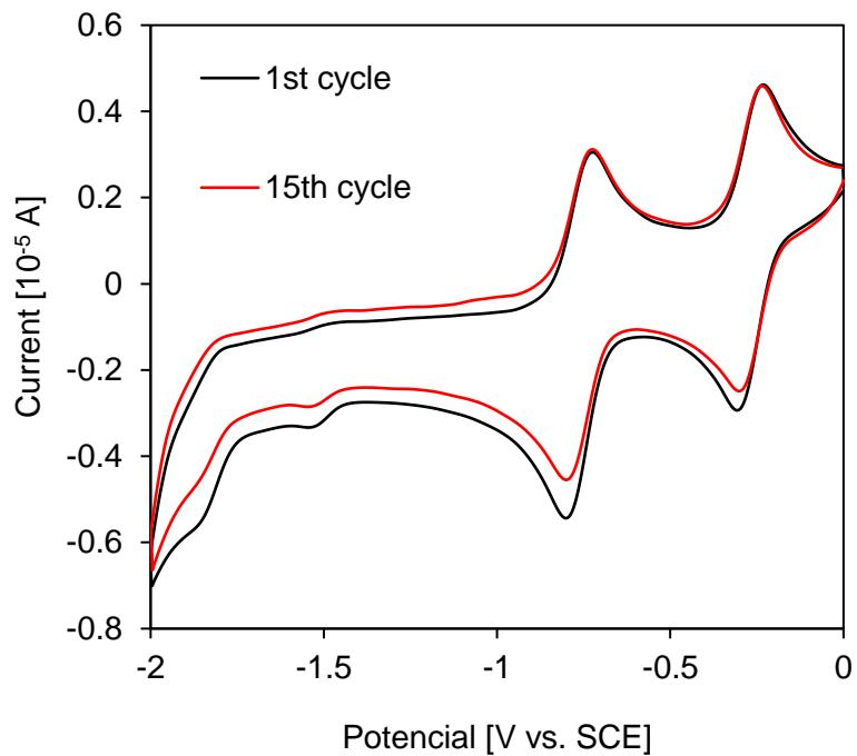
**Fig. S2** CV of **1** (1 mM) in 0.1 M  $\text{Bu}_4\text{NClO}_4$ /DMF using a GC working electrode at a scan rate of 10 mV/sec.
