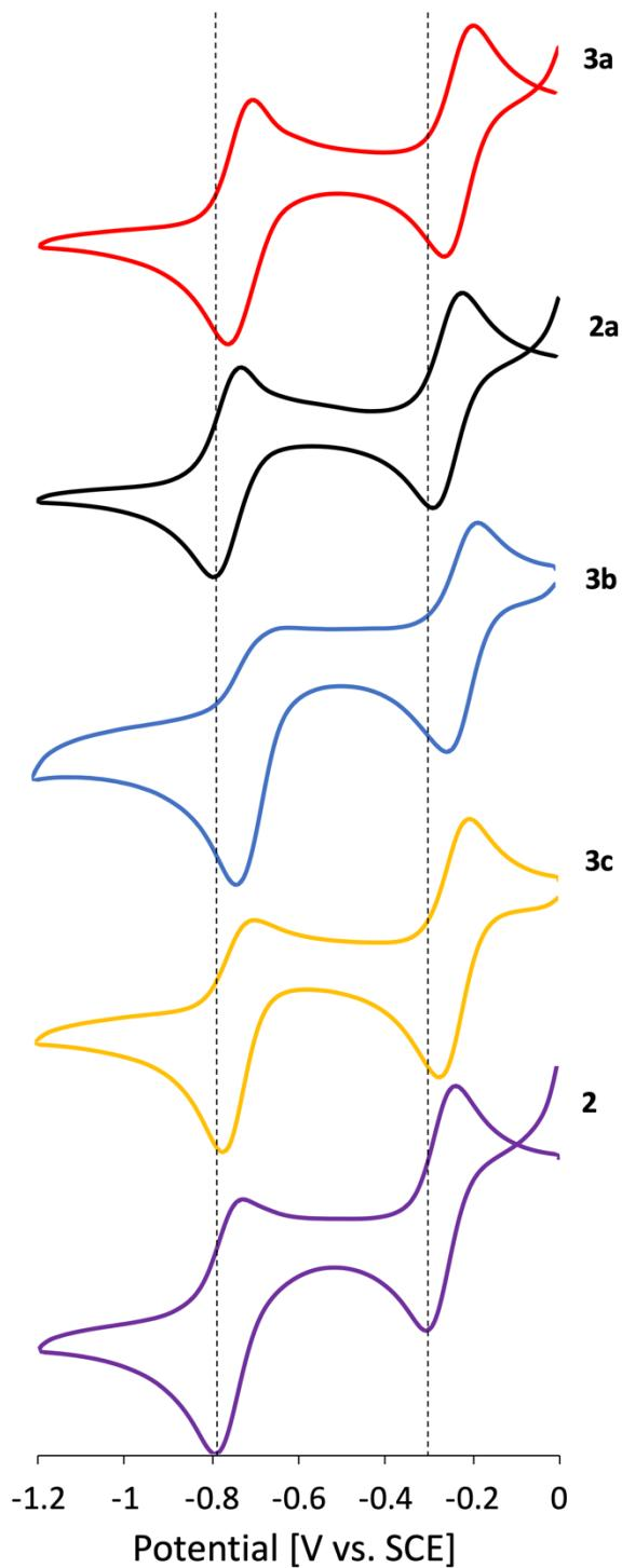
**Fig. S3** CVs of **1**, **2a**, **3a-c** (1 mM) in 0.1 M  $\text{Bu}_4\text{NClO}_4$ /DMF using a GC working electrode at a scan rate of 10 mV/sec.
