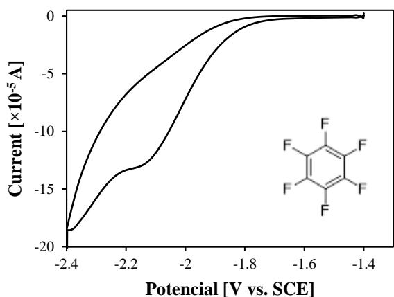
**Fig. S1** CV of hexafluorobenzene (10 mM) in 0.1 M  $\text{Bu}_4\text{NClO}_4$ /DMF using a GC working electrode at a scan rate of 100 mV/s.
