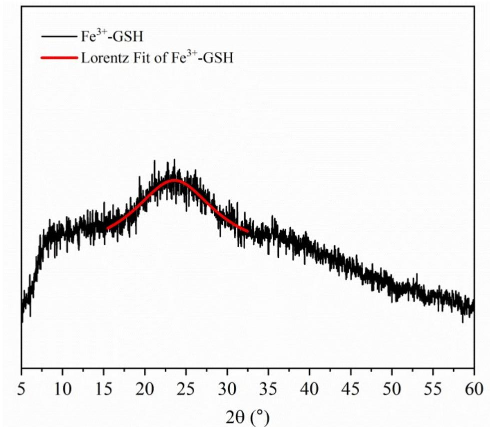
**Figure S7** X-ray powder diffraction spectrum of Fe<sup>3+</sup>-GSH.
