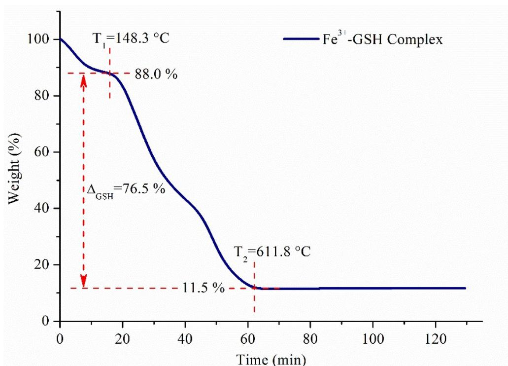
**Figure S10** TGA thermogram corresponding to the Fe<sup>3+</sup>-GSH complex.
