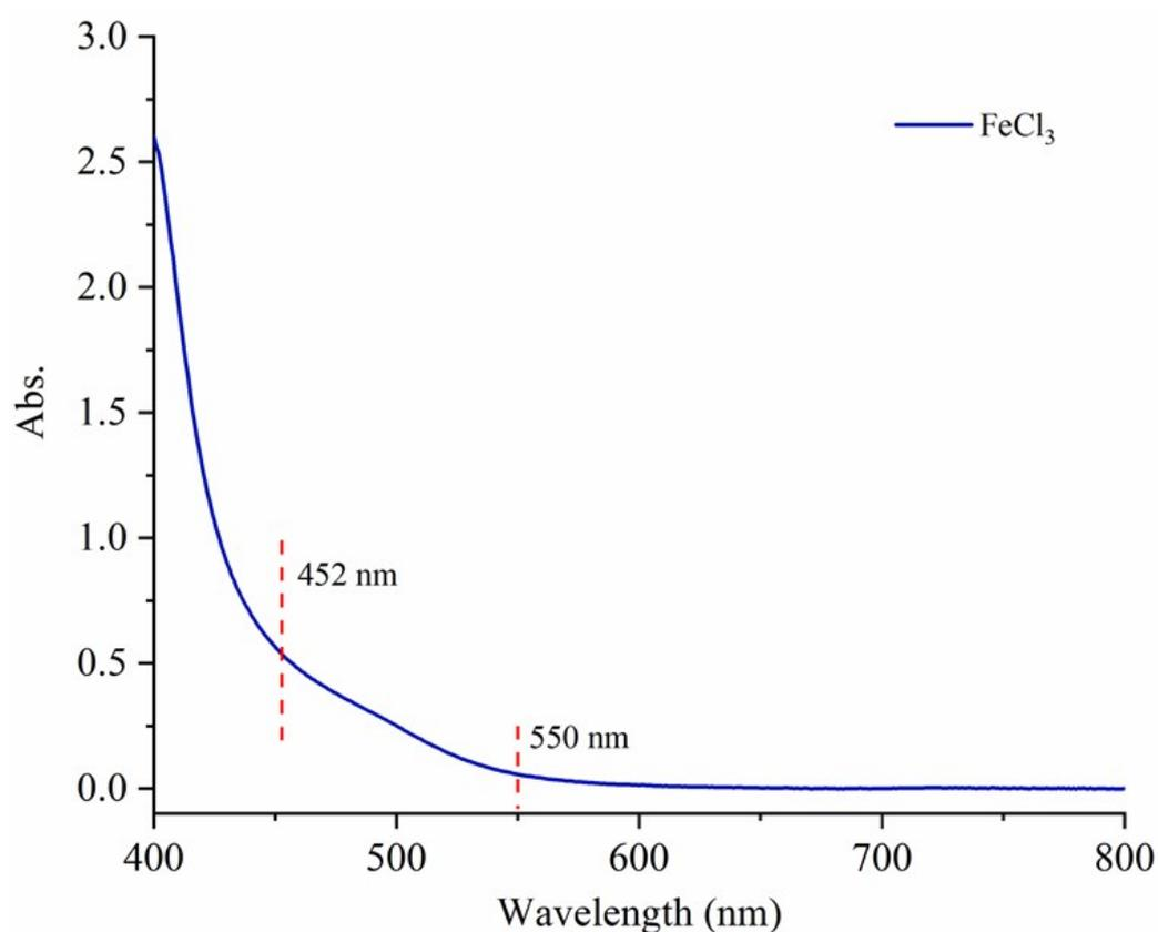
**Figure S2.** UV-Vis adsorption spectrum of a 40 mM FeCl<sub>3</sub> aqueous solution depicting absorption peaks at 452 nm and 550 nm.
