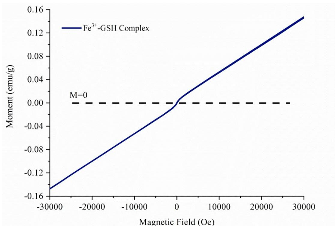
**Figure S12** Vibrating-sample magnetometer measurement of  $\text{Fe}^{3+}$ -GSH from -3 T to 3 T magnetic field at room temperature.
