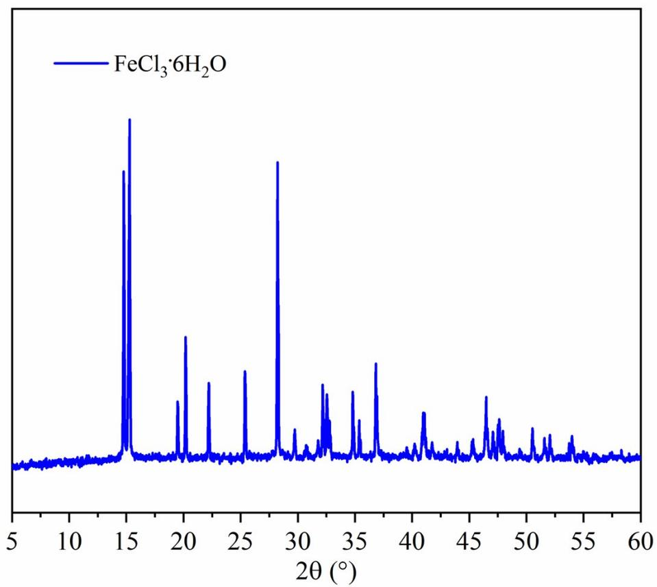
**Figure S8** X-ray powder diffraction of Iron(III) chloride hexahydrate (FeCl<sub>3</sub>·6H<sub>2</sub>O)
