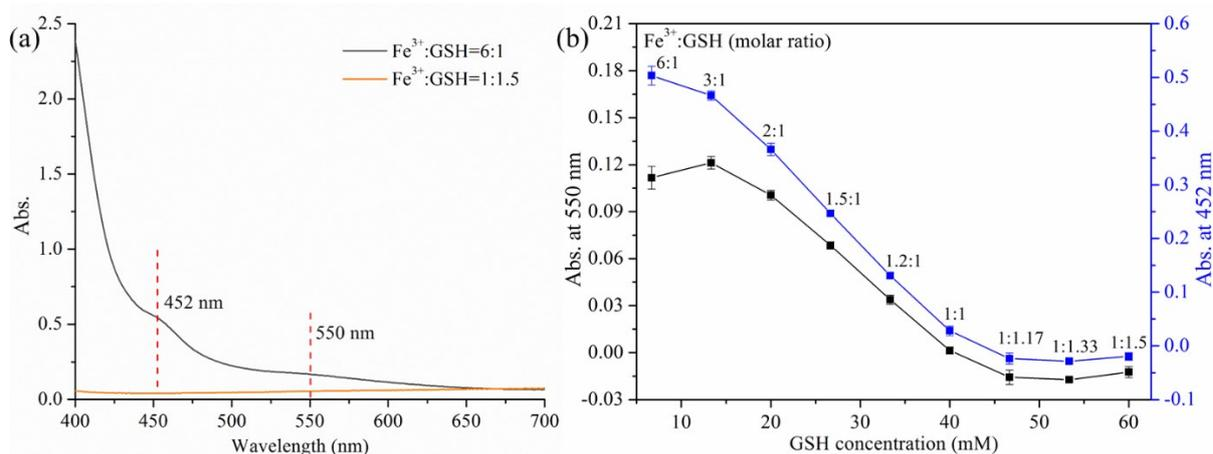
**Figure S1** UV-Vis absorption spectroscopy of Fe<sup>3+</sup>-GSH complex solution formed in H<sub>2</sub>O with 40 mM FeCl<sub>3</sub>. (A): Full wavelength spectrum of solutions containing an FeCl<sub>3</sub>:GSH molar ratio of either 6:1 (black) or 1:1.5 (orange). (B): Tracking of 452 nm (right-handed y-axis) and 550 nm (left-handed y-axis) absorbances recorded in solutions with an FeCl<sub>3</sub>:GSH molar ratio in the range of 6:1–1:1.15.
