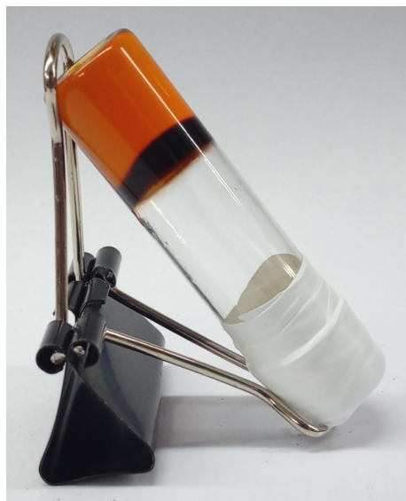
Fig. S15 Reduction of Fe(III) to Fe(II) of metallogel by ascorbic acid.
