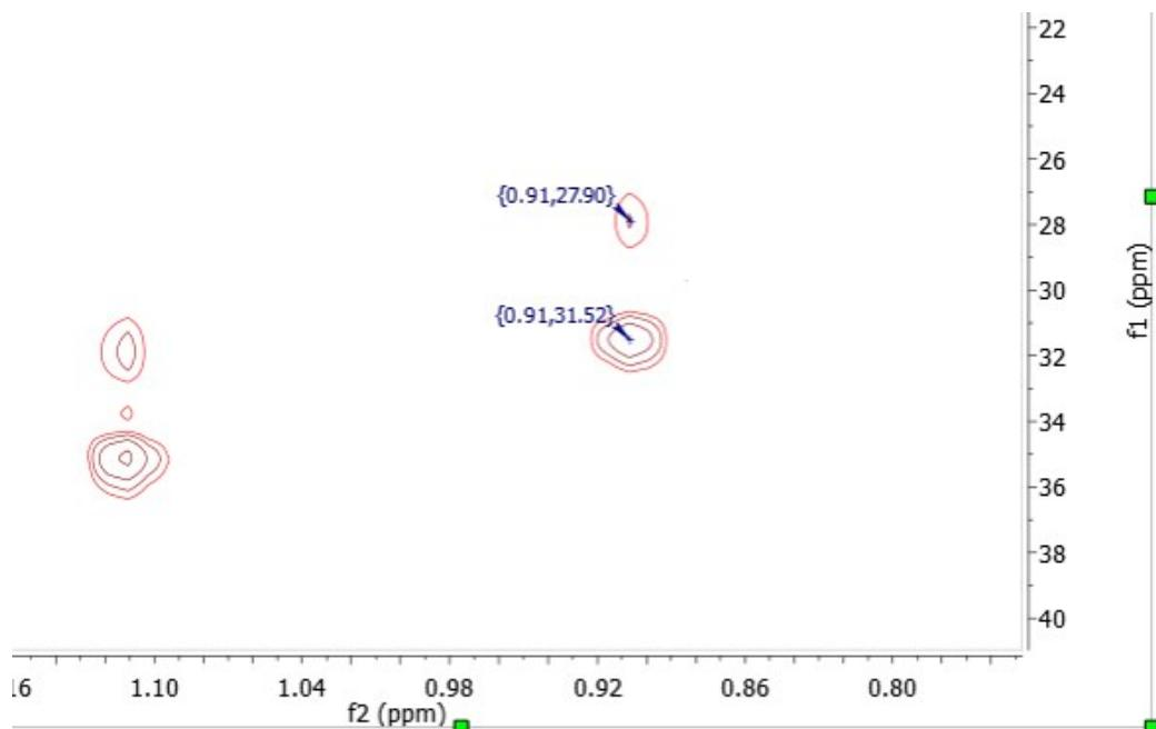
Figure 6: HMBC $\{{}^1\text{H}, {}^{13}\text{C}\}$ (500 MHz) spectrum of the reaction AlNp<sub>3</sub> with C<sub>14</sub>H<sub>8</sub>(N(*m*-Xy))<sub>2</sub>, neo-pentane is found with cross peaks at (0.91, 27.9 ( $(\text{H}_3\text{C})_3\text{-C-CH}_3$ ))) and (0.91, 31.5( $(\text{H}_3\text{C})_3\text{-C-CH}_3$ ))), which is the consistent as described in the literature.<sup>2</sup>
