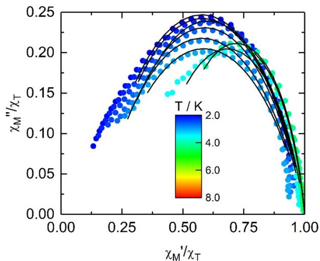
**Figure S10.** Normalized Cole-Cole plot at several temperatures between 2 and 4.5 K for **1<sub>10</sub>**.
