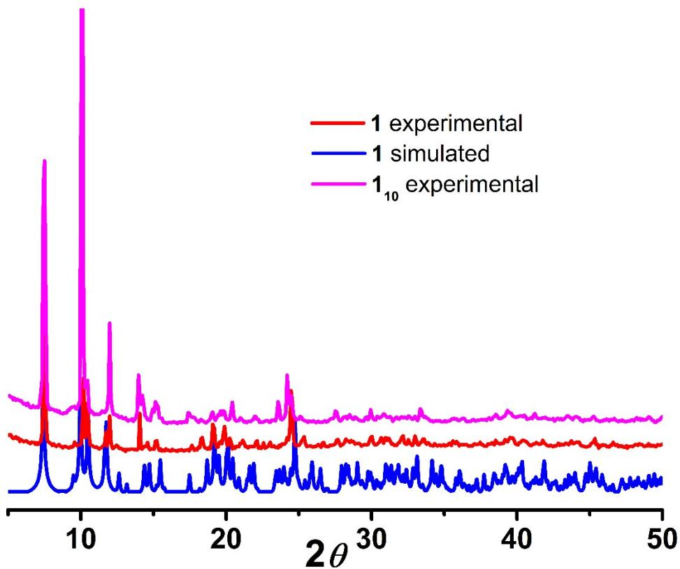
**Figure S1.** Simulated and experimental XRD pattern for **1** along with experimental pattern of **1<sub>10</sub>**.
