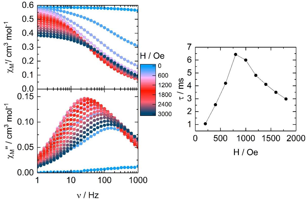
**Figure S5.** (Left) In-phase and out-of-phase components of the ac magnetic susceptibility for **1<sub>10</sub>** at 2 K under a DC magnetic field from 0 to 3000 Oe. (Right) Representation of the field-dependence of the relaxation time of the magnetization at 2 K, the maximal  $\tau$  corresponding to 800 Oe.
