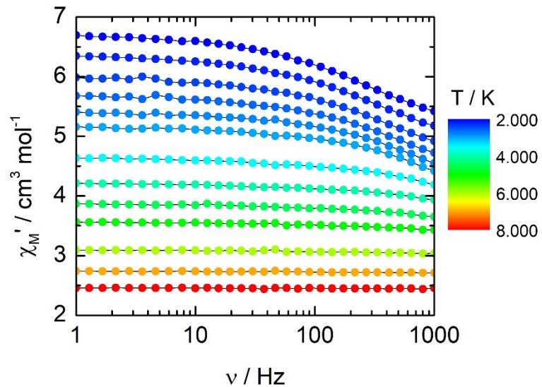
**Figure S6.** In-phase component of the ac magnetic susceptibility data for **1**, from 2 to 8 K under 1200 Oe.
