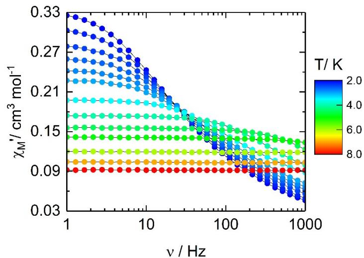
**Figure S7.** In-phase component of the ac magnetic susceptibility data for **1<sub>10</sub>**, from 2 to 8 K under 800 Oe.
