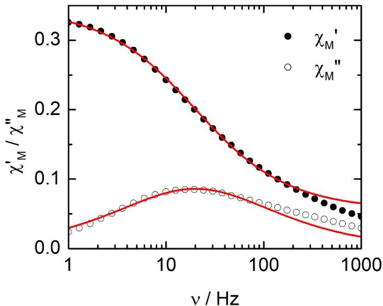
**Figure S8.** Frequency dependence of the in-phase ( $\chi_M'$ ) and out-of-phase ( $\chi_M''$ ) components of the ac susceptibility measured on powder at 2 K and 800 Oe with the best fitted curves (red lines) for  $\mathbf{1}_{10}$ .
