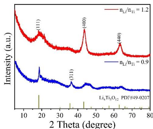
Fig. S1 XRD patterns of titanium oxides with different molar ratios of Li/Ti obtained by acid
