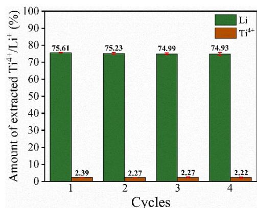
**Fig. S5** The amount of extracted lithium and the dissolution of titanium in recycle process.
