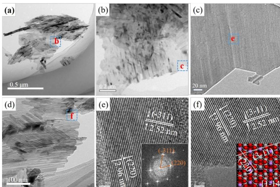
**Fig. S2** (a)(b)(c)(d) TEM images of  $\text{Li}_4\text{Ti}_5\text{O}_{12}$  (e) and (f) high-resolution TEM images of  $\text{Li}_4\text{Ti}_5\text{O}_{12}$ . The inset images of (e) is FFT and the inset of (f) is  $\text{Li}_4\text{Ti}_5\text{O}_{12}$  (1-14) facet.
