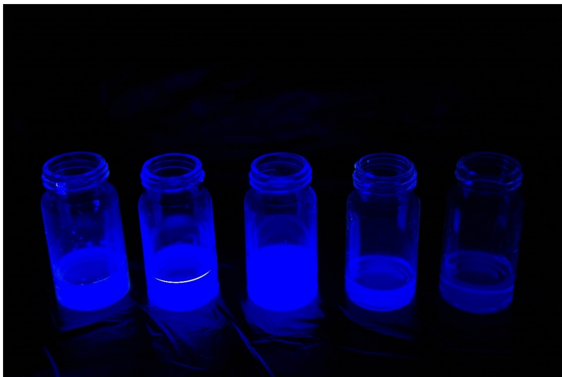
Figure S4. Fluorescence of NMA in DMSO solution of different concentrations under 365 nm UV irradiation. The concentration from left to right: saturated, 10^{-3} M, 10^{-4} M, 10^{-5} M, 10^{-6} M.
