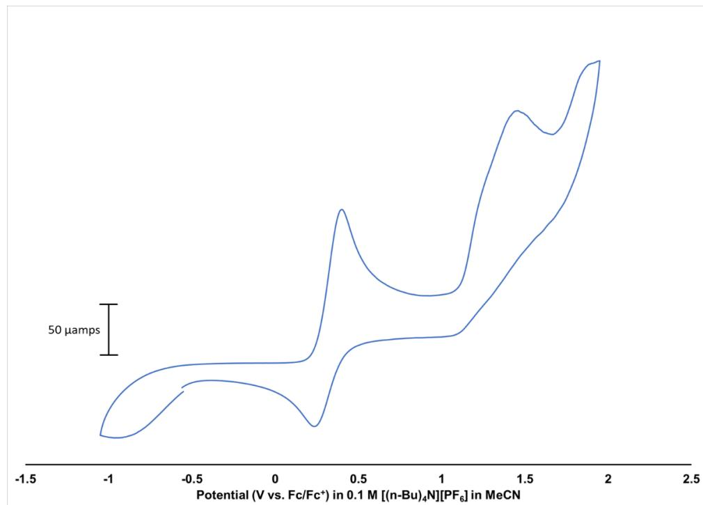
**Figure S2.** CV trace of complex **6** at 500 mV/s showing coalescence of the two unknown oxidation events.
