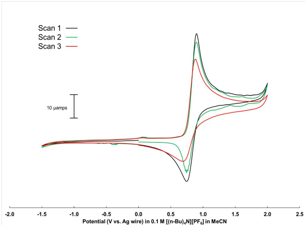
**Figure S3.** CV traces showing diminished reversibility of the Rh oxidation over multiple scans for complex **4** in MeCN.
