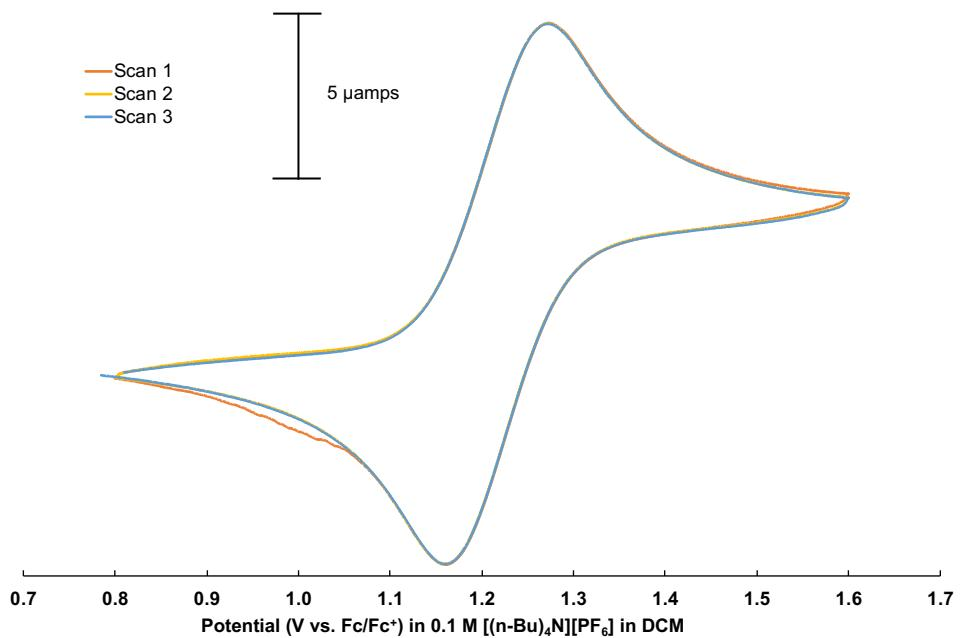
**Figure S4.** CV traces showing diminished reversibility of the Rh oxidation over multiple scans for complex **4** in DCM.
