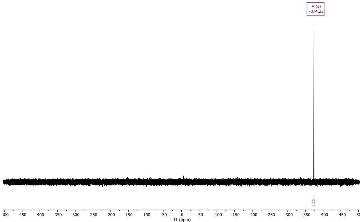
**Figure S13.**  $^{31}\text{P}\{\text{H}\}$  NMR spectrum of **2c** in  $\text{C}_6\text{D}_6$ .
