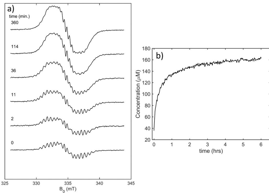
**Figure S29.** Time course of room temperature X-band CW-EPR (a.u.) of the **2a** sample dissolved in pyridine, at selected time points as indicated in panel a) and the concentration dependence of the entire signal as a function of time in panel b). The initial **2a** concentration was 20 mM. The signal evolves from a prior radical to one unresolved in features. The microwave frequency was 9.3877 GHz, and modulation amplitude of 0.1 mT.
