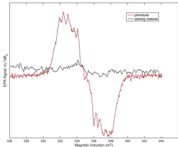
**Figure 32.** X-band CW-EPR of the photolysis product of **2b** in the presence of trimethylphosphine, leading to a spin concentration of 68 uM, from an initial concentration of **2b** of 5 mM. The microwave frequency was 9.38845 GHz, , modulation amplitude of 0.1 mT, microwave power of 1 mW, and a field offset of 0.1 mT was applied.modulation amplitude of 0.05 mT, and a microwave power of 0.1 mW.
