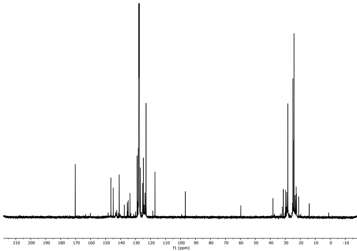
**Figure S20.**  $^{13}\text{C}$  NMR spectrum of **5** in  $\text{C}_6\text{D}_6$ .
