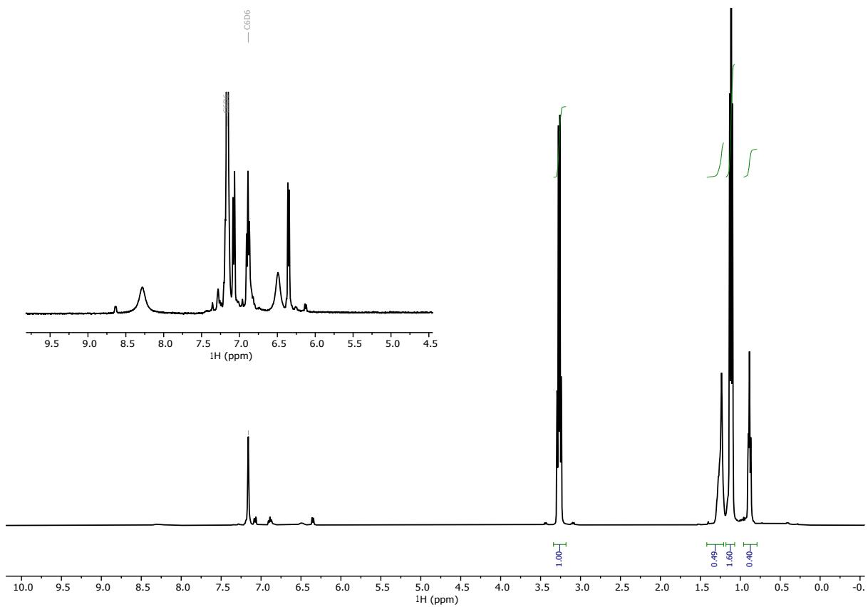
**Figure S15.** <sup>1</sup>H NMR spectrum of crystals of **3** showing residual diethyl ether and hexane. Inset: enhancement of small peaks around aromatic region.
