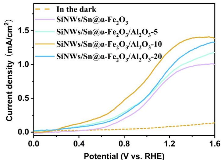
**Fig. S15**  $J$ - $V$  curves of the SiNWs/Sn@ $\alpha$ -Fe $_2$ O $_3$ /Al $_2$ O $_3$  photoanodes with 5, 10 and 20 ALD-cycle Al $_2$ O $_3$ .
