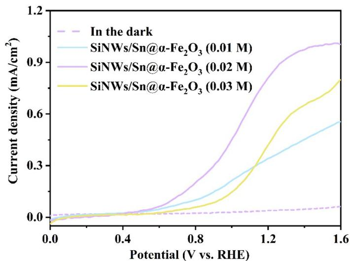
**Fig. S13**  $J$ - $V$  curves of the SiNWs/Sn@ $\alpha$ -Fe<sub>2</sub>O<sub>3</sub> prepared with 0.01 M, 0.02 M and 0.03 M Fe(NO<sub>3</sub>)<sub>3</sub> precursor solutions.
