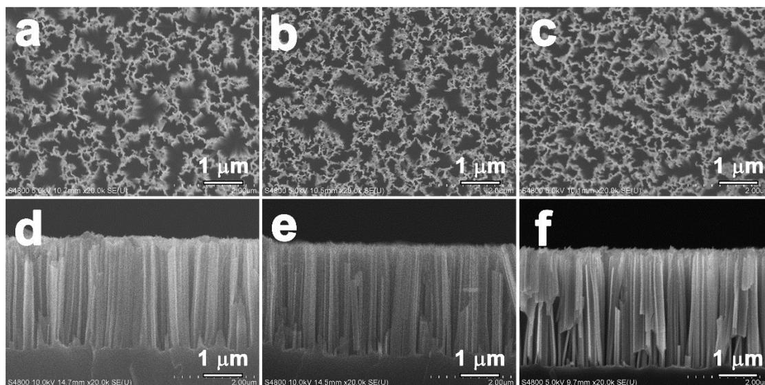
**Fig. S14** SEM images of the SiNWs/Sn@ $\alpha$ -Fe<sub>2</sub>O<sub>3</sub>/Al<sub>2</sub>O<sub>3</sub> with different thicknesses of Al<sub>2</sub>O<sub>3</sub> overlayer. (a–c) and (d–f) are the top-view and cross-section SEM images, respectively. (a and d), (b and e) and (c and f) represent the 5, 10 and 20 ALD-cycle Al<sub>2</sub>O<sub>3</sub> coated on the SiNWs/Sn@ $\alpha$ -Fe<sub>2</sub>O<sub>3</sub>, respectively.
