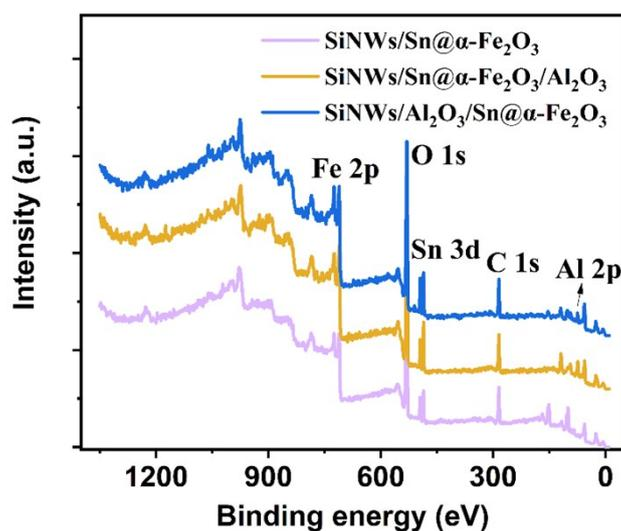
**Fig. S10** XPS spectra of the SiNWs/Sn@ $\alpha$ -Fe<sub>2</sub>O<sub>3</sub>, SiNWs/Sn@ $\alpha$ -Fe<sub>2</sub>O<sub>3</sub>/Al<sub>2</sub>O<sub>3</sub>, SiNWs/Al<sub>2</sub>O<sub>3</sub>/Sn@ $\alpha$ -Fe<sub>2</sub>O<sub>3</sub> photoanodes, respectively.
