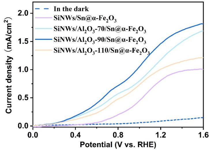
**Fig. S17**  $J$ - $V$  curves of the SiNWs/ $\text{Al}_2\text{O}_3$ /Sn@ $\alpha$ - $\text{Fe}_2\text{O}_3$  photoanodes with 70, 90 and 110 ALD-cycle  $\text{Al}_2\text{O}_3$ .
