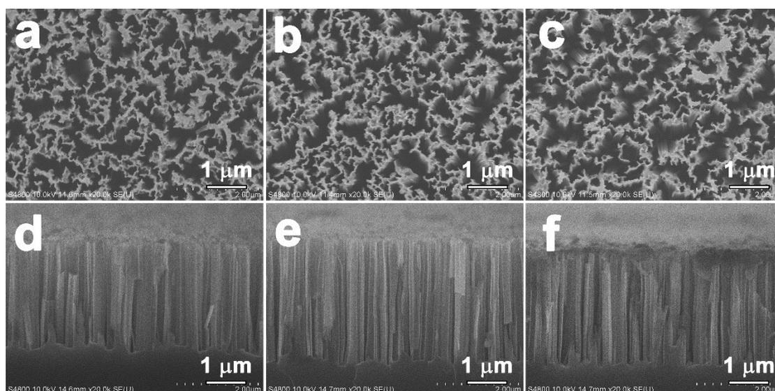
**Fig. S12** SEM images of the SiNWs/Sn@ $\alpha$ -Fe<sub>2</sub>O<sub>3</sub> with different thicknesses of Sn@ $\alpha$ -Fe<sub>2</sub>O<sub>3</sub> film. (a–c) and (d–f) are top-view and cross-section SEM images, respectively. (a and d), (b and e) and (c and f) represent the Sn@ $\alpha$ -Fe<sub>2</sub>O<sub>3</sub> films prepared with 0.01 M, 0.02 M and 0.03 M Fe(NO<sub>3</sub>)<sub>3</sub> precursor solutions, respectively.
