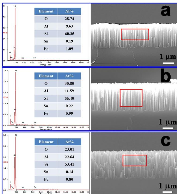
**Fig. S9** EDS comparison and corresponding SEM images in the (a) SiNWs/Sn@ $\alpha$ -Fe<sub>2</sub>O<sub>3</sub>, (b) SiNWs/Sn@ $\alpha$ -Fe<sub>2</sub>O<sub>3</sub>/Al<sub>2</sub>O<sub>3</sub> and (c) SiNWs/Al<sub>2</sub>O<sub>3</sub>/Sn@ $\alpha$ -Fe<sub>2</sub>O<sub>3</sub> photoanodes, respectively.
