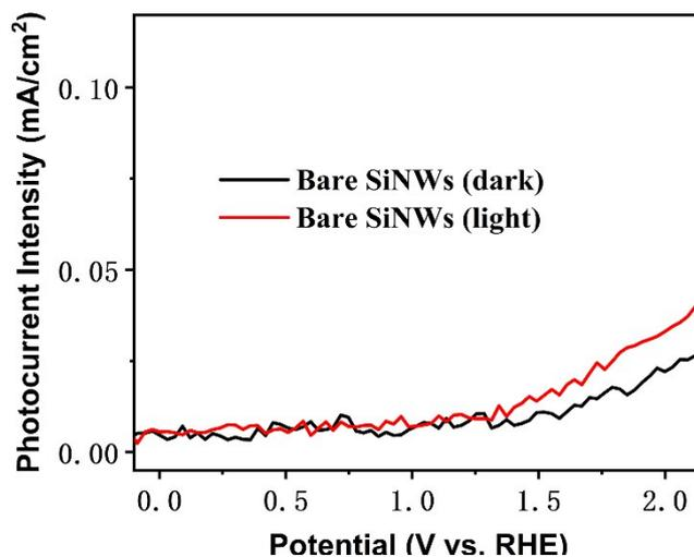
**Fig. S11** Linear scan voltammograms of SiNWs in 1 M NaOH electrolyte in dark and under simulated AM 1.5G illumination.
