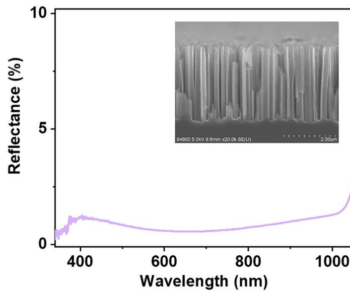
**Fig. S2** Reflectance spectrum of the as-prepared SiNWs with the length of  $\sim 3 \mu\text{m}$ , and the insert is the corresponding SEM image.
