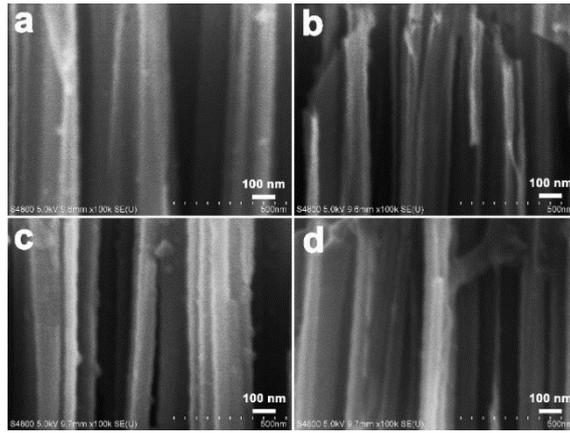
**Fig. S3** Detailed SEM images of the side regions in the prepared (a) SiNWs, (b) SiNWs/Sn@ $\alpha$ -Fe<sub>2</sub>O<sub>3</sub>, (c) SiNWs/Sn@ $\alpha$ -Fe<sub>2</sub>O<sub>3</sub>/Al<sub>2</sub>O<sub>3</sub> and (d) SiNWs/Al<sub>2</sub>O<sub>3</sub>/Sn@ $\alpha$ -Fe<sub>2</sub>O<sub>3</sub>.
