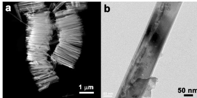
**Fig. S4** TEM images of the Si/Sn@ $\alpha$ -Fe<sub>2</sub>O<sub>3</sub> nanowire heterostructures scraped from the substrate.
