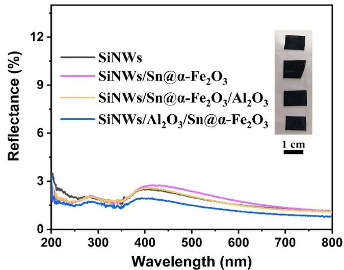
**Fig. S8** Reflectance spectra of the as-prepared SiNWs, SiNWs/Sn@ $\alpha$ -Fe<sub>2</sub>O<sub>3</sub>, SiNWs/Sn@ $\alpha$ -Fe<sub>2</sub>O<sub>3</sub>/Al<sub>2</sub>O<sub>3</sub> and SiNWs/Al<sub>2</sub>O<sub>3</sub>/Sn@ $\alpha$ -Fe<sub>2</sub>O<sub>3</sub> photoanodes. The corresponding digital photographs are shown in the insert.
