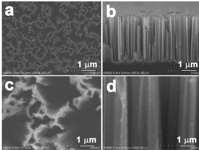
**Fig. S1** SEM images of the as-prepared SiNWs. (a and b) are the top-view and cross-section SEM images, (c and d) are the detailed views of the top and side regions, respectively.
