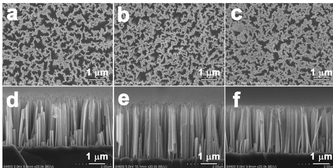
**Fig. S16** SEM images of the SiNWs/Al $_2$ O $_3$ /Sn@ $\alpha$ -Fe $_2$ O $_3$  with different thicknesses of Al $_2$ O $_3$  interlayer. (a–c) and (d–f) are the top-view and cross-section SEM images, respectively. (a and d), (b and e) and (c and f) represent the 70, 90 and 110 ALD-cycle Al $_2$ O $_3$  coated on the SiNWs substrate and buried by the Sn@ $\alpha$ -Fe $_2$ O $_3$  film, respectively.
