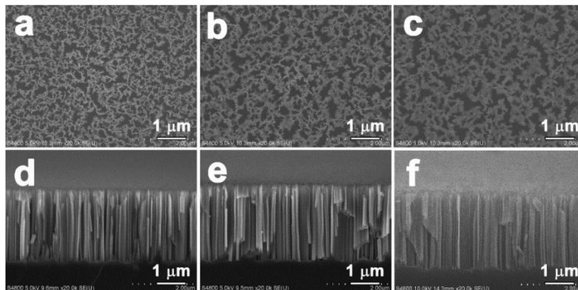
**Fig. S5** SEM images of the SiNWs/Al<sub>2</sub>O<sub>3</sub> photoanodes with different thicknesses of Al<sub>2</sub>O<sub>3</sub> film. (a–c) and (d–f) are the top-view and cross-section SEM images, respectively. (a and d), (b and e) and (c and f) represent the 10, 50 and 100 ALD-cycle Al<sub>2</sub>O<sub>3</sub> coated on the SiNWs, respectively.
