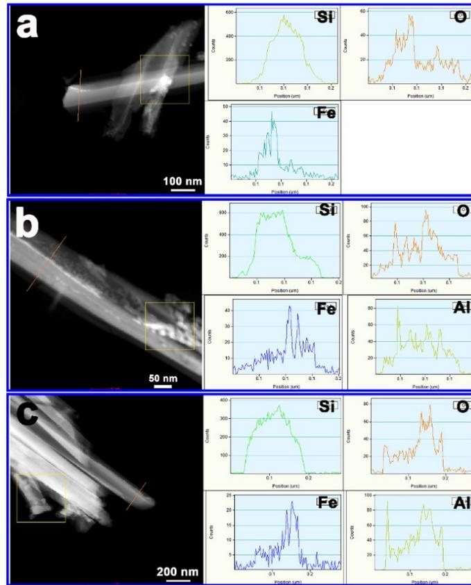
**Fig. S7.** STEM-EDS comparison in the (a) SiNWs/Sn@ $\alpha$ -Fe<sub>2</sub>O<sub>3</sub>, (b) SiNWs/Sn@ $\alpha$ -Fe<sub>2</sub>O<sub>3</sub>/Al<sub>2</sub>O<sub>3</sub> and (c) SiNWs/Al<sub>2</sub>O<sub>3</sub>/Sn@ $\alpha$ -Fe<sub>2</sub>O<sub>3</sub> nanowire heterostructures, respectively.
