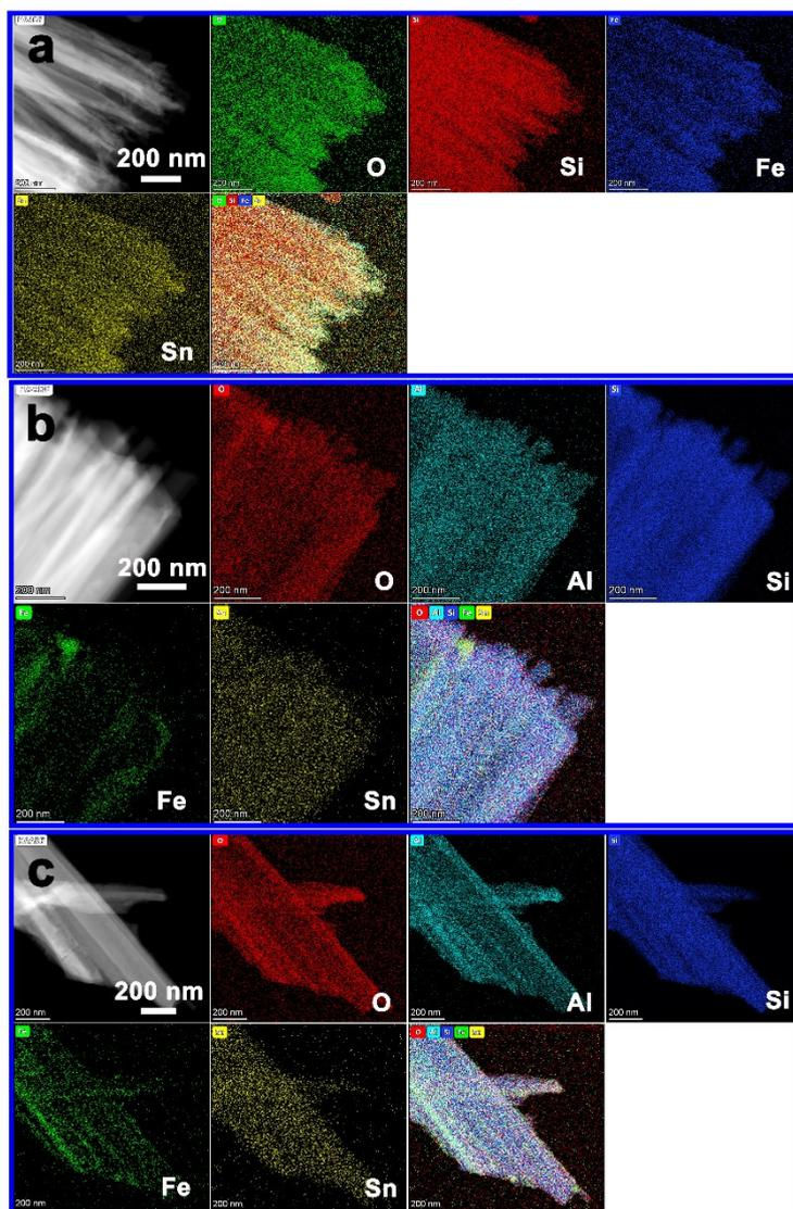
**Fig. S6** STEM-EDS analysis of the (a) SiNWs/Sn@ $\alpha$ -Fe<sub>2</sub>O<sub>3</sub>, (b) SiNWs/Sn@ $\alpha$ -Fe<sub>2</sub>O<sub>3</sub>/Al<sub>2</sub>O<sub>3</sub> and (c) SiNWs/Al<sub>2</sub>O<sub>3</sub>/Sn@ $\alpha$ -Fe<sub>2</sub>O<sub>3</sub> nanowire heterostructures, respectively.
