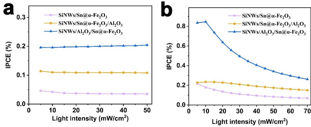
**Fig. S19** Incident photon-to-current conversion efficiency (IPCE) as a function of light power density of the SiNWs/Sn@ $\alpha$ -Fe<sub>2</sub>O<sub>3</sub>, SiNWs/Sn@ $\alpha$ -Fe<sub>2</sub>O<sub>3</sub>/Al<sub>2</sub>O<sub>3</sub>, SiNWs/Al<sub>2</sub>O<sub>3</sub>/Sn@ $\alpha$ -Fe<sub>2</sub>O<sub>3</sub> photoanodes under (a)  $\lambda=365$  nm and (b)  $\lambda=620$  nm irradiation.
