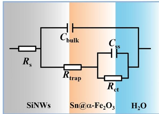
**Fig. S18** The employed equivalent circuit for EIS analysis.
