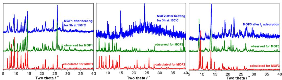
Figure S2. The comparison of the observed, calculated and PXRD patterns after heating or  $I_2$  adsorption for the three reported MOFs.
