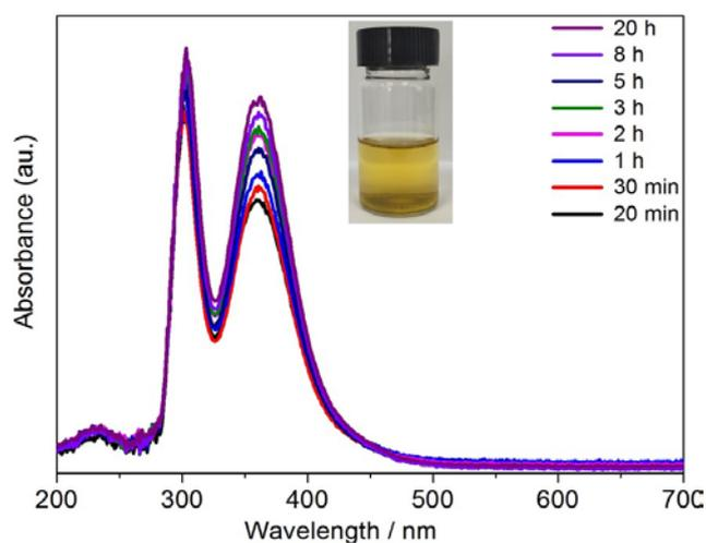
Figure S3. The UV-vis spectra of I<sub>2</sub> release process in ethanol.
