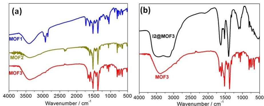
Figure S1. The FT- IR spectra of the three MOFs presented in this paper.
