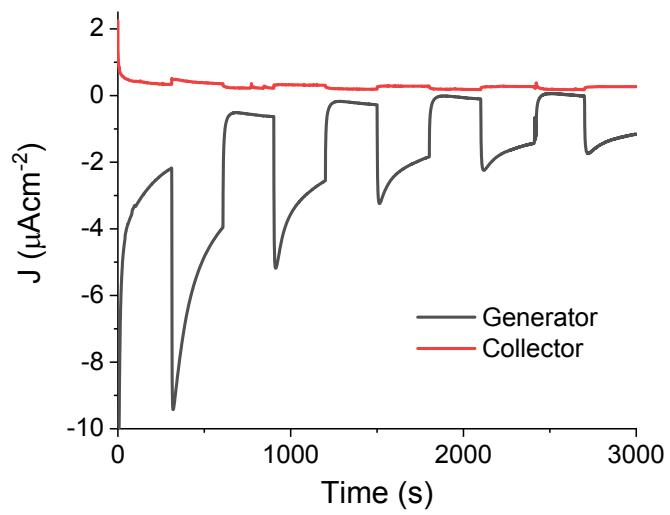
**Figure S22.** Faradaic efficiency determination for photoelectrochemical hydrogen production by NiO|(MAA)QDs at 0 V vs. NHE under chopped irradiation ( $100 \text{ mW}\cdot\text{cm}^{-2}$ ) in 0.1 M acetate buffer at pH 4. The black trace is the produced photocurrent generated by the NiO electrode (generator), whereas the red trace represents the current registered at the FTO|Pt electrode (collector) held at +0.4 V vs. NHE.
