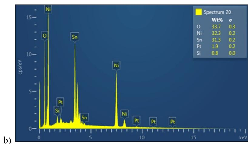
**Figure S15.** (a) SEM image of NiO|(MAA)QDs|Pt(100s) and (b) EDS analysis.
