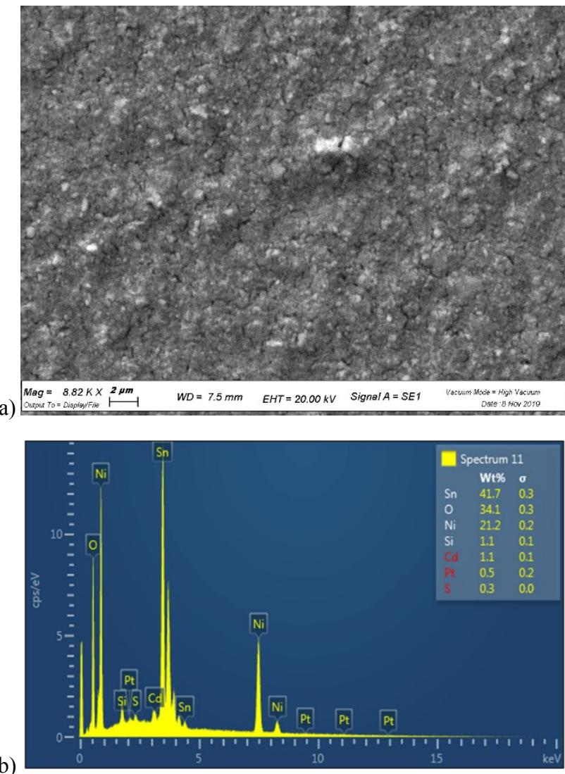
**Figure S13.** (a) SEM image of NiO|(MAA)QDs|Pt(20s) and (b,c) EDS analysis.
