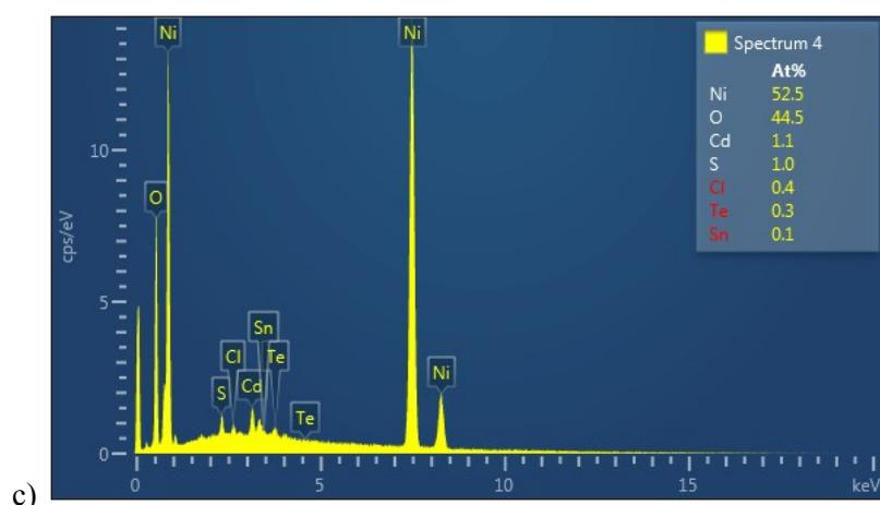
**Figure S2.** (a) SEM image of NiO|(MPA)QDs and (b,c) EDS analysis.
