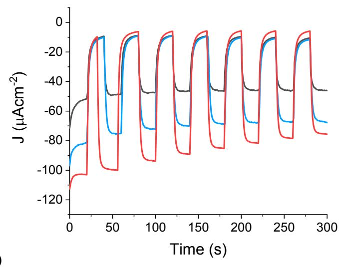
**Figure S11.** a) Linear sweep voltammetry (recorded at a scan rate of  $10 \text{ mV}\cdot\text{s}^{-1}$ ) and b) chronoamperometry at  $0 \text{ V}$  vs. NHE under chopped irradiation ( $100 \text{ mW}\cdot\text{cm}^{-2}$ ) of NiO|QDs electrodes with different capping agents in the presence of  $20 \text{ mM} [\text{Co}^{\text{III}}(\text{NH}_3)_5\text{Cl}]\text{Cl}_2$  as an irreversible electron acceptor ( $0.1 \text{ M}$  acetate buffer at  $\text{pH } 4$ ).
