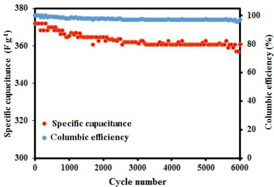
Figure S3. The columbic efficiency of the SPc at 4.5 A g<sup>-1</sup> for 6000 cycles.
