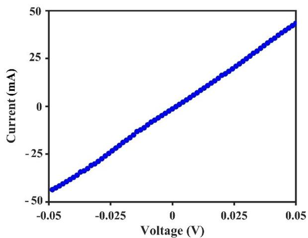
Figure S2. I-V curve of the SPc pellet employed for the conductivity measurements.
