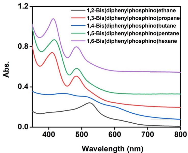
Figure S2. The UV-Vis spectra of crude product synthesized via adding phosphine ligands with different chain lengths
