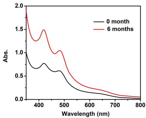
Figure S4. UV-vis spectra of  $[\text{Ag}_{13}\text{Cu}_{10}(\text{C}_{10}\text{H}_{15}\text{S})_{12}]X_3$  which stored in solid state for more than 6 months.
