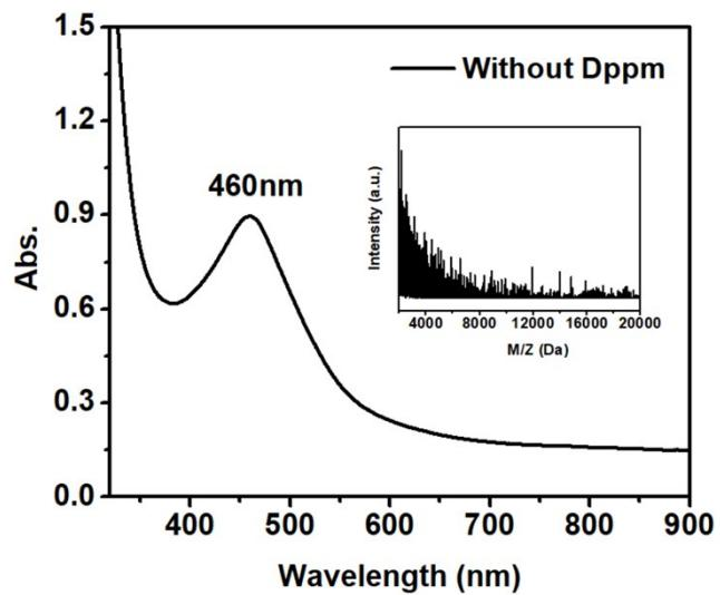
Figure S1. The UV-vis spectrum and MALDI spectrum of product synthesized without Dppm ligand during the synthesis process.
