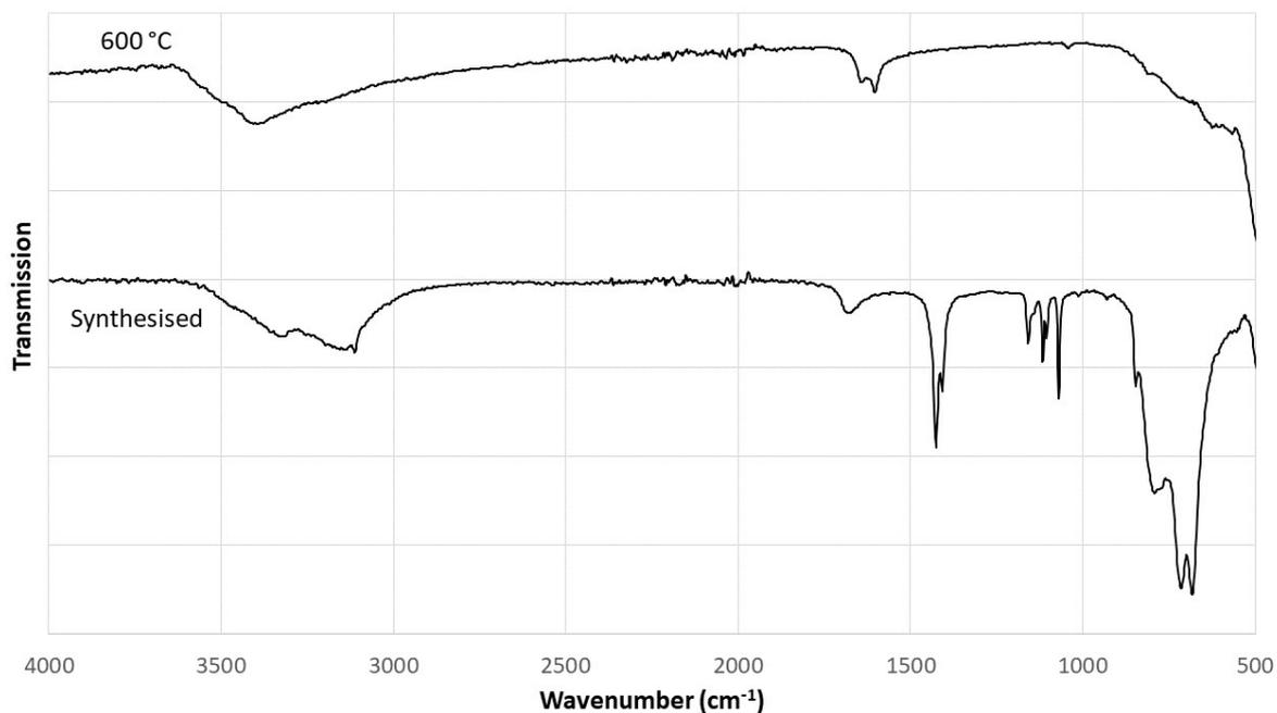
**Figure S19** – IR spectra of  $[\text{Ni}(\text{SiF}_6)(\text{pyrazine})(\text{H}_2\text{O})_2]$  as synthesised and the residue prepared by heating  $[\text{Ni}(\text{SiF}_6)(\text{pyrazine})(\text{H}_2\text{O})_2]$  samples at 10 °C/min under  $\text{N}_2$  atmosphere to the quoted temperature.
