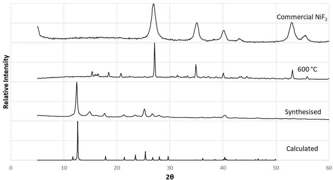
**Figure S12** – PXRD spectra of [SIFSIX-3-Ni] as calculated from single crystal data; as synthesised; residue isolated by heating [SIFSIX-3-Ni] samples at 10 °C/min under  $N_2$  atmosphere to the quoted temperature, and a commercial sample of  $NiF_2$ .
