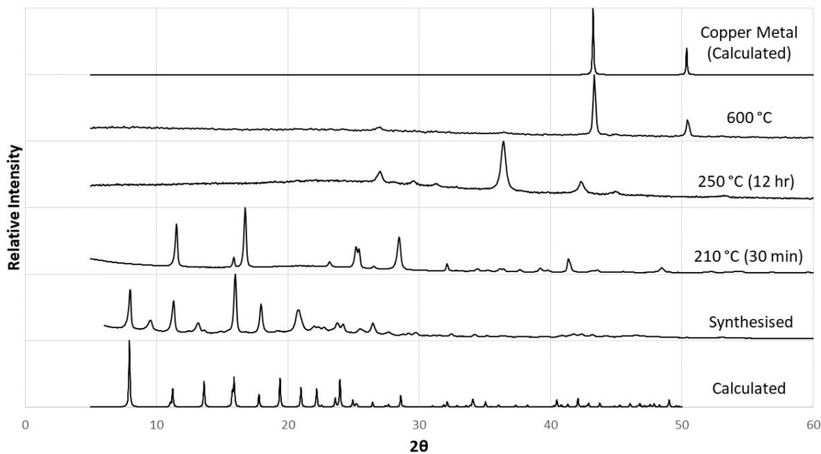
**Figure S16** – PXRd spectra of [SIFSIX-1-Cu] as calculated from single crystal data; as synthesised; residues isolated by heating [SIFSIX-1-Cu] samples at 10 °C/min under N<sub>2</sub> atmosphere to the quoted temperatures (and hold times), and; copper metal.
