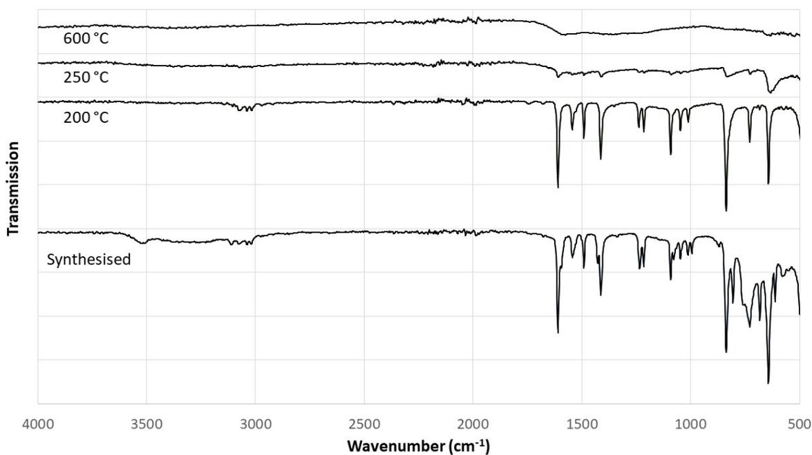
**Figure S22** – IR spectra of [SIFSIX-1-Cu] as synthesised and the residues prepared by heating [SIFSIX-1-Cu] samples at 10 °C/min under N<sub>2</sub> atmosphere to the quoted temperatures.
