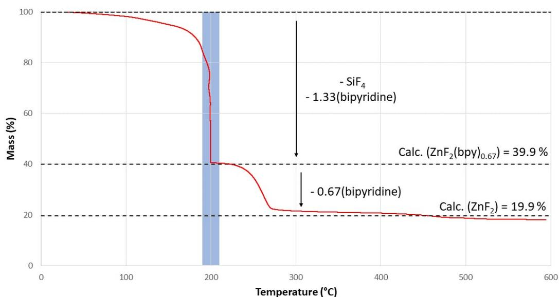
**Figure S6** – Ramp-hold-ramp TGA trace of [SIFSIX-1-Zn] under N<sub>2</sub> atmosphere. The sample was heated to 200 °C at a constant rate of 10 °C/min, held at this temperature for 30 minutes (indicated by blue region), and subsequently ramped to 600 °C at a constant rate of 10 °C/min.
