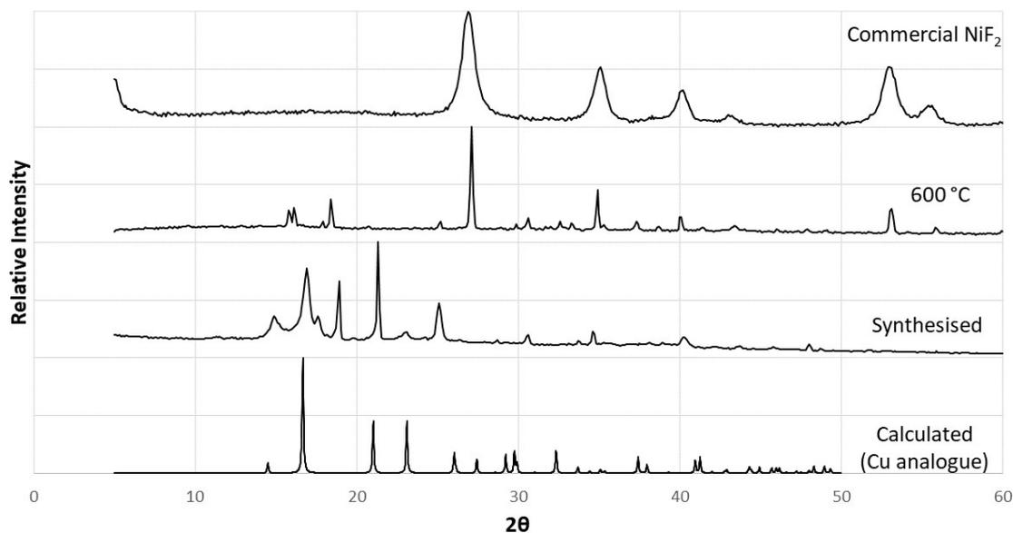
**Figure S13** – PXR D spectra of  $[\text{Ni}(\text{SiF}_6)(\text{pyrazine})(\text{H}_2\text{O})_2]$  as calculated from single crystal data (Cu analogue); as synthesised; residue isolated by heating  $[\text{Ni}(\text{SiF}_6)(\text{pyrazine})(\text{H}_2\text{O})_2]$  samples at 10 °C/min under  $\text{N}_2$  atmosphere to the quoted temperature, and a commercial sample of  $\text{NiF}_2$ .
