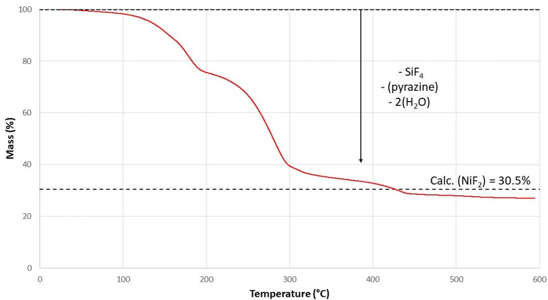
**Figure S3** – TGA trace of  $[\text{Ni}(\text{SiF}_6)(\text{pyrazine})(\text{H}_2\text{O})_2]$  under constant heating at 10 °C/min under N<sub>2</sub> atmosphere.
