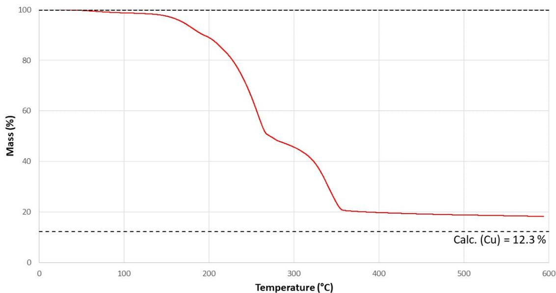
**Figure S8** – TGA trace of [SIFSIX-1-Cu] under constant heating at 10 °C/min under N<sub>2</sub> atmosphere. This sample was activated at 150 °C for 30 minutes at ambient pressure before analysis. PXRD analysis (see below) indicates that metallic Cu is present in the residue, not CuF<sub>2</sub>. The additional mass is assigned as amorphous carbon.
