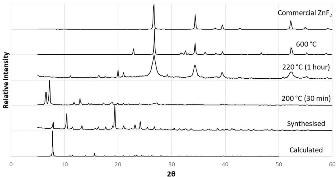
**Figure S15** – PXRd spectra of [SIFSIX-1-Zn] as calculated from single crystal data; as synthesised; residues isolated by heating [SIFSIX-1-Zn] samples at 10 °C/min under N<sub>2</sub> atmosphere to the quoted temperatures (and hold times), and; ZnF<sub>2</sub>.
