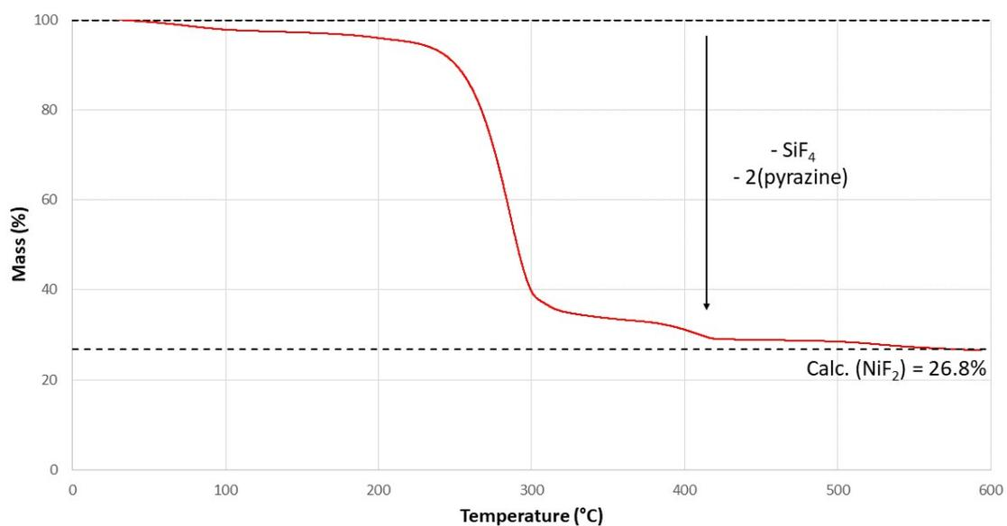
Figure S2 – TGA trace of [SIFSIX-3-Ni] under constant heating at 10 °C/min under N<sub>2</sub> atmosphere.
