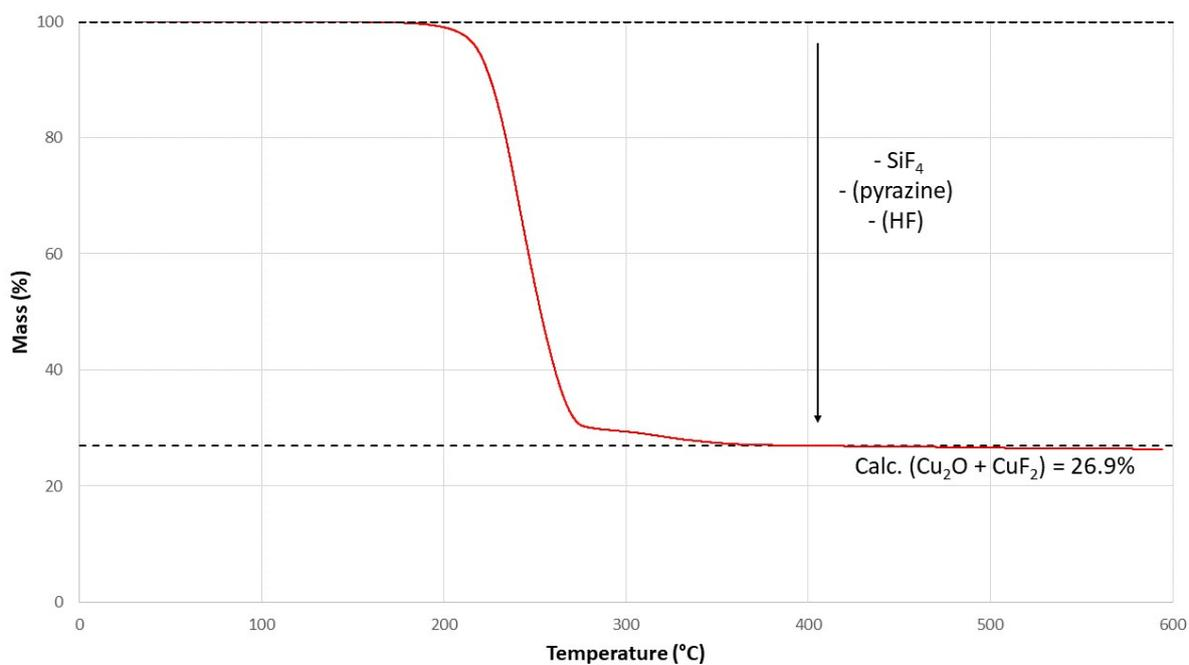
**Figure S4** – TGA trace of  $[\text{Cu}(\text{SiF}_6)(\text{pyrazine})(\text{H}_2\text{O})_2]$  under constant heating at 10 °C/min under N<sub>2</sub> atmosphere. The quoted residual weight (26.9%) is calculated assuming a 50:50 mixture of Cu<sub>2</sub>O and CuF<sub>2</sub>.
