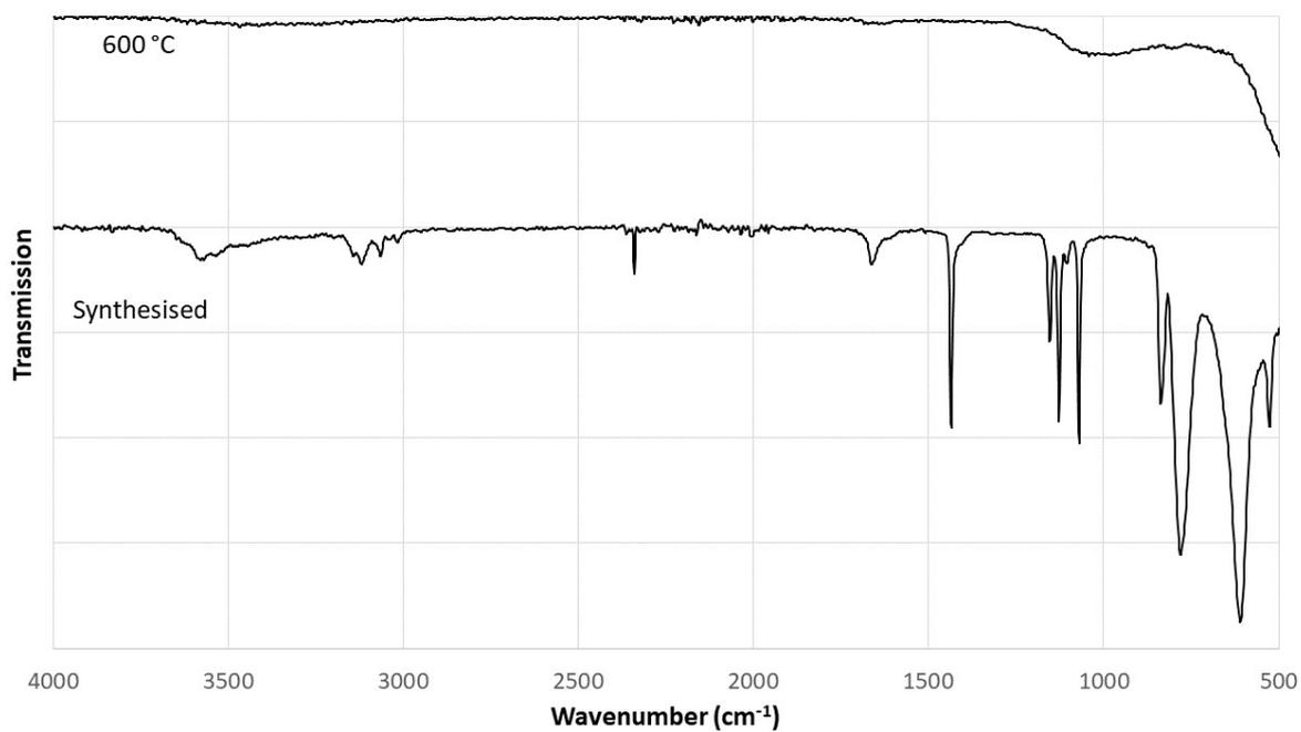
**Figure S18** – IR spectra of [SIFSIX-3-Ni] as synthesised and the residue prepared by heating [SIFSIX-3-Ni] samples at 10 °C/min under N<sub>2</sub> atmosphere to the quoted temperature.
