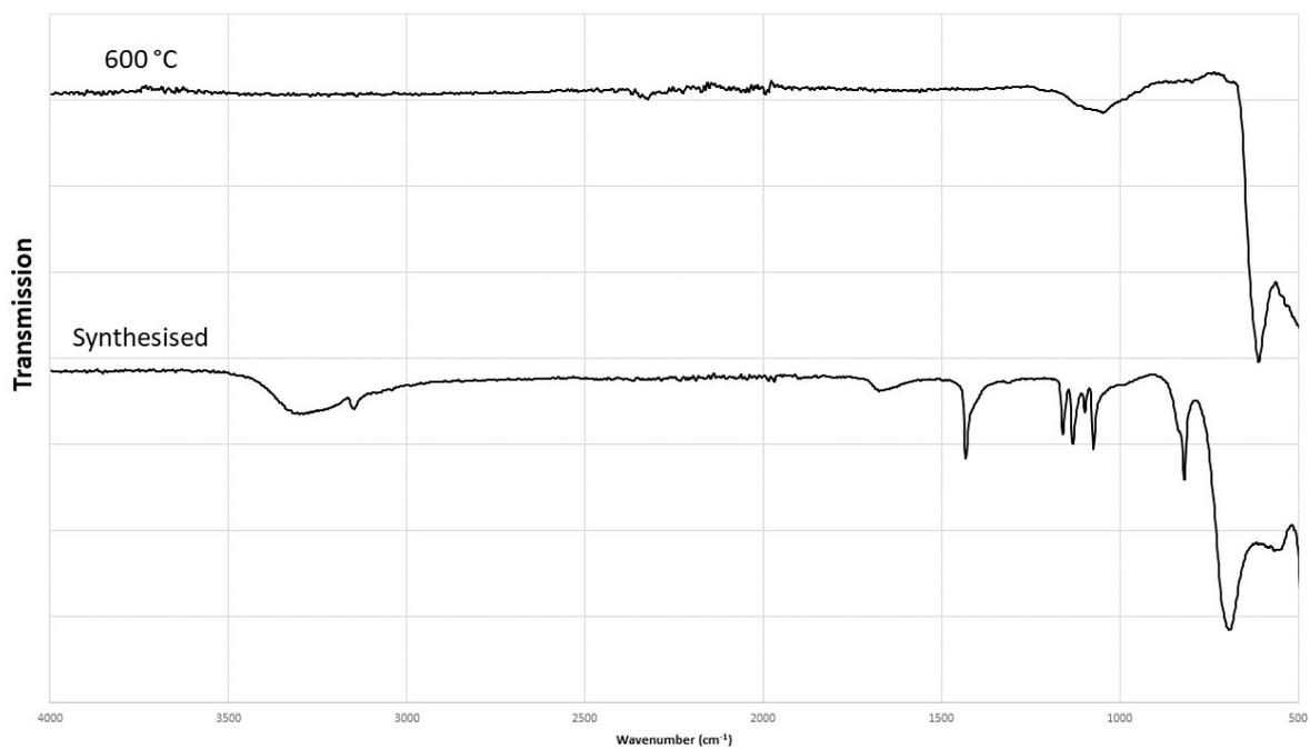
**Figure S20** – IR spectra of  $[\text{Cu}(\text{SiF}_6)(\text{pyrazine})(\text{H}_2\text{O})_2]$  as synthesised and the residue prepared by heating  $[\text{Cu}(\text{SiF}_6)(\text{pyrazine})(\text{H}_2\text{O})_2]$  samples at 10 °C/min under  $\text{N}_2$  atmosphere to the quoted temperature.
