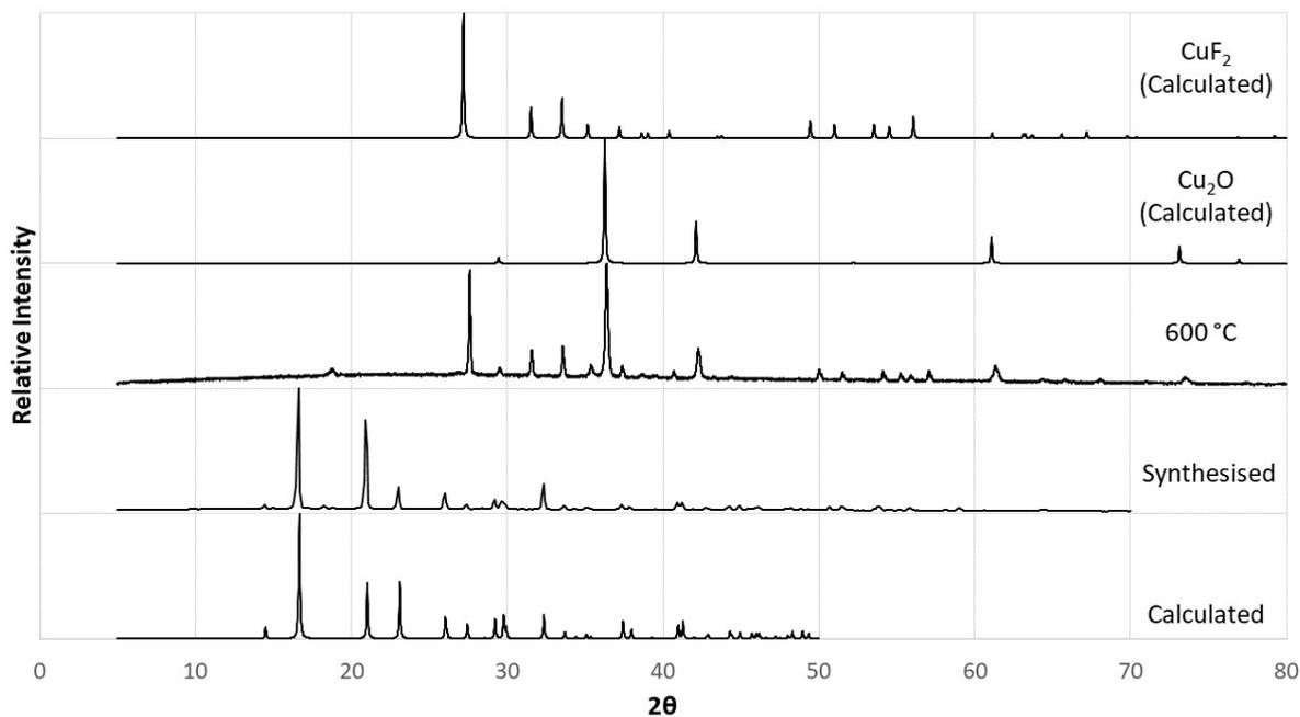
**Figure S14** – PXR D spectra of  $[\text{Cu}(\text{SiF}_6)(\text{pyrazine})(\text{H}_2\text{O})_2]$  as calculated from single crystal data; as synthesised; residue isolated by heating  $[\text{Cu}(\text{SiF}_6)(\text{pyrazine})(\text{H}_2\text{O})_2]$  samples at 10 °C/min under  $\text{N}_2$  atmosphere to the quoted temperature, and;  $\text{Cu}_2\text{O}$  and  $\text{CuF}_2$  as calculated from literature data.
