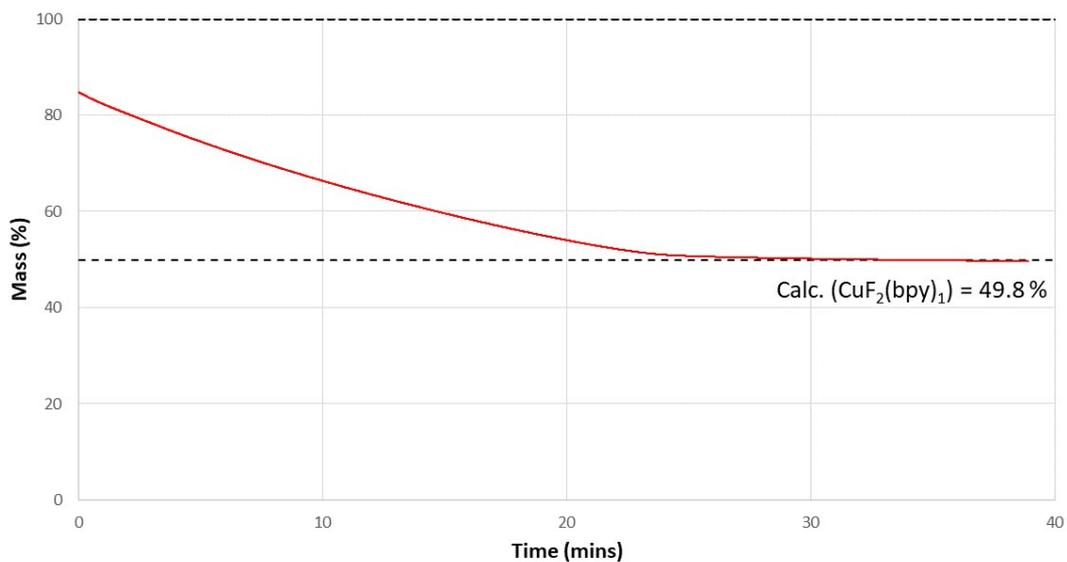
**Figure S9** – Time course TGA of [SIFSIX-1-Cu] held at 210 °C under N<sub>2</sub> atmosphere for 40 minutes. This sample was activated at 150 °C for 30 minutes at ambient pressure before analysis.
