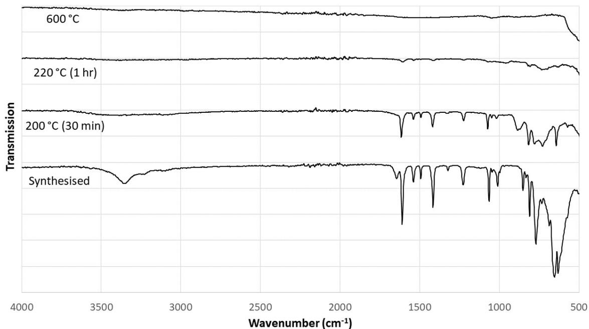
**Figure S21** – IR spectra of [SIFSIX-1-Zn] as synthesised and the residues prepared by heating [SIFSIX-1-Zn] samples at 10 °C/min under N<sub>2</sub> atmosphere to the quoted temperatures (and hold times).
