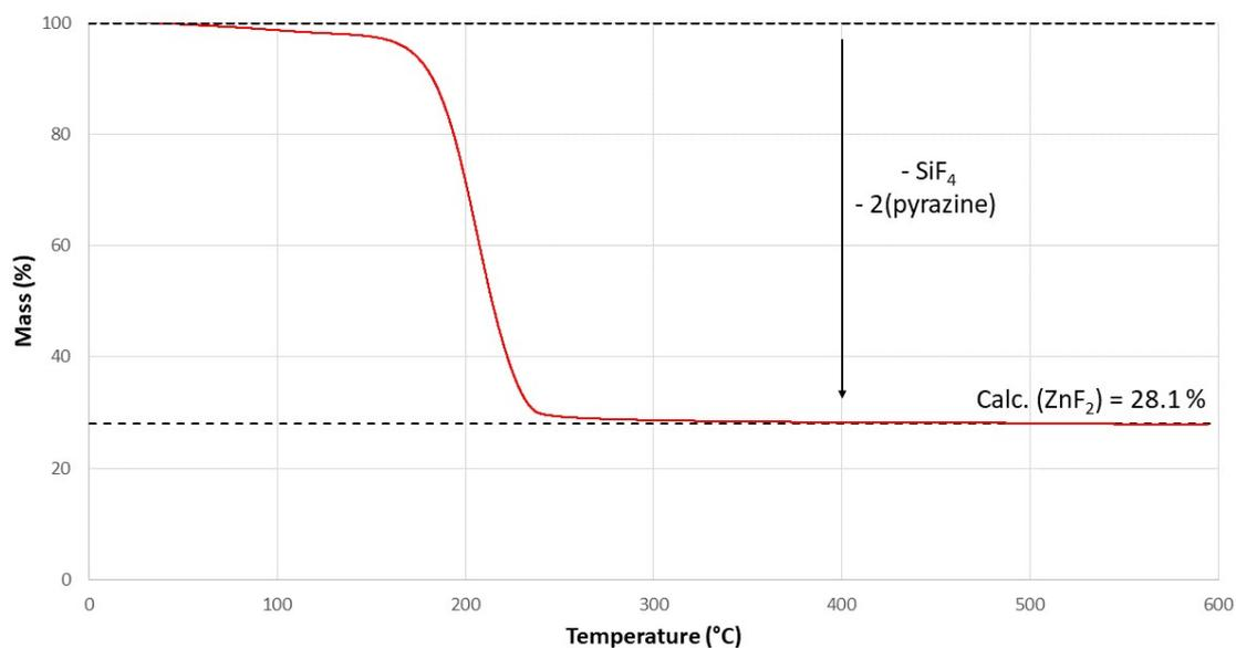
Figure S1 – TGA trace of [SIFSIX-3-Zn] under constant heating at 10 °C/min under N<sub>2</sub> atmosphere.
