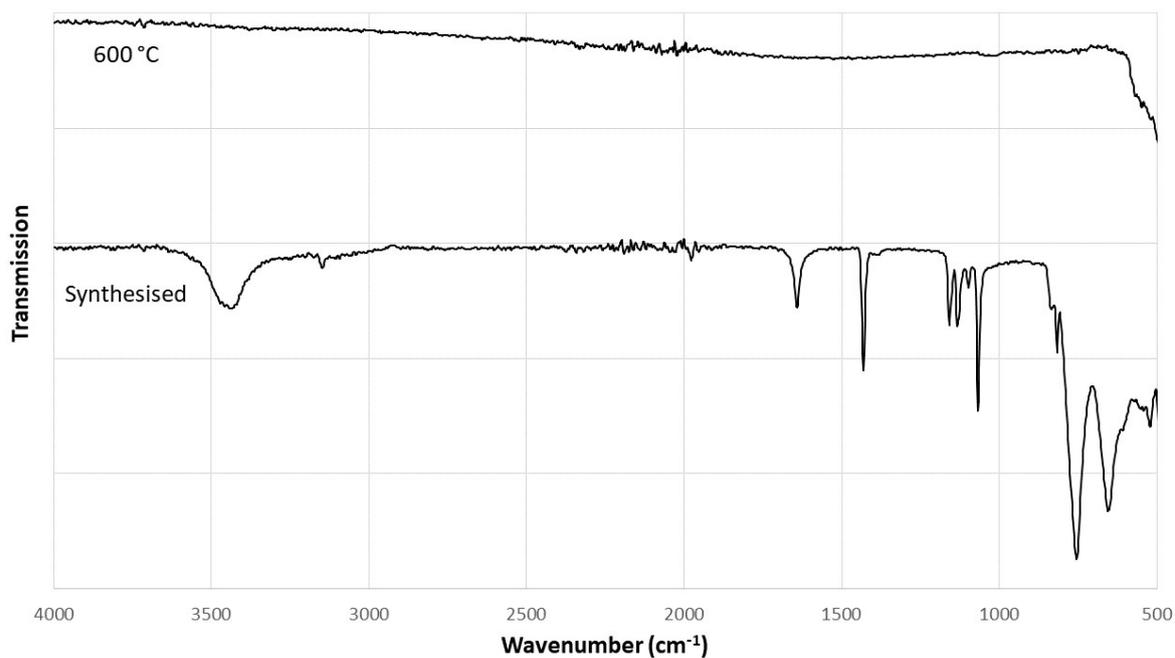
**Figure S17** – IR spectra of [SIFSIX-3-Zn] as synthesised and the residue prepared by heating [SIFSIX-3-Zn] samples at 10 °C/min under N<sub>2</sub> atmosphere to the quoted temperature.
