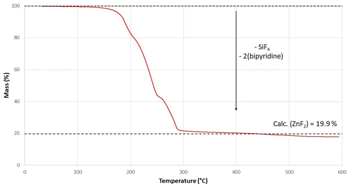
**Figure S5** – TGA trace of [SIFSIX-1-Zn] under constant heating at 10 °C/min under N<sub>2</sub> atmosphere.
