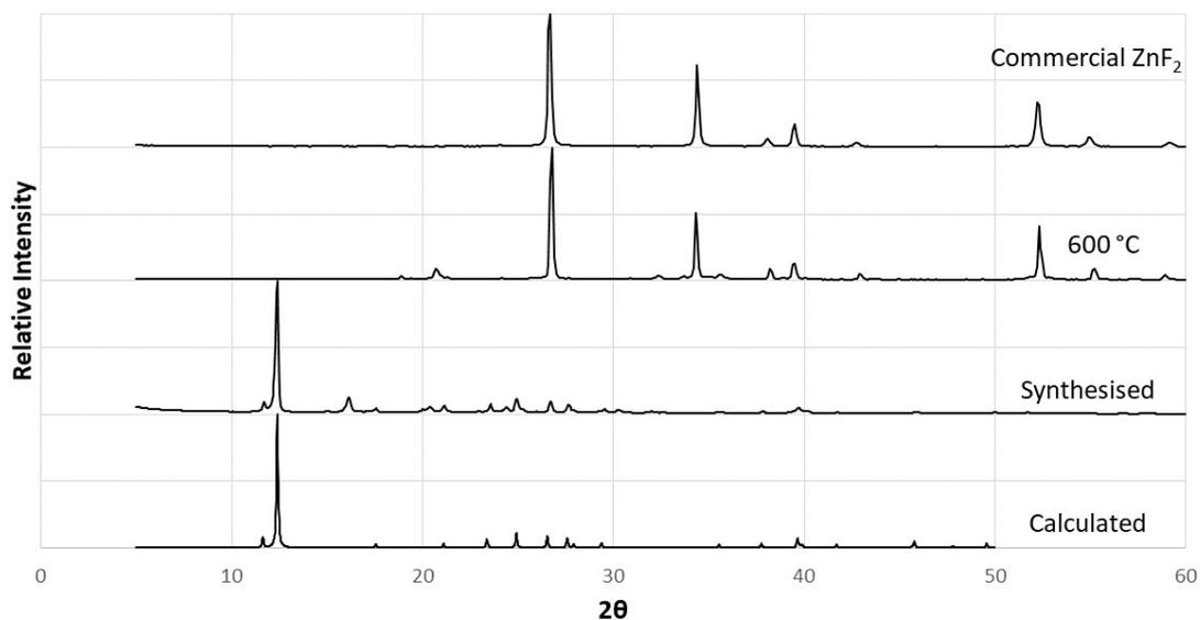
**Figure S11** – PXRD spectra of [SIFSIX-3-Zn] as calculated from single crystal data; as synthesised; residue isolated by heating [SIFSIX-3-Zn] samples at 10 °C/min under  $N_2$  atmosphere to the quoted temperature, and a commercial sample of  $ZnF_2$ .
