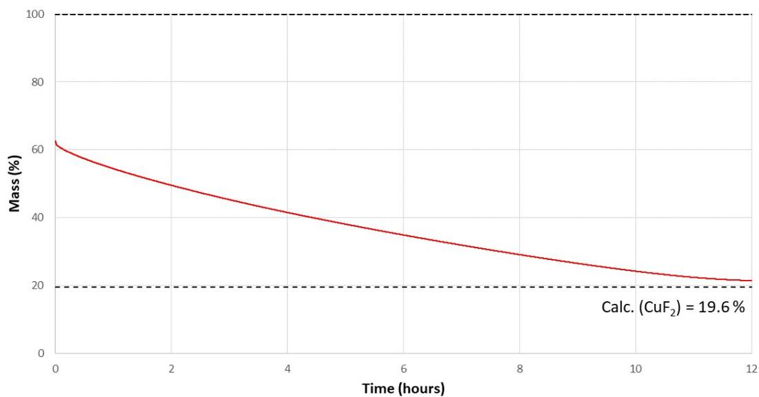
**Figure S10** – Time course TGA of [SIFSIX-1-Cu] held at 250 °C under N<sub>2</sub> atmosphere for 12 hours. This sample was activated at 150 °C for 30 minutes at ambient pressure before analysis.
