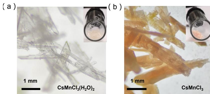
**Figure S3.** (a) and (b) display optical photographs of CMCH-1 and CMC crystal, respectively.
