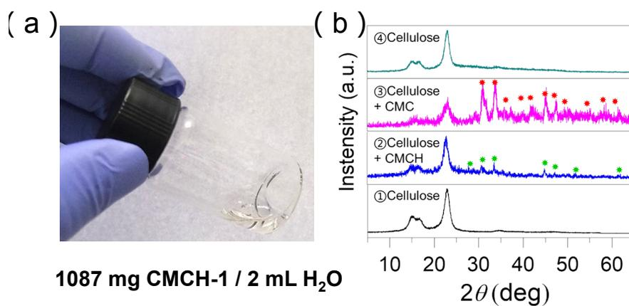
**Figure S8.** CMCH-1 aqueous solution (a). The PXRD of the products during the CMCH-1 and CMC structural transformation in the filter paper (b): ① the PXRD of blank filter paper; ② the PXRD of filter paper printed by CMCH-1 aqueous solution; ③ the PXRD of ② after heat treatment at 125 °C for 30 min; ④ the PXRD of ③ after water vapour treatment.
