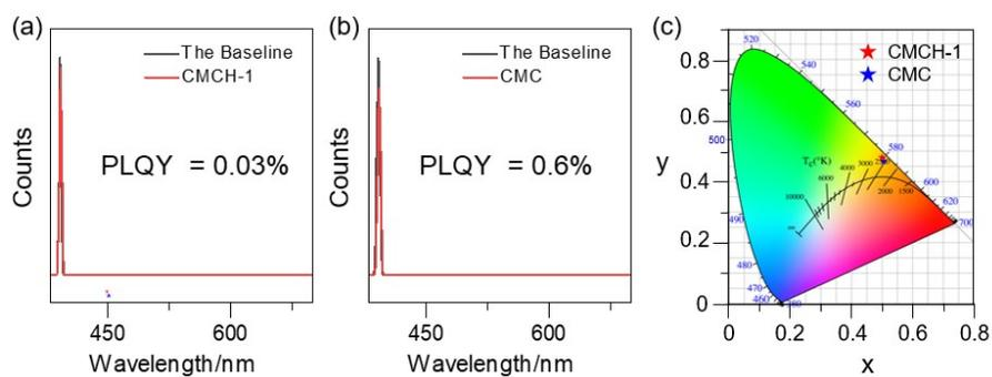
**Figure S6.** Photoluminescence quantum yield (PLQY) of CMCH-1 (a) and CMC (b). The coordinate of CMCH-1 and CMC in CIE map (c).
