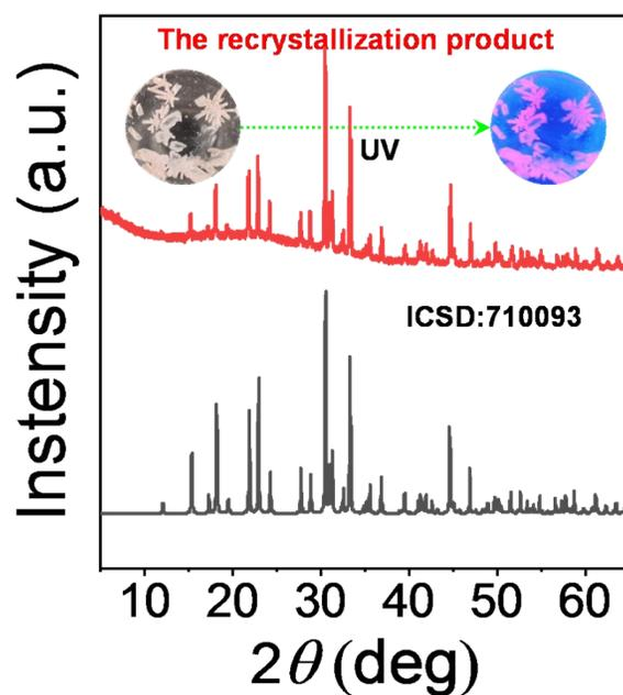
**Figure S7.** PXRD pattern of CMCH-1 compound recrystallized from aqueous solution (the inserts show compound under natural light and UV light, respectively).
