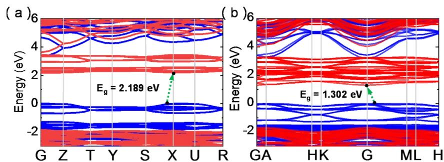
**Figure S9.** Band structure of CMCH (a) and CMC (b). Blue and red represent the spin-up and spin-down, respectively.
