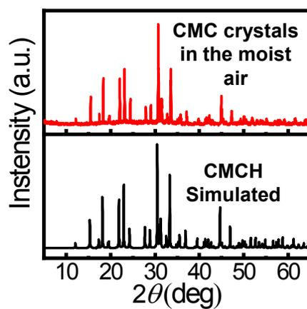
**Figure S4.** Experimental PXRD shows the product of CMC crystals in the moist air for 24 h. Obviously, CMC can convert into CMCH under moisture treatment.
