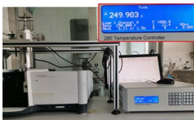
Figure S1. The variable temperature fluorescence test systems.
