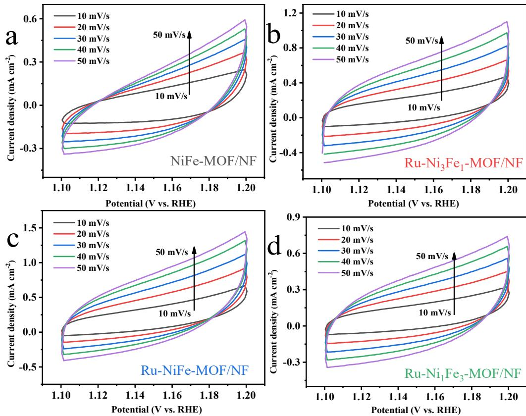
**Fig.S5CV** curves of (a)NiFe-MOF/NF,(b) Ru-Ni<sub>3</sub>Fe<sub>1</sub>-MOF/NF,(c) Ru-NiFe-MOF/NF, and (d) Ru-Ni<sub>1</sub>Fe<sub>3</sub>-MOF/NF catalysts with various scan rates (10, 20, 30, 40, and 50 mV/s) toward OER 1 M KOH.
