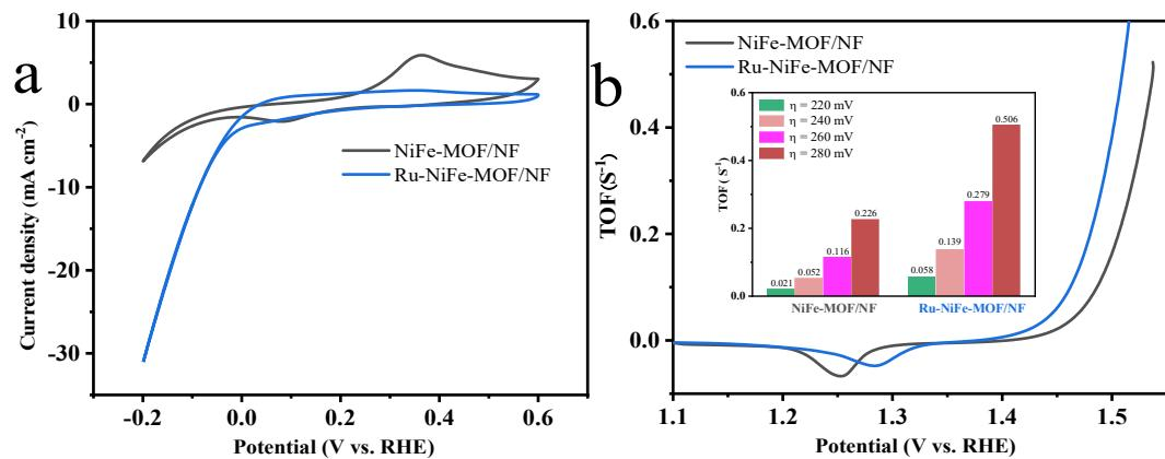
**Fig. S4** (a) CV curves of NiFe-MOF/NF and Ru-NiFe-MOF/NF catalysts in the potential range from -0.2 to 0.6 V (vs. RHE) in 1 M PBS (pH=7) with scan rate of 50 mVs⁻¹. (b) Calculated TOFs of NiFe-MOF/NF and Ru-NiFe-MOF/NF for OER (inset shows the corresponding TOFs at special overpotentials of 220, 240, 260, and 280 mV, respectively).
