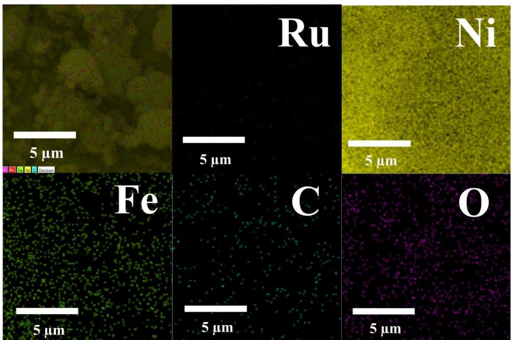
**Fig.S6** EDX elemental mapping of Ru-NiFe-MOF/NF after long-term stability test.
