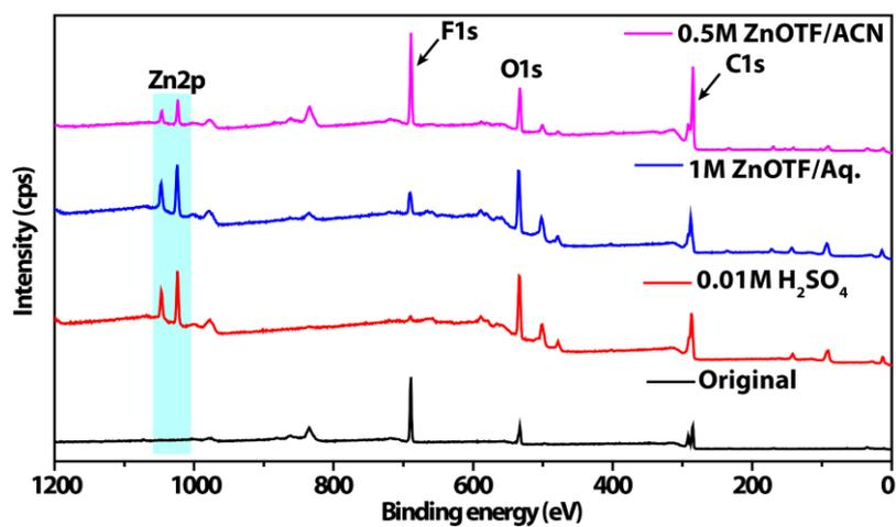
**Figure S5.** XPS survey spectra of the NTCDA electrodes at the original state and after recovering from the NTCDA||Zn-(N), NTCDA||Zn-(A), and NTCDA||Zn-(O) cells at the discharged state.
