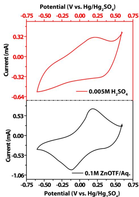
**Figure S11.** CV profiles for the MnO<sub>2</sub> electrode characterized in the three-electrode cell with respect to the Hg/Hg<sub>2</sub>SO<sub>4</sub> reference electrode in 0.005M H<sub>2</sub>SO<sub>4</sub> and 0.1M ZnOTF/Aq. electrolytes.
