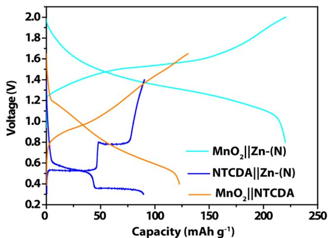
**Figure S12.** Charge/discharge capacities of the MnO<sub>2</sub>||Zn-(N), NTCDA||Zn-(N), and MnO<sub>2</sub>||NTCDA cells recorded at the current rate of 0.50 A g<sup>-1</sup> (here, the capacity values and current rate are normalized with respect to the mass-loading of the electrode material in the positive electrode).
