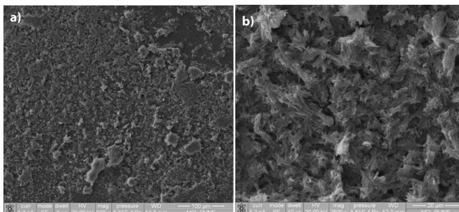
**Figure S9.** (a)-(b) SEM images of the NTCDA electrode recovered from the NTCDA||Zn-(N) half-cell after the cycling stability test (the electrode was washed with water and dried before the SEM analysis).
