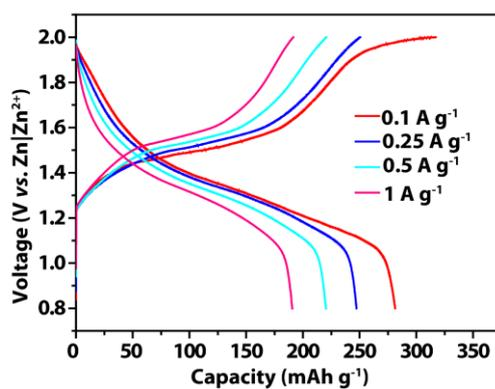
**Figure S10.** GCD profiles of the MnO<sub>2</sub>||Zn-(N) half-cell recorded at different current rates.
