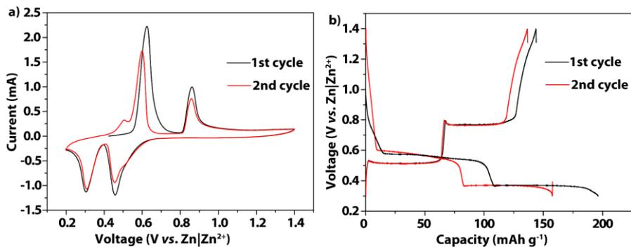
**Figure S2.** (a) CV profiles recorded at the scan rate of  $1.0 \text{ mV s}^{-1}$  and (b) GCD profiles recorded at the current rate of  $0.1 \text{ A g}^{-1}$  for the NTCDA||Zn cell.
