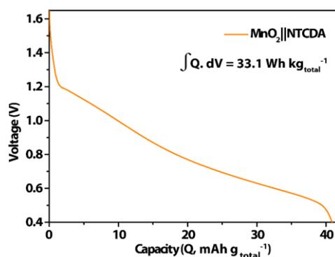
**Figure S13.** Voltage vs. discharge capacity plot of the MnO<sub>2</sub>||NTCDA full-cell recorded at a current rate of 0.17 A g<sub>total</sub><sup>-1</sup>.
