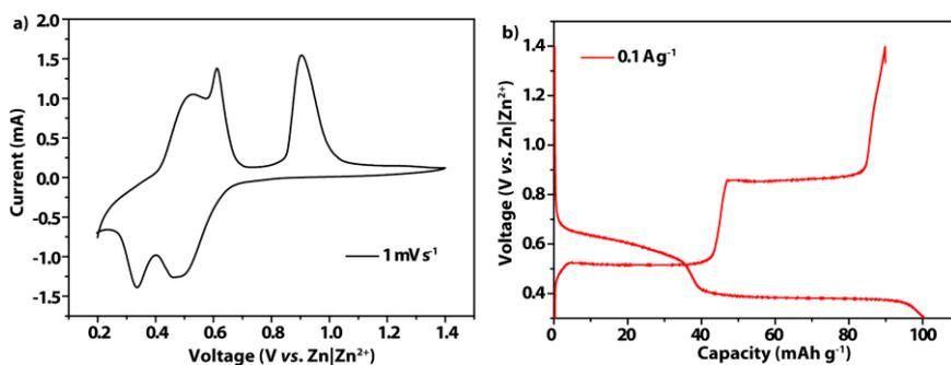
**Figure S4.** (a) CV profile recorded at the scan rate of  $1.0 \text{ mV s}^{-1}$  and (b) GCD profile recorded at the current rate of  $0.1 \text{ A g}^{-1}$  for the NTCDA||Zn-(A) cell in  $0.01 \text{ M H}_2\text{SO}_4$  electrolyte.
