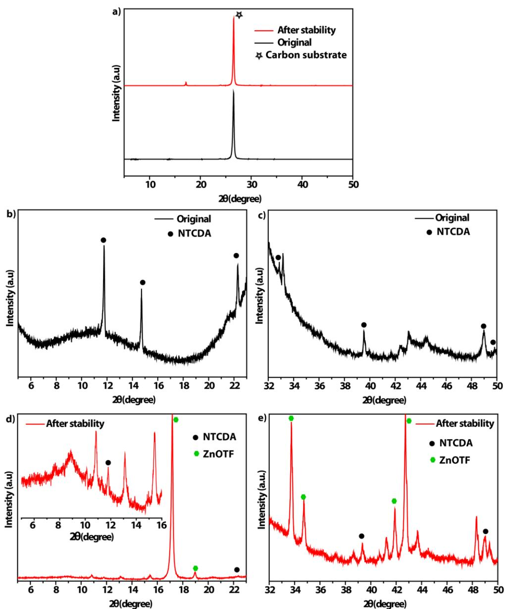
**Figure S8.** (a) XRD profiles of the NTCDA cathode recorded at the original state and after recovering from the post-cycled NTCDA||Zn-(N) half-cell; (b)-(c) and (d)-(e) show the zoomed view of the XRD data of the original electrode and the post stability electrode (the electrode was washed with water and dried before the XRD analysis), respectively.
