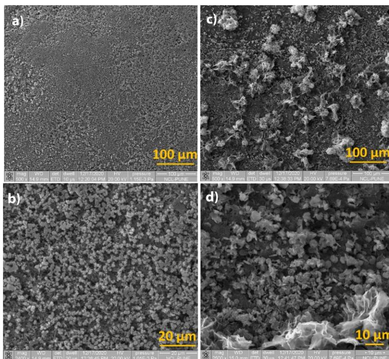
**Figure S7.** SEM image of NTCDA electrodes recovered from the NTCDA||Zn-(N) cell at the (a-b) discharged, and (c-d) charged states at different magnifications.
