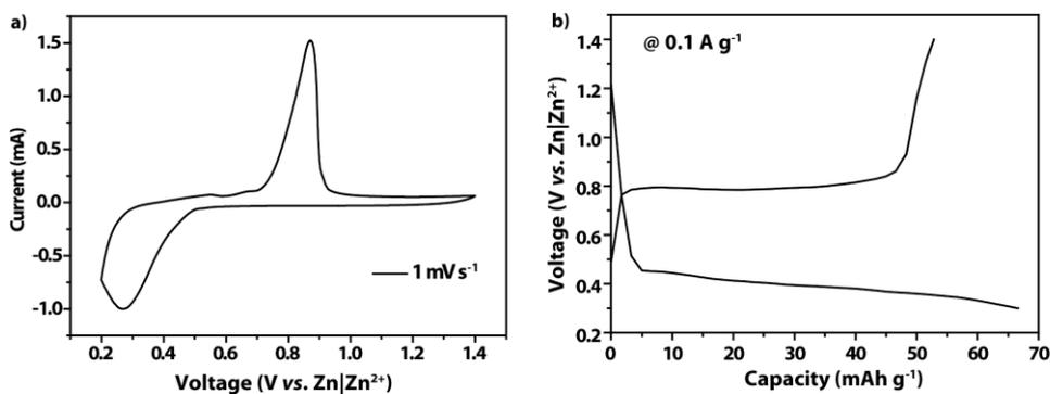
**Figure S3.** (a) CV profile recorded at the scan rate of  $1.0 \text{ mV s}^{-1}$  and (b) GCD profile recorded at the current rate of  $0.1 \text{ A g}^{-1}$  for the NTCDA||Zn-(O) cell in  $0.5 \text{ M ZnOTf/ACN}$  electrolyte.
