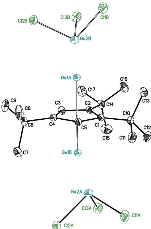
**Figure S15.** Full asymmetric unit for compound **8**. Hydrogen atoms are omitted for clarity. ADPs are depicted at 50% probability level. Atoms labelled with the indexes “A” and “B” belong to mutually exclusive disordered groups. The atoms belonging to the disorder were refined with restraints for the distances and ADPs. The ADPs of the chlorine atoms were fixed to identical values with their nearest neighbour. The occupancy of the minor component refined to 0.0161(4).
