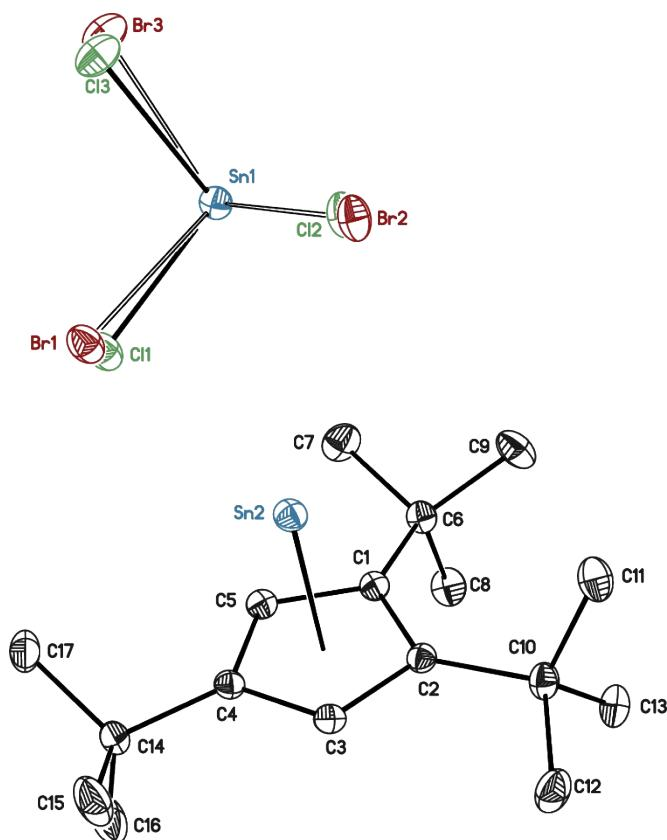
**Figure S17.** Full asymmetric unit for compound 9. Hydrogen atoms are omitted for clarity. ADPs are depicted at 50% probability level. Each chlorine atom is disordered with a small amount of bromine, the bromine from the impurities  $\text{SnBr}_2$  or  $\text{SnBr}_3\text{Cl}$  in the starting material  $\text{SnCl}_2$ . The Sn-Cl and the Sn-Br distances were refined with distance restraint, while the ADPs were fixed to equal values. The occupancies of the bromine atoms refined to 0.1014(14),
