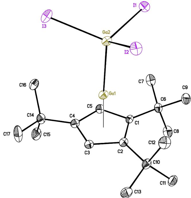
**Figure S13.** Full asymmetric unit for compound **6**. Hydrogen atoms are omitted for clarity
