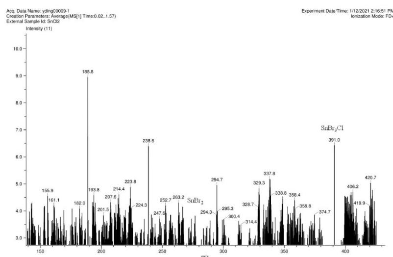
Figure S18. Mass spectra of the starting material SnCl<sub>2</sub>.
