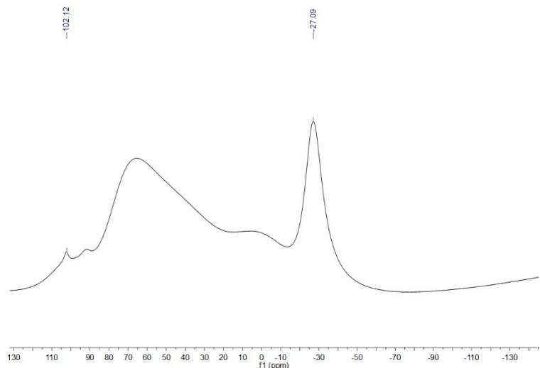
Figure S1.3  $^{27}\text{Al}$  NMR of compound 1 ( $\text{AlCl}_3$  peak at 102.12 ppm).
