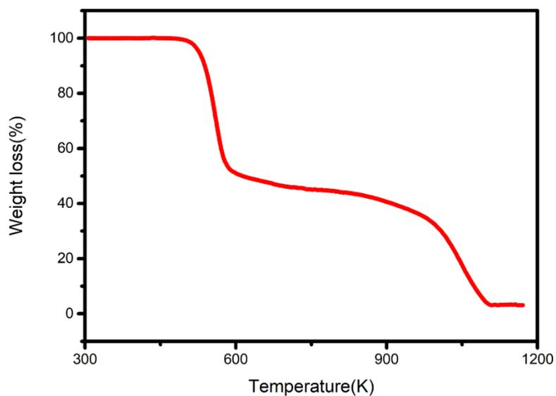
**Fig S3.** TGA curve of  $[FMPD][Cd(SCN)_3]$ .
