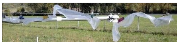
Figure.S.3: Different sampling set-ups in the field (Entringen): Left: Transparent and black PE sheets hanging within the aluminium box cover. Right: Black (top) and transparent (bottom) sheets hanging freely without protection from wind, sunlight etc..
