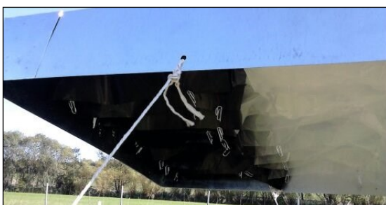
Figure.S.3: Different sampling set-ups in the field (Entringen): Left: Transparent and black PE sheets hanging within the aluminium box cover. Right: Black (top) and transparent (bottom) sheets hanging freely without protection from wind, sunlight etc..
