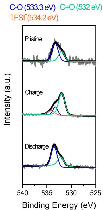
**Fig. S27** Ex-situ O 1s XPS spectra of 3PXZ electrodes in the pristine, charged, and discharged states.
