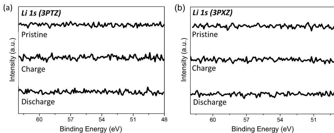
**Fig. S28** Li 1s spectra of ex-situ XPS measurements for (a) 3PTZ and (b) 3PXZ electrodes. No signals appeared for all ex-situ samples, which indicates Li ion-free redox reactions and complete removal of LiTFSI electrolyte by washing the ex-situ samples.
