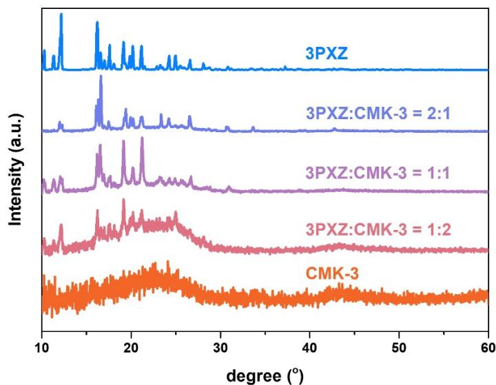
**Fig. S32** PXRD spectra of the pristine 3PXZ, 3PXZ@CMK-3 composites with different mixing ratio, and the pristine CMK-3. The slightly different PXRD peaks observed in the 2:1 sample is most likely attributed to the occurrence of fast recrystallization from the supersaturated solution leading to formation of somewhat different crystal structure of 3PXZ from the other samples.
