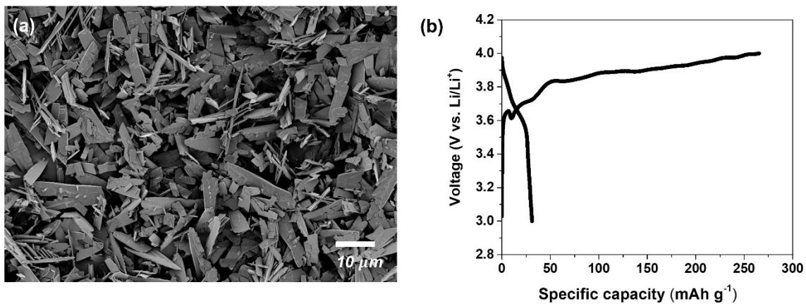
**Fig. S23** (a) SEM image of the downsized 3PTZ particles after the antisolvent precipitation process. (b) Galvanostatic charge/discharge profile (1<sup>st</sup> cycle) of the electrode fabricated with downsized 3PTZ at a current rate of 1 C.
