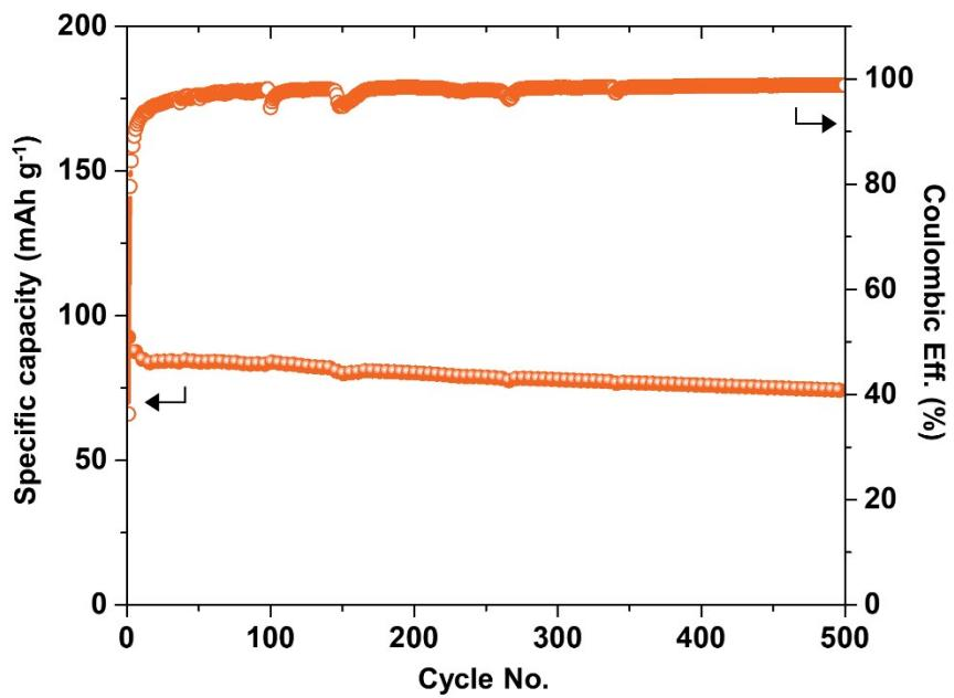
**Fig. S37** Specific capacities with the corresponding coulombic efficiencies obtained from cycling stability test of 3PXZ@CMK-3 electrode at 1C rate, after removing the capacity contribution of CMK-3.
