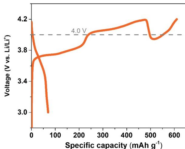
**Fig. S21** The galvanostatic charge/discharge profile of 3PXZ in voltage range 3.0 V – 4.2 V at current rate of 1C.
