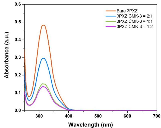
**Fig. S34** UV-vis absorption spectroscopic investigations after 24 h immersion of the electrodes in the excessive amount of electrolyte. A 3 mL of 2 M LiTFSI in DOL/DME (1:1 v/v) electrolyte was used per 1 mg of 3PXZ in the electrode. After 24 h immersion, the solutions were diluted ten times for measuring absorbance.
