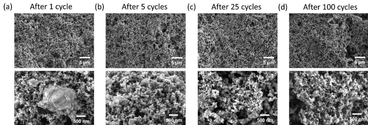
**Fig. S24** SEM images of the surface of 3PXZ electrodes after (a) 1 (b) 5 (c) 25 (d) 100 charge/discharge cycle(s).
