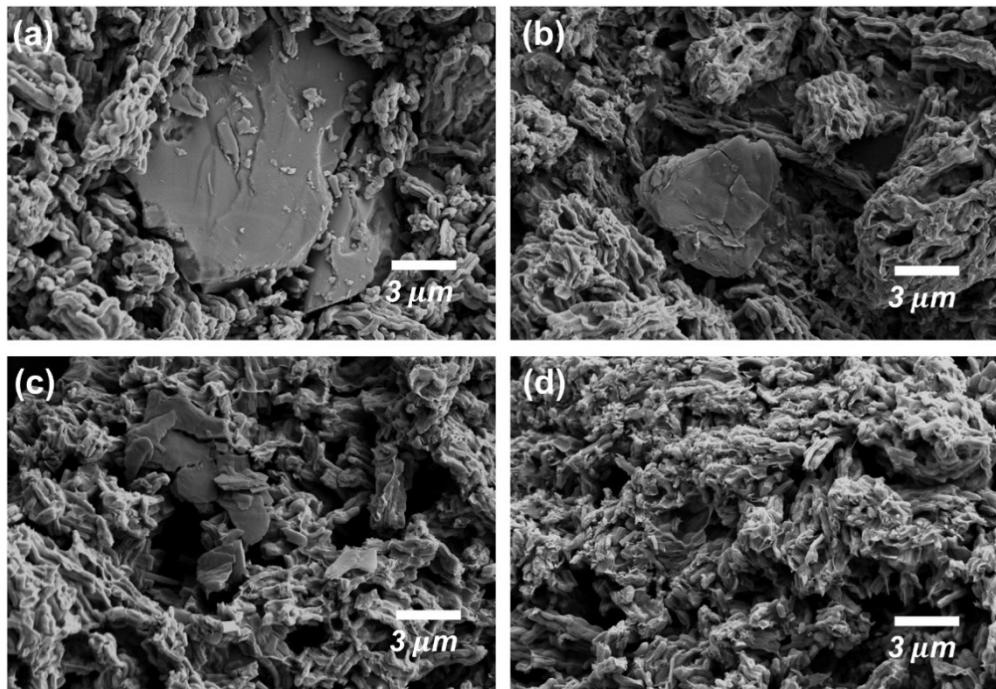
**Fig. S33** SEM images of 3PXZ@CMK-3 composites with different mixing ratio: 3PXZ: CMK-3 was (a) 2:1, (b) 1:1, and (c) 1:2 in weight. (d) An SEM image of the pristine CMK-3.
