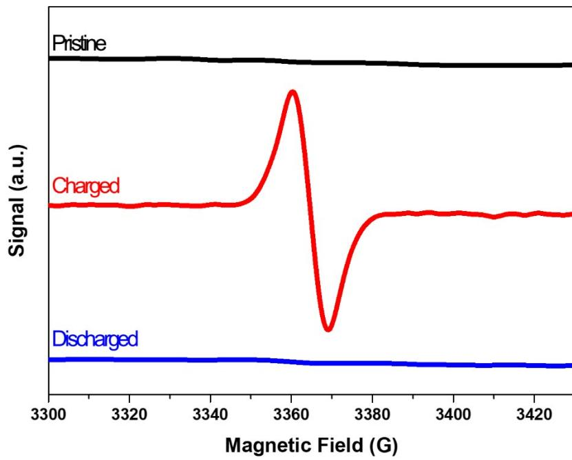
**Fig. S30** Ex-situ electron spin resonance (ESR) spectroscopy measurements of 3PXZ electrodes. Only charged electrode showed ESR signal with  $g = 2.0030$ , which indicates formation of radical cations after oxidation.
