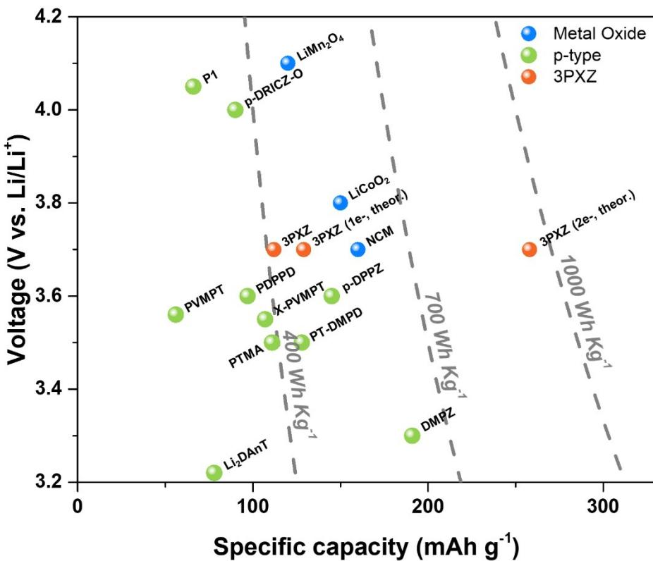
**Fig. S38** Specific capacity *vs.* voltage plot of the previously reported p-type organic electrode materials, conventional inorganic materials, 3PXZ and theoretical two-electron storage specific capacity of 3PXZ. See Table S2 (ESI<sup>†</sup>) for detailed information on the reported materials used in this plot.
