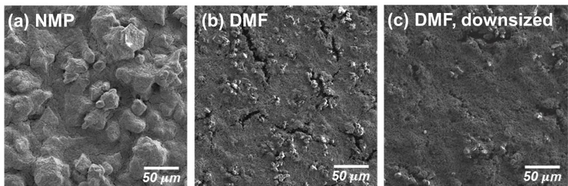
**Fig. S20** SEM images of 3PXZ electrodes prepared by various conditions: (a) NMP and (b) DMF was used as the slurry-making solvent. (c) DMF was used as the slurry-making solvent, and the downsized particle of 3PXZ by the antisolvent precipitation process was used.
