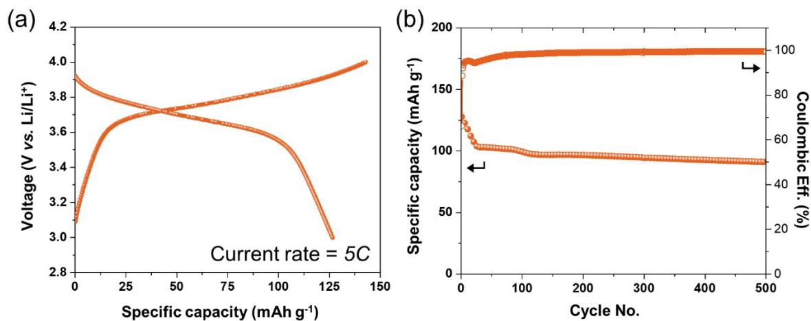
**Fig. S36** (a) Representative galvanostatic charge/discharge profiles and (b) specific capacity with the corresponding coulombic efficiency obtained from the cycling stability test of 3PXZ@CMK-3 electrode at 5C, before removing the capacity contribution of CMK-3 in the composite.
