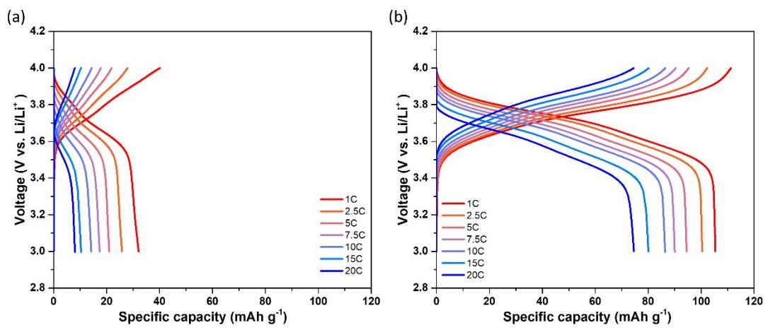
**Fig. S26** Electrochemical profiles of (a) 3PTZ and (b) 3PXZ, under different C-rates.
