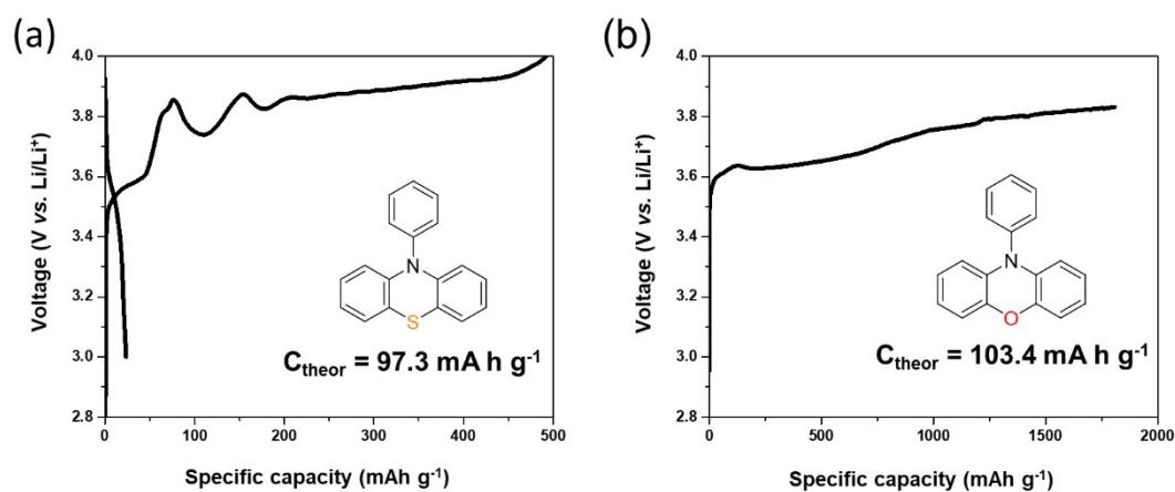
**Fig. S13** The charge/discharge profiles of the first cycle for (a) PhPTZ and (b) PhPXZ electrode at 1 C rate. 2 M LiTFSI with 1 wt% LiNO<sub>3</sub> in DOL/DME (1:1 v/v) was used as an electrolyte. The C rate of each material was calculated by its theoretical capacity, which corresponds to 97.3 mA g<sup>-1</sup> and 103.4 mA g<sup>-1</sup> for PhPTZ and PhPXZ, respectively.
