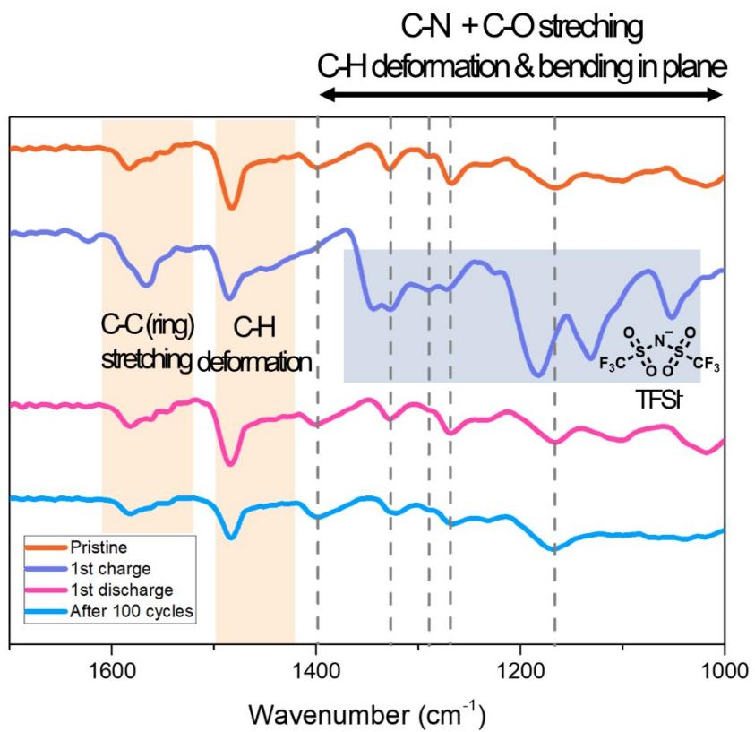
**Fig. S29** FT-IR measurements of 3PXZ ex-situ electrodes.
