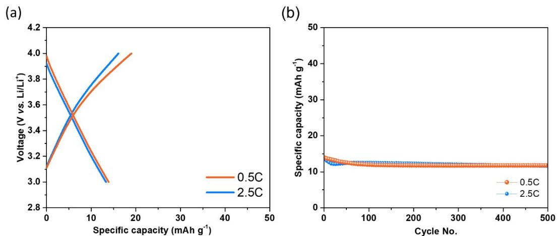
**Fig. S35** (a) The charge/discharge profiles and (b) cycle data at 0.5C and 2.5C rate of the genuine CMK-3 electrode (80 wt% of CMK-3, 10 wt% of carbon black, and 10% of PVDF). Given that the weight ratio of 3PXZ:CMK-3 is 1:2 in the 3PXZ@CMK-3 composite, we evaluated the genuine CMK-3 electrode at 0.5C and 2.5C.
