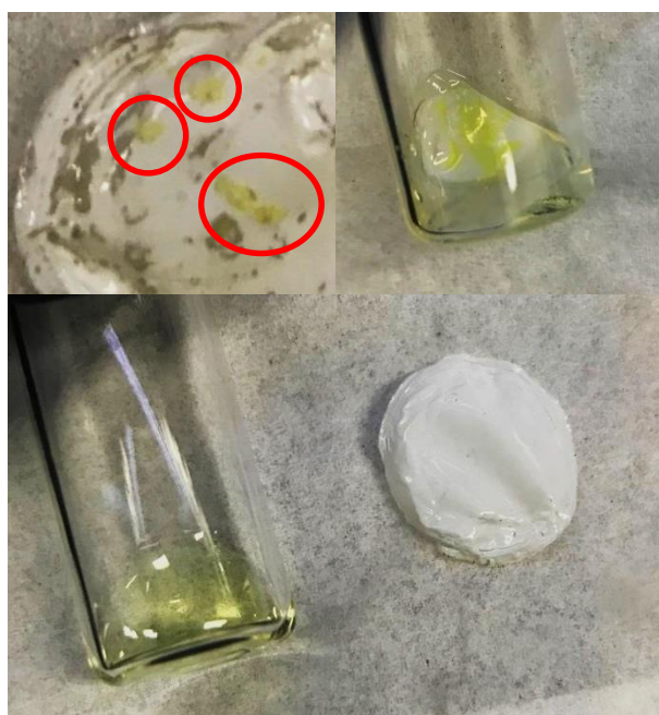
Figure S33. Dissolution of solid magnesium (poly)sulfide species via reaction with derivatizer. Upper left, separator with deposits circled. Top right, separator in solution of derivatizing agent + DME. Bottom, dried separator after removing from solution and yellow derivatized polysulfides.
