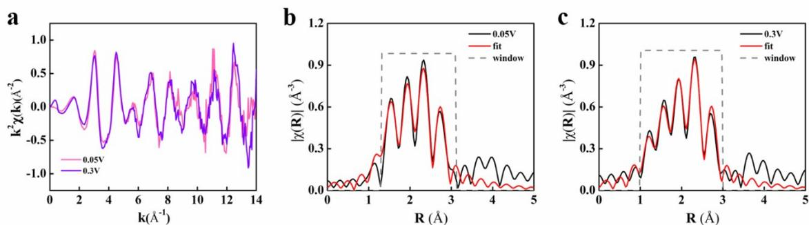
**Figure S9.** The *in situ* FT-EXAFS spectra at the Ru K-edge of the Pt<sub>1</sub>Ru<sub>1</sub>/C at both the k (**a**) and R (**b-c**) spaces, together with the corresponding EXAFS fitting.
