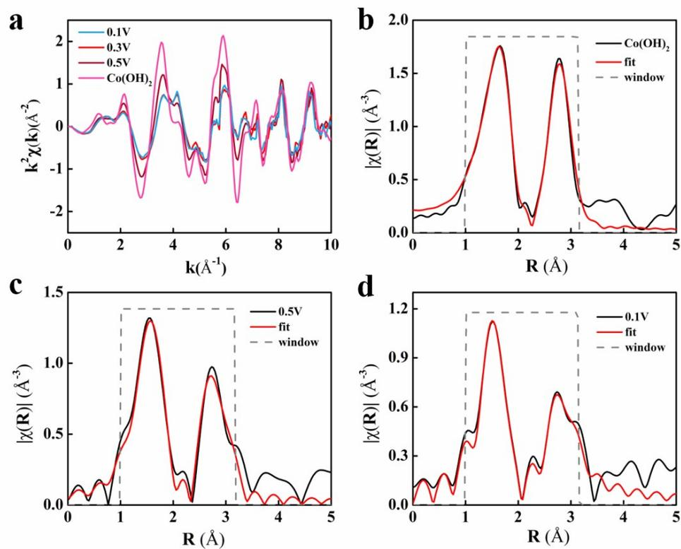
**Figure S5.** The *in situ* EXAFS spectra at the Co K-edge of Co@Pt and  $\text{Co(OH)}_2$  at both the  $k$  (a) and  $R$  (b-d) spaces, together with the corresponding EXAFS fitting.
