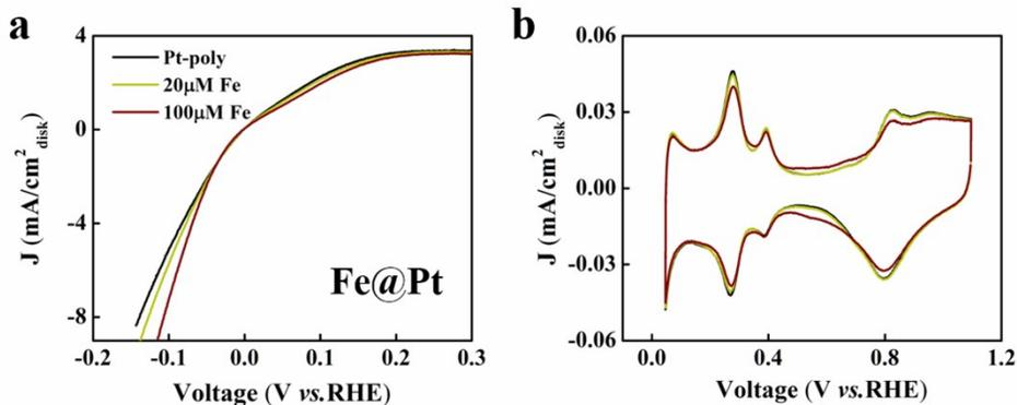
**Figure S1.** (a) *IR*-corrected HOR/HER polarization curves collected at room temperature in an  $\text{H}_2$ -saturated 0.1 M KOH electrolyte on the Pt polycrystalline electrode with  $\text{Fe}^{3+}$ . Scan rate:  $10 \text{ mV}\cdot\text{s}^{-1}$ . Rotation rate: 2,500 rpm. (b) The *CV* collected at room temperature in an Ar-saturated 0.1 M KOH electrolyte on the Pt polycrystalline electrode with varied concentrations of  $\text{Fe}^{3+}$ . Scan rate:  $20 \text{ mV}\cdot\text{s}^{-1}$ .
