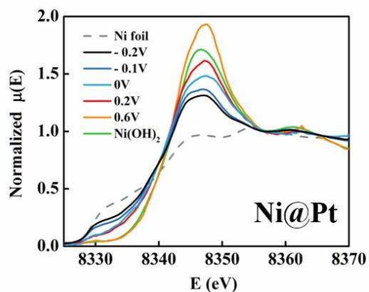
**Figure S3.** The K-edge XANES spectra of the Ni@Pt as a function of applied potentials collected in an H<sub>2</sub>-purged 0.1 M KOH electrolyte. Some of the data were obtained from our previous work (Ref 15).
