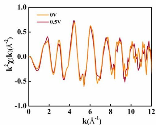
**Figure S6.** The *in situ* FT-EXAFS spectra at the Cu K-edge of Cu@Pt at the  $k$  space.
