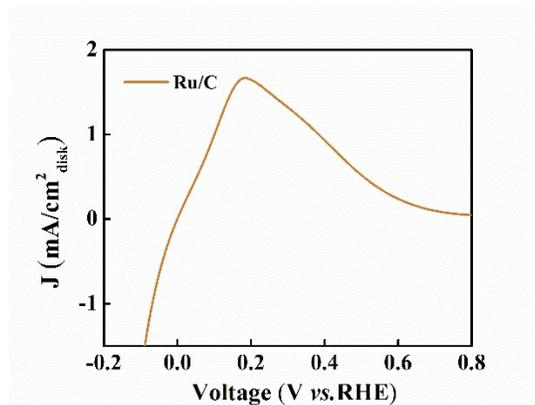
**Figure S12.** The *iR*-corrected HOR/HER polarization curves collected at room temperature in an H<sub>2</sub>-saturated 0.1 M KOH electrolyte of Ru/C. Scan rate: 10 mV·s<sup>-1</sup>. Rotation rate: 2,500 rpm.
