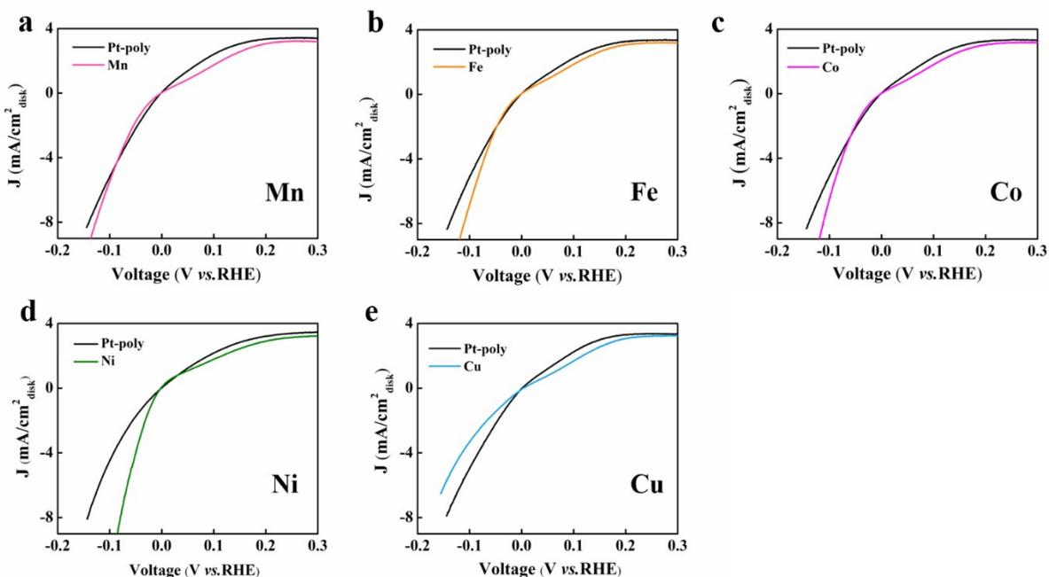
**Figure S13.** The iR-corrected HOR/HER polarization curves collected at room temperature in an  $\text{H}_2$ -saturated 0.1 M KOH electrolyte on the Pt polycrystalline electrode with  $\text{Mn}^{2+}$  (a),  $\text{Fe}^{3+}$  (b),  $\text{Co}^{2+}$  (c),  $\text{Ni}^{2+}$  (d) and  $\text{Cu}^{2+}$  (e). TM coverage is 30% ~ 40%. Scan rate:  $10 \text{ mV} \cdot \text{s}^{-1}$ . Rotation rate: 2,500 rpm.
