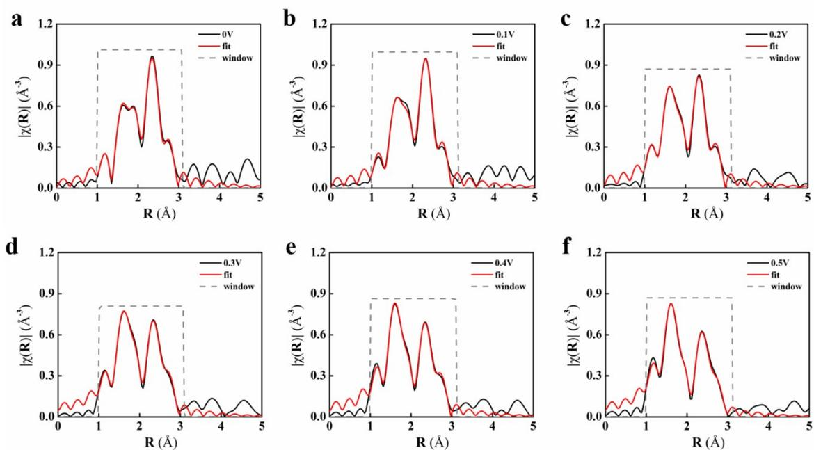
**Figure S8.** The *in situ* FT-EXAFS spectra at the Ru K-edge of Ru@Pt within 0 – 0.5 V, together with the corresponding EXAFS fittings.
