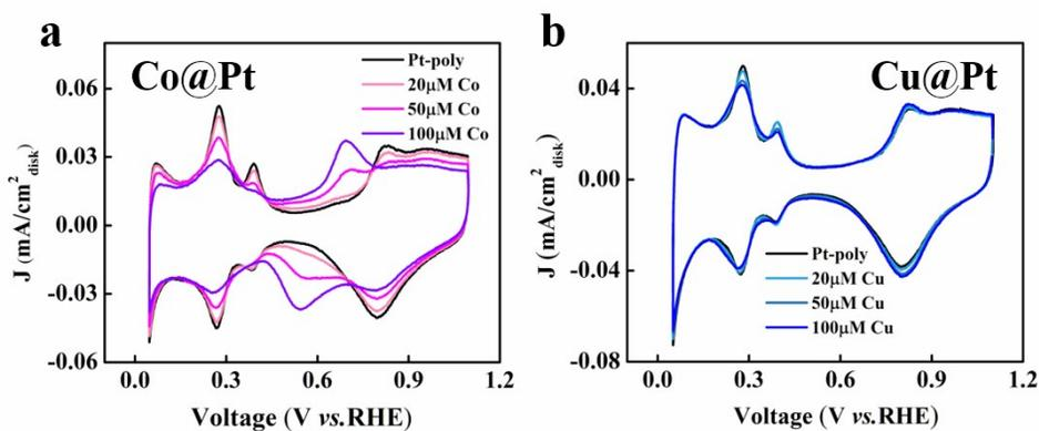
**Figure S2.** The *CV* collected at room temperature in an Ar-saturated 0.1 M KOH electrolyte on the Pt polycrystalline electrode with varied concentrations of  $\text{Co}^{2+}$  (a) and  $\text{Cu}^{2+}$  (b). Scan rate:  $20 \text{ mV}\cdot\text{s}^{-1}$ .
