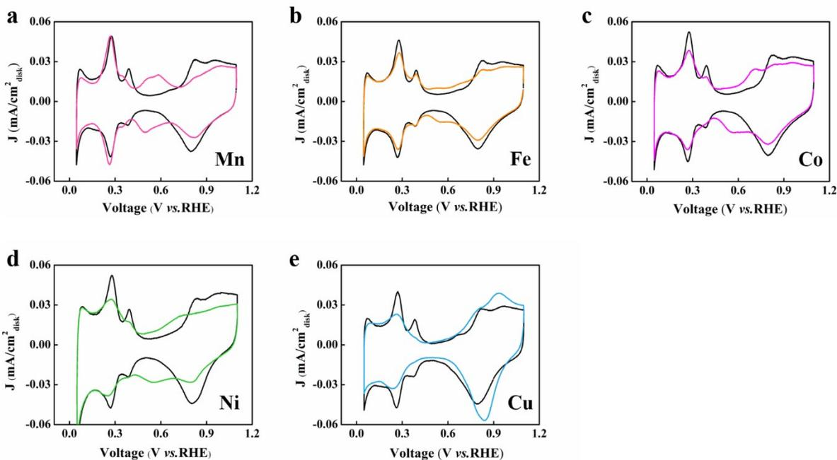
**Figure S14.** The CVs collected at room temperature in an Ar-saturated 0.1 M KOH electrolyte on the Pt polycrystalline electrode with  $\text{Mn}^{2+}$  (a),  $\text{Fe}^{3+}$  (b),  $\text{Co}^{2+}$  (c),  $\text{Ni}^{2+}$  (d) and  $\text{Cu}^{2+}$  (e). TM coverage is 30% ~ 40%. Scan rate:  $20 \text{ mV} \cdot \text{s}^{-1}$ .
