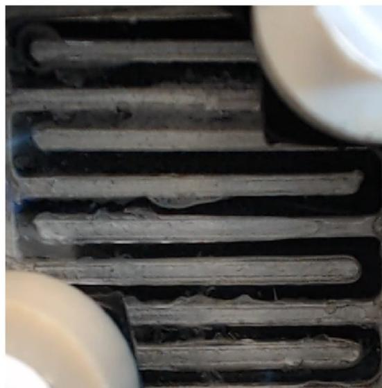
**Figure S17:** Images of precipitation in flow field channels with an applied current density of 200 mA cm<sup>-2</sup> with a wet feed (left) and 100 mA cm<sup>-2</sup> with a dry feed (right). Excess glue from assembly can be observed near the left and right edges of the flow field in both photos. Photos are high resolution versions of the thumbnail images in Figure 4.
