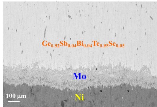
Fig. S8 Microstructure of the \text{Ge}_{0.92}\text{Sb}_{0.04}\text{Bi}_{0.04}\text{Te}_{0.95}\text{Se}_{0.05}/\text{Mo}/\text{Ni} interface.
