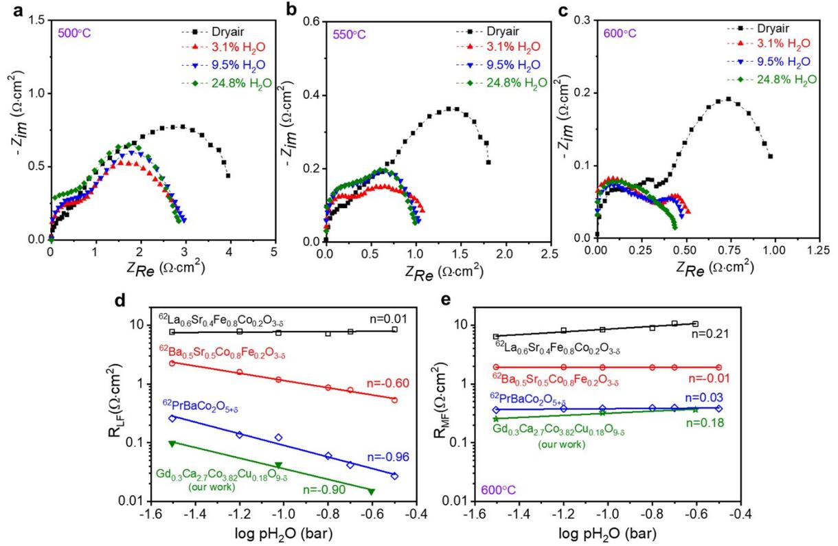
**Fig. S11** EIS spectra and polarization resistance ( $R_p$ ) for GCCCO under different  $p\text{H}_2\text{O}$  conditions. (a-c) EIS spectra for GCCCO at 500°C (a), 550°C (b), and 600°C (c). (d-e)  $p\text{H}_2\text{O}$  dependences of  $R_p$  of various oxygen electrodes at 600°C in low frequency (LF) (d) and middle frequency (MF) ranges (e).
