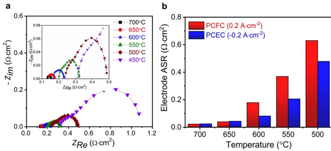
**Fig. S6** EIS spectra and comparison of electrode ASR of an anode-supported GCCCO cell under PCFC and PCEC modes. (a) EIS in PCFC mode under OCV condition at 450–700°C. (b) Electrode ASRs for PCFC and PCEC mode at 0.2 A·cm<sup>-2</sup> and -0.2 A·cm<sup>-2</sup> conditions.
