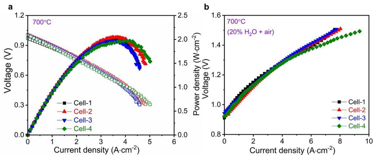
**Fig. S5** Reproducibility of NiO-BCZYYb anode-supported cells with a composite GCCCO-BCZYYb air electrode. (a-b) Cell voltage as functions of current density in multiple tests at 700°C under PCFC (a) and PCEC modes (b).
