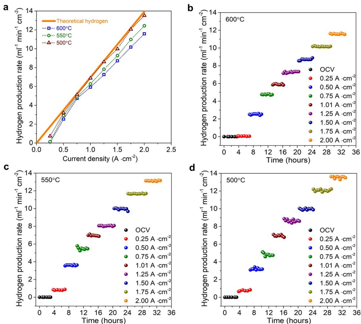
**Fig. S7** Hydrogen production rate of GCCCO cell as a function of current density at 500–600°C. (a) Hydrogen production rate as a function of current density at 500–600°C. (b-d) Hydrogen production rate as a function of time under various current density at 600 (b), 550 (c), and 500°C (d).
