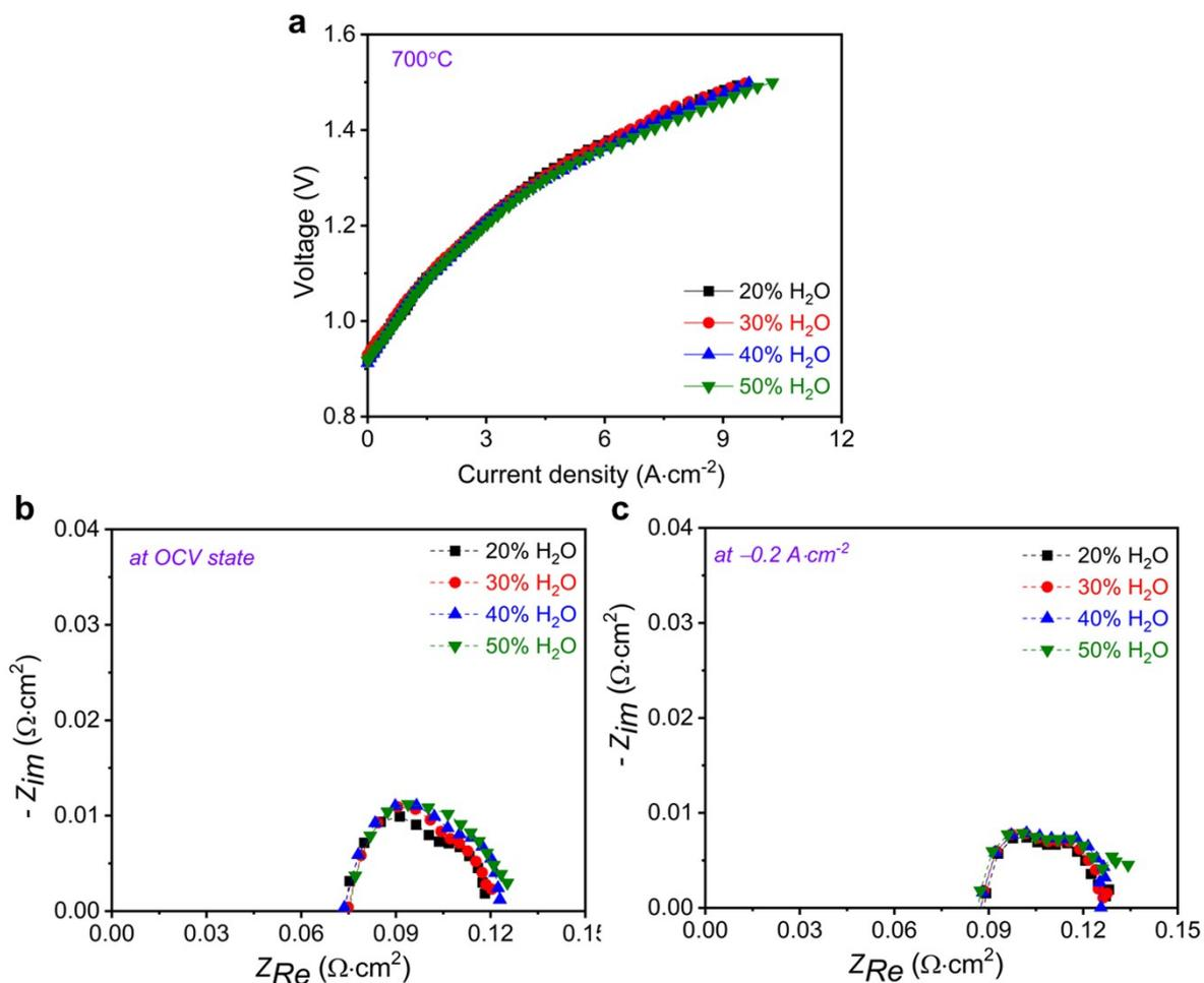
**Fig. S8** Electrochemical performances of the RPCC in PCEC mode under various steam concentrations (20–50% H<sub>2</sub>O in ambient air) at 700 °C. (a) I-V curves of a GCCCO cell. (b) EIS in PCEC mode under OCV condition. (c) EIS in PCEC mode under  $-0.2 \text{ A}\cdot\text{cm}^{-2}$  condition.
