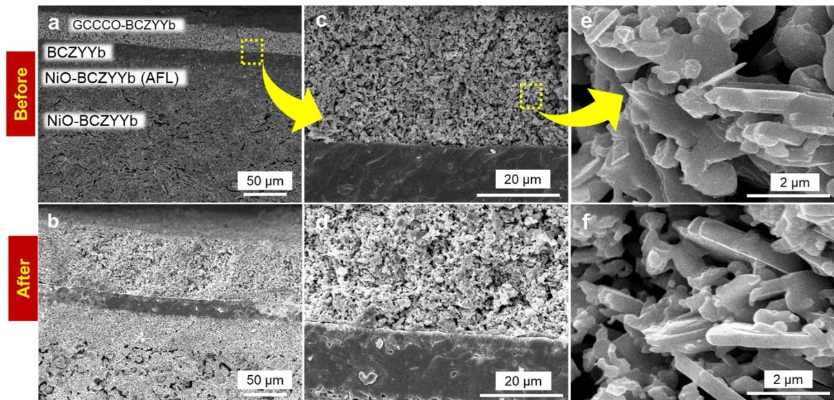
**Fig. S4** Microstructural analyses of NiO-BCZYYb-supported cell with BCZYYb electrolyte and GCCCO-BCZYYb composite air/steam electrode by using FESEM. (a-b) Cross-sectional view of the as-prepared NiO-BCZYYb single cell (a) and after durability tests (b). (c-d) Interfacial region between air electrode and electrolyte before (c) and after durability tests (d). (e-f) GCCCO-BCZYYb composite air (steam) electrode before (e) and after durability tests (f).
