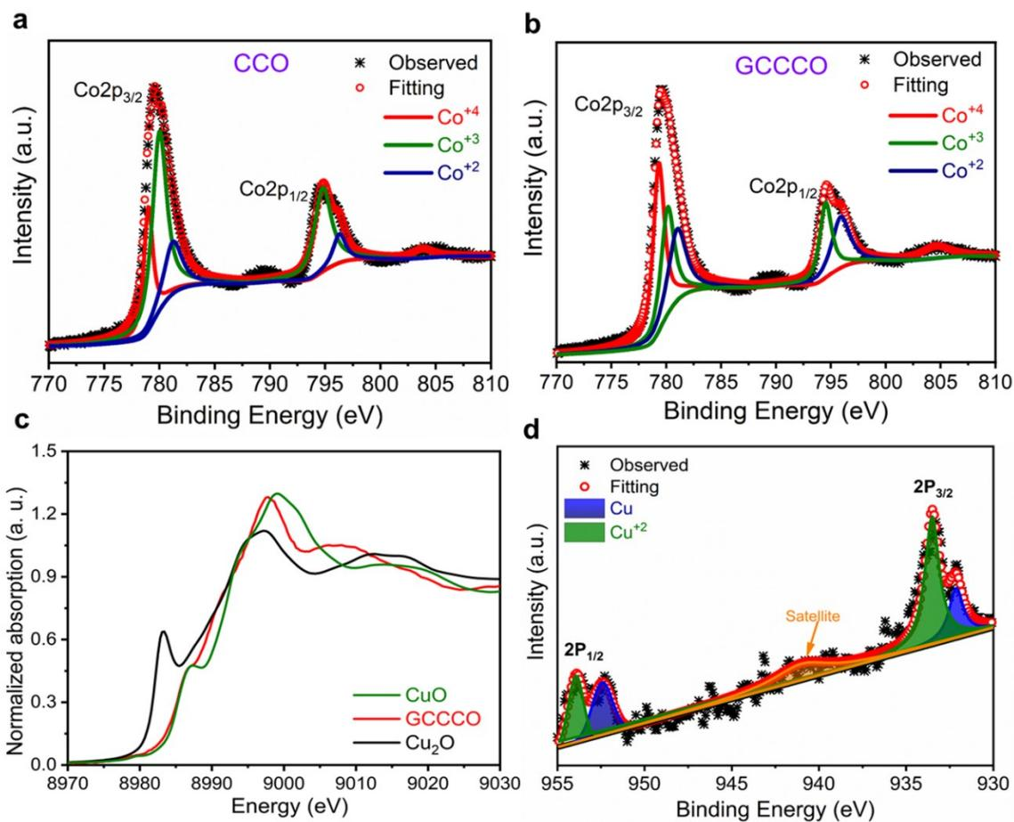
**Fig. S9** XPS and X-ray absorption near edge structure (XANES) survey spectra of GCCCO materials. (a-b) Deconvoluted Co 2p XPS spectra for CCO (a) and GCCCO (b) materials. (c) Cu K-edge XANES spectra of GCCCO and Cu references (CuO and Cu<sub>2</sub>O). (d) Deconvoluted Cu 2p XPS peaks for GCCCO.
