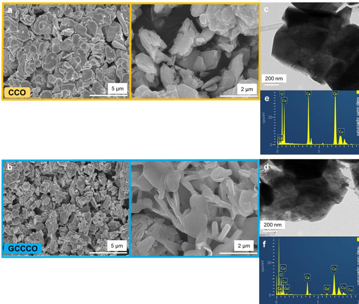
**Fig. S2** Morphology characterization and elemental analyses of CCO and GCCCO. (a-b) FESEM images of CCO (a) and GCCCO (b). (c-d) HRTEM images of CCO (c) and GCCCO (d). (e-f) EDX spectra of each element in CCO (e) and GCCCO (f).
