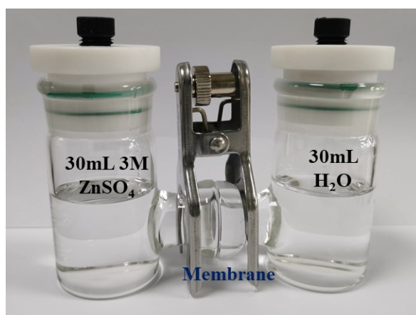
Figure S19. Test device for ZnSO 4 permeability.
