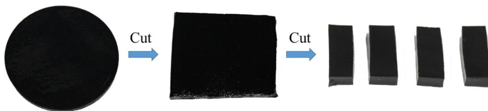
**Figure S4.** The integrated device units of different shapes prepared by simple cutting technology.
