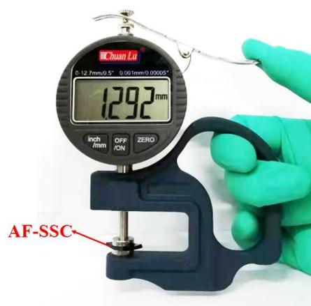
**Figure S2.** The minimum thickness (~1.3 mm) of AF-SSC.
