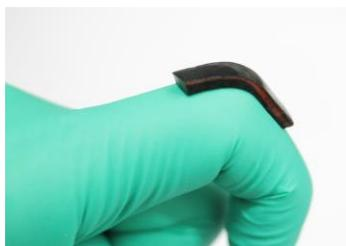
**Figure S8.** AF-SSC stably adhering to the surface of rubber gloves substrates without the extra adhesives even at the bending and stretching conditions.
