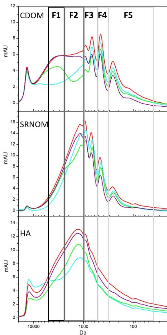
Figure S2: Division of DOM molecular weight into 5 fractions according to preferential adsorption by biochar (— blue line), graphite (— green line), and carbon nanotubes (— purple line). Each sorbent preferentially sorbed distinct molecular weight fractions of the DOM, which were then categorized as fractions 1 – 5 (F1-F5). Each fraction was collected and further characterized.
