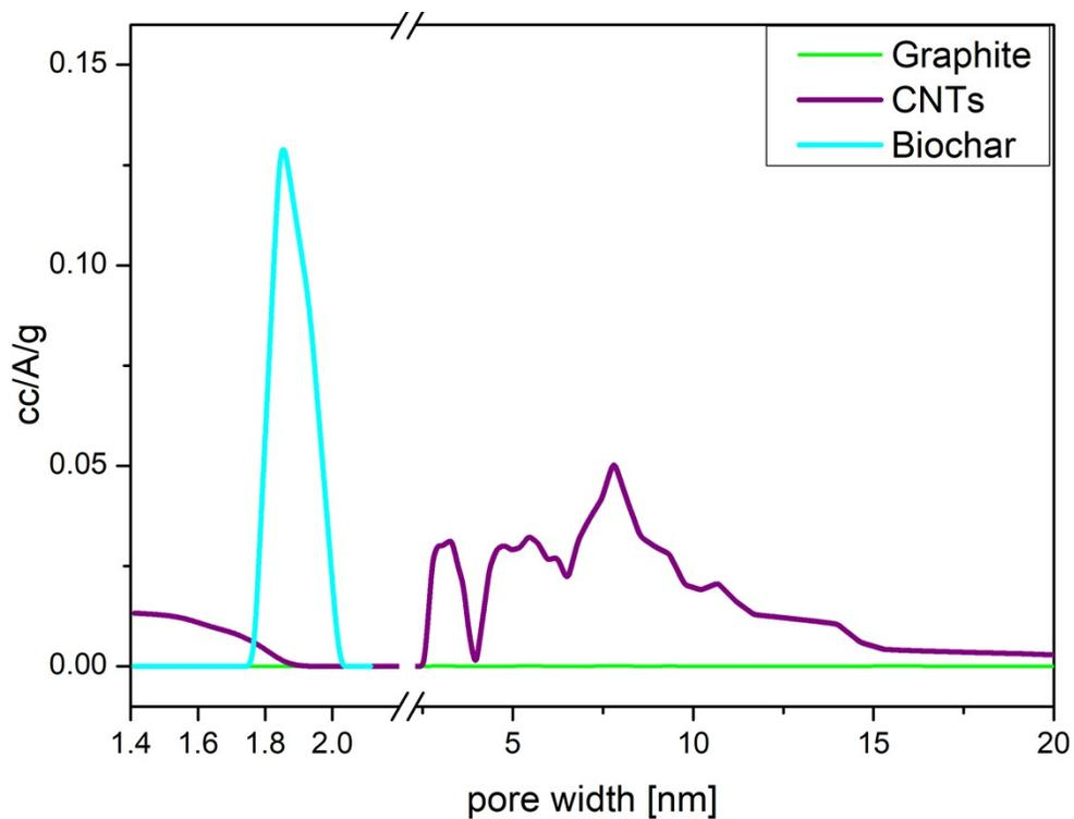
Figure S5. N<sub>2</sub> pore size distribution of biochar (— blue line), graphite (— green line), and carbon nanotubes (— purple line).
