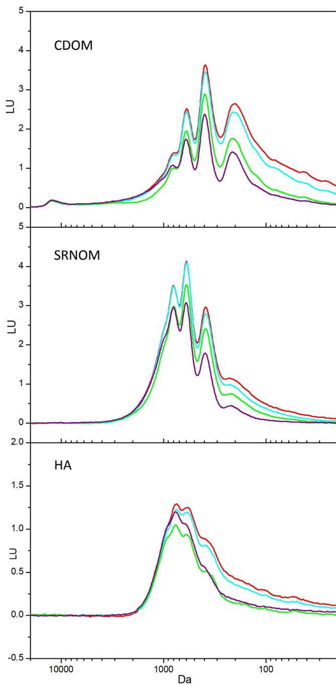
Figure S3. SEC chromatograms of CDOM, SRNOM and HA, detected by fluorescence (excitation wavelength 350 nm, emission wavelength 450 nm) prior to sorption (— red line), and after sorption to biochar (— blue line), graphite (— green line), and carbon nanotubes (— purple line).
