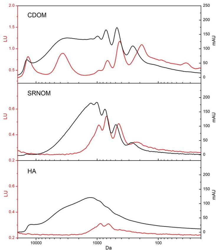
Figure S6. SEC chromatograms of CDOM, SRNOM and HA, detected by fluorescence at an excitation wavelength of 270 nm and an emission wavelength of 350 nm (— red line), and by UV at a wavelength of 254 nm (— black line). The peak in the molecular weight fractions  $> 2.5$  kDa and  $< 4$  kDa in CDOM indicates the presence of protein-like and tryptophan-like compounds in this molecular weight fraction, which also applies for the smaller fraction  $< 1$  kDa.
