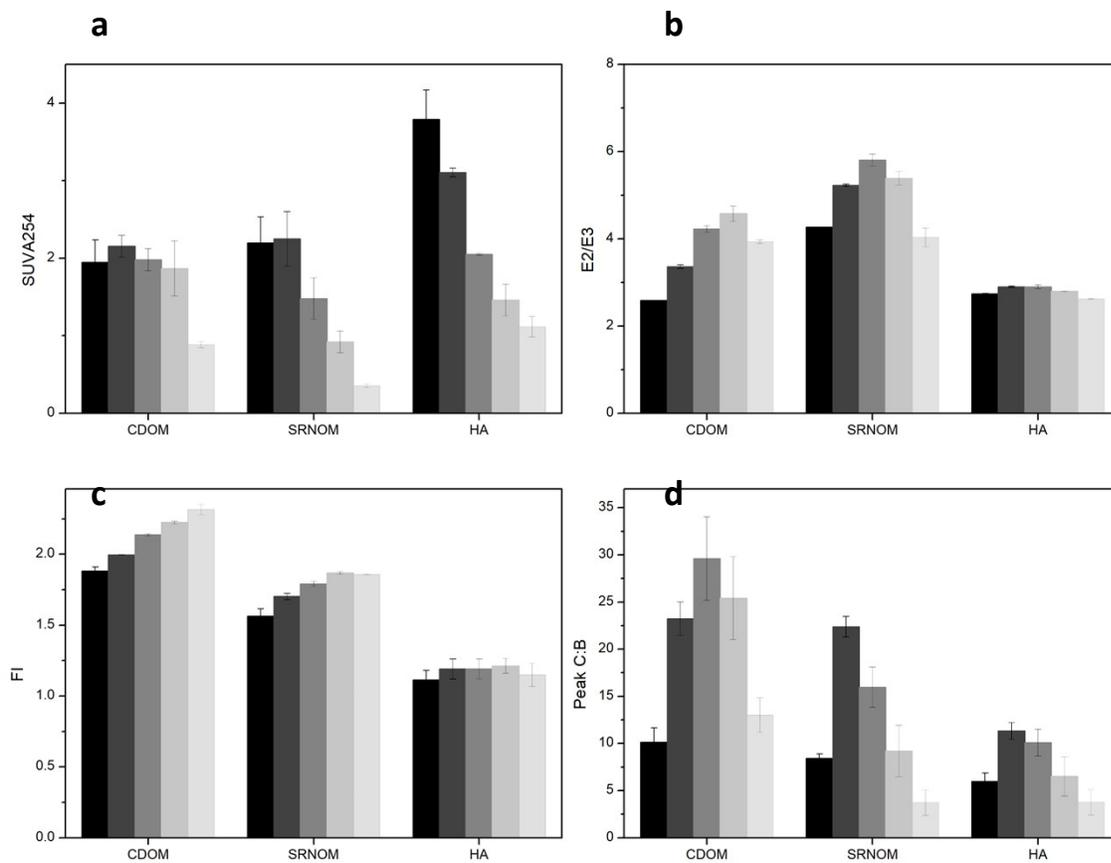
Figure S4. a) SUVA<sub>254</sub> value, b) E<sub>2</sub>/E<sub>3</sub> ratio, c) FI value, and d) Peak C:B ratio of CDOM, SRNOM and HA divided into five molecular weight fractions: 5 – 2.5 kDa (—), 2.5 – 1 kDa (—), 1 – 0.5 kDa (—), 0.5 – 0.3 kDa (—), and 0.3 – 0.03 kDa (—). The error bars represent the standard deviation from duplicate measurements.
