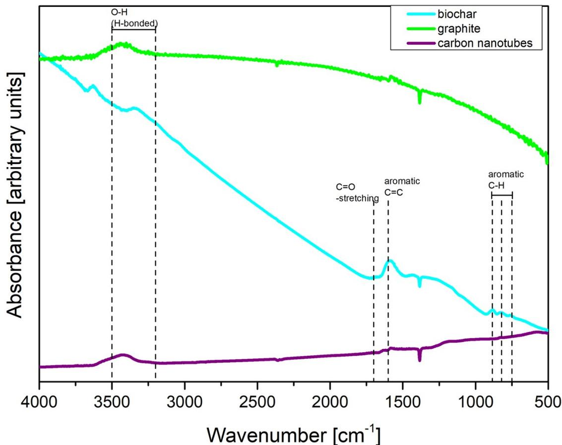
Figure S1. Fourier transform infrared (FT-IR) spectra for biochar (— blue line), graphite (— green line), and carbon nanotubes (— purple line). Spectra were recorded on a Bruker Tensor 27. CMs were embedded in KBr pellets, peak assignments according to Keiluweit et al. (2010).<sup>1</sup>
