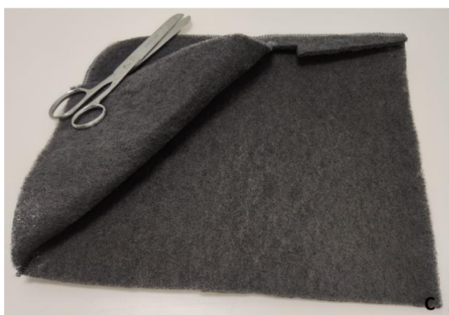
Figure S1: Photos of parts of the filters A, B and C after half year exposure in HVAC system.
