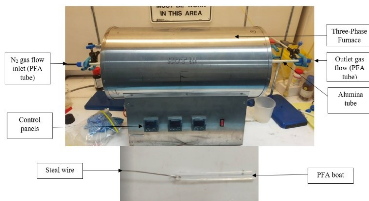
Figure S1. The main features of the apparatus three-zone furnace and boat.
