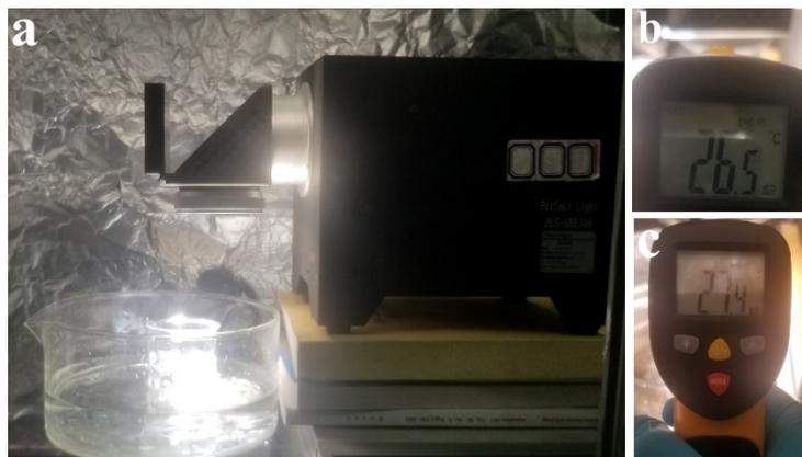
Fig. S5 Photos of the reaction system surrounded by cold water (a), the temperatures of the solution surface before (b) and after (c) the photocatalytic reaction.
