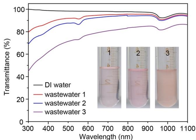
**Fig. S1** Transmittance of light in deionized (DI) water and simulated wastewater. (Inset) photos of simulated wastewater 1-3. Wastewater 1: 0.6 g/L soil + 2 ppm RhB + 2 ppm TC + 2 ppm BPA, wastewater 2: 0.8 g/L soil + 5 ppm RhB + 5 ppm TC + 5 ppm BPA, wastewater 3: 1.5 g/L soil + 5 ppm RhB + 5 ppm TC + 10 ppm BPA.
