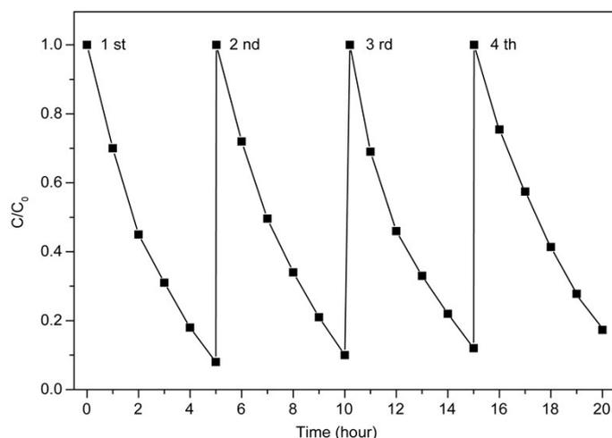
**Fig. S21** The reusability of NGFCS@TiO<sub>2</sub> for photocatalytic degradation of RhB under NIR light irradiation.
