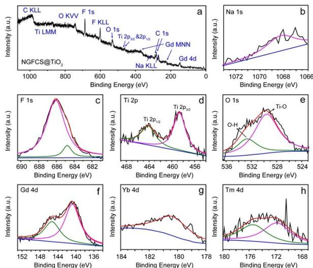
**Fig. S5** (a) Wide XPS spectra for the NGFCS@TiO<sub>2</sub> nanocomposites, (b)-(g) High-resolution XPS spectra of Na 1s, F 1s, Ti 2p, O 1s, Gd 4d, Yb 4d and Tm 4d, respectively.
