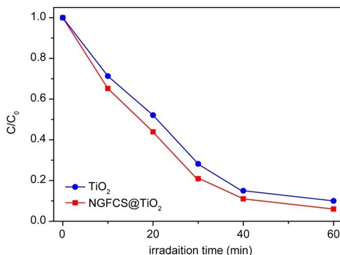
**Fig. S22** RhB photodegradation efficiency with the presence of NGFCS@TiO<sub>2</sub> and pure TiO<sub>2</sub> under simulated sunlight irradiation (100 mW/cm<sup>2</sup>).
