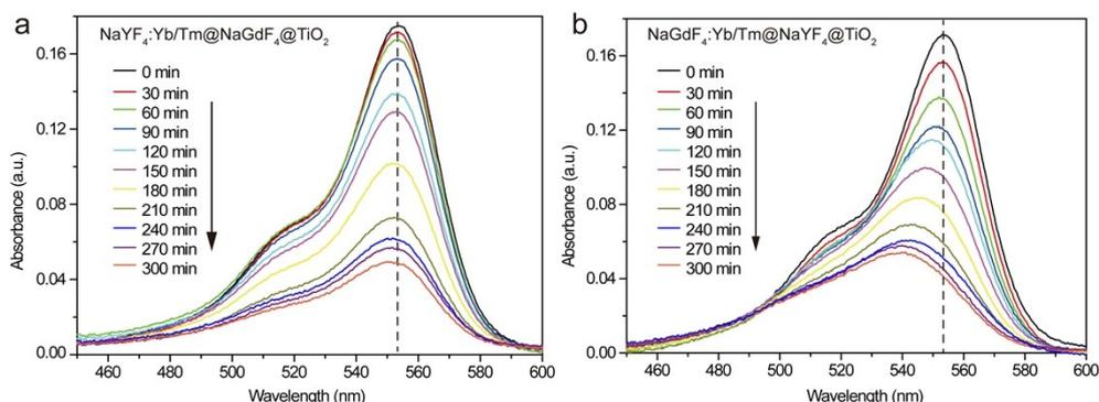
**Fig. S15** Change of absorption spectra of RhB in aqueous solution (20 ppm) with reaction time, with the addition of (a) NYF/NGF@TiO<sub>2</sub>, (b) NGF/NYF@TiO<sub>2</sub> under 980 nm excitation with a power density of 2.5 W/cm<sup>2</sup>, respectively.
