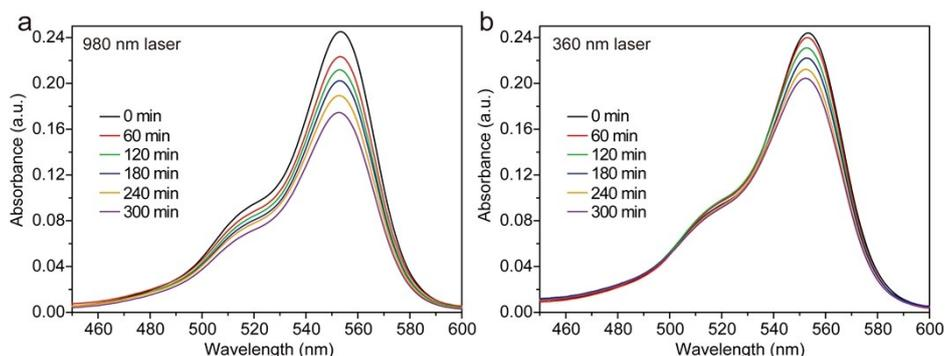
**Fig. S19** Absorption spectra of RhB in aqueous solution (20 ppm) with reaction time, with the addition of NGFCS@TiO<sub>2</sub> under (a) 980 nm excitation (48 mW/cm<sup>2</sup>) and (b) 360 nm excitation (44 mW/cm<sup>2</sup>). The real wastewater was a barrier between the light source and RhB solution.
