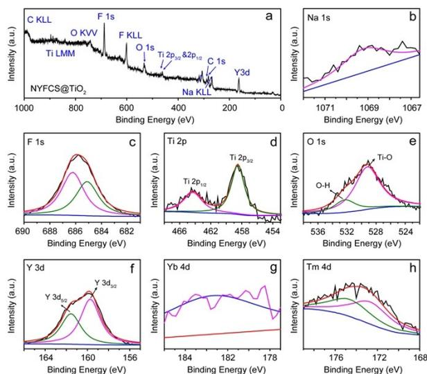
**Fig.S6** (a) Wide XPS spectra for the NYFCS@TiO<sub>2</sub> nanocomposites, (b)-(g) High-resolution XPS spectra of Na 1s, F 1s, Ti 2p, O 1s, Y 3d, Yb 4d and Tm 4d, respectively.
