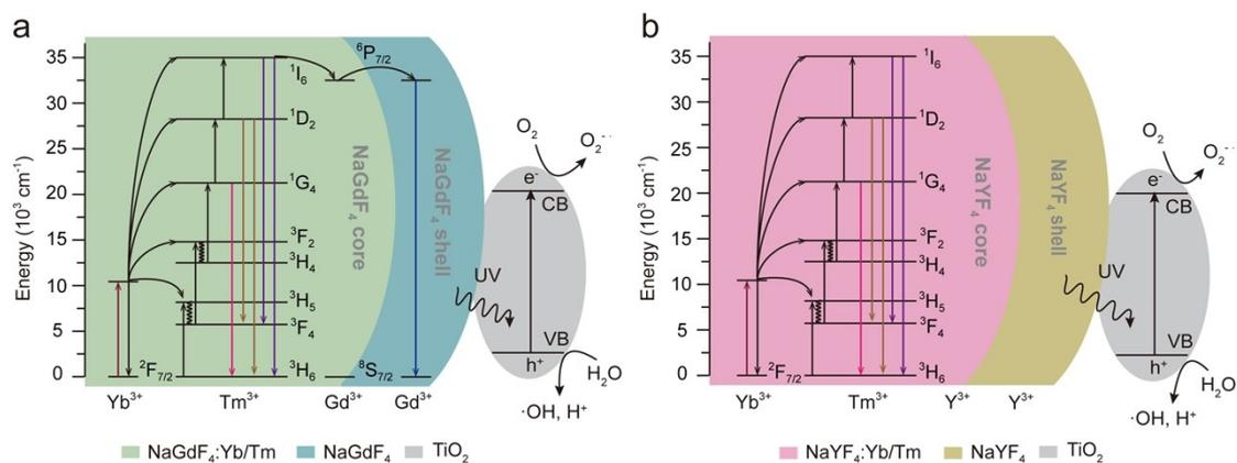
**Fig. S10** Energy transfer processes involved in (a) NGFCS@TiO<sub>2</sub> and (b) NYFCS@TiO<sub>2</sub> nanocomposites.
