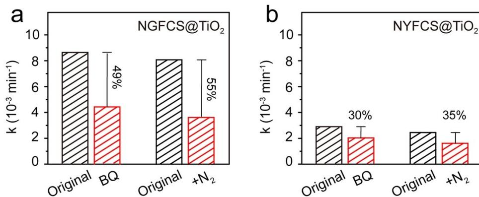
**Fig. S14.** RhB photodegradation efficiency comparison of different situations, with BQ trapping agent and purging of N<sub>2</sub> gas respectively, under 980 nm light excitation with (a) NGFCS@TiO<sub>2</sub> and (b) NYFCS@TiO<sub>2</sub> photocatalysts.
