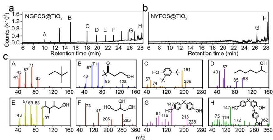
**Fig. S18** (a), (b) The respective gas chromatograms patterns for the intermediate products of BPA catalyzed by NGFCS@TiO<sub>2</sub> and NYFCS@TiO<sub>2</sub>, after 300 minutes under 980-nm light irradiation. (c) The corresponding ESI mass spectra of the intermediates detected in (a) and (b).
