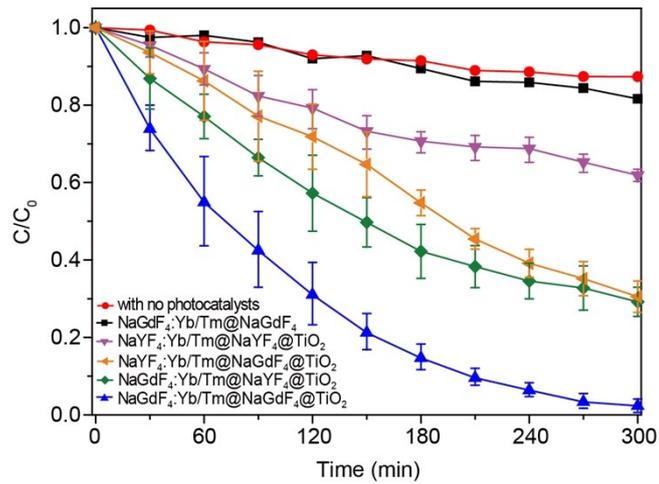
**Fig. S12** Degradation of RhB in aqueous solution (20 ppm) with reaction time, in the absence and presence of NGFCS@TiO<sub>2</sub>, NYFCS@TiO<sub>2</sub>, NYF/NGF@TiO<sub>2</sub>, NGF/NYF@TiO<sub>2</sub> and NGFCS under 980 nm excitation with a power density of 2.5 W/cm<sup>2</sup>, respectively.
