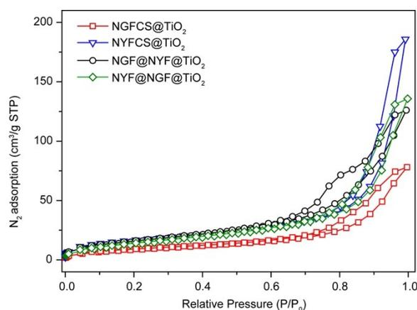
**Fig. S9** N<sub>2</sub> adsorption–desorption isotherms of different samples.
