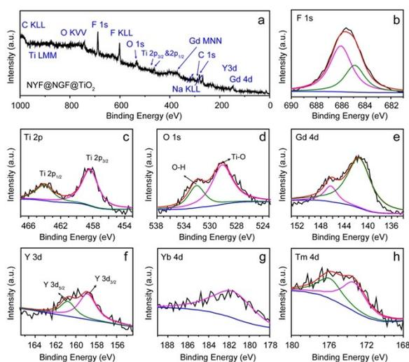
**Fig. S8** (a) Wide XPS spectra for the NYF@NGF@TiO<sub>2</sub> nanocomposites, (b)-(g) High-resolution XPS spectra of F 1s, Ti 2p, O 1s, Gd 4d, Y 3d, Yb 4d and Tm 4d, respectively.
