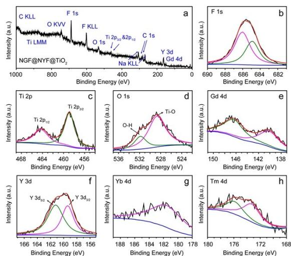
**Fig. S7** (a) Wide XPS spectra for the NGF@NYF@TiO<sub>2</sub> nanocomposites, (b)-(g) High-resolution XPS spectra of F 1s, Ti 2p, O 1s, Gd 4d, Y 3d, Yb 4d and Tm 4d, respectively.
