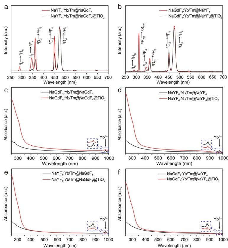
**Fig. S11** (a) Upconversion luminescence spectra of (a) NYF/NGF and NYF/NGF@TiO<sub>2</sub> in aqueous solution, (b) NGF/NYF and NGF/NYF@TiO<sub>2</sub> in aqueous solution. UV-vis absorption spectra of (c) NGFCS and NGFCS@TiO<sub>2</sub>, (d) NYFCS and NYFCS@TiO<sub>2</sub>, (e) NYF/NGF and NYF/NGF@TiO<sub>2</sub>, (f) NGF/NYF and NGF/NYF@TiO<sub>2</sub> in aqueous solution.
