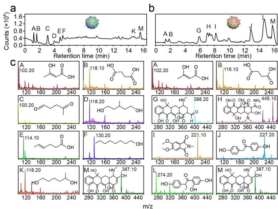
**Fig. S17** (a), (b) The respective liquid chromatograms patterns for the intermediate products of TC catalyzed by NGFCS@TiO<sub>2</sub> and NYFCS@TiO<sub>2</sub>, after 30 minutes under 980-nm light irradiation. (c) The corresponding ESI mass spectra of the intermediates detected in (a) and (b).
