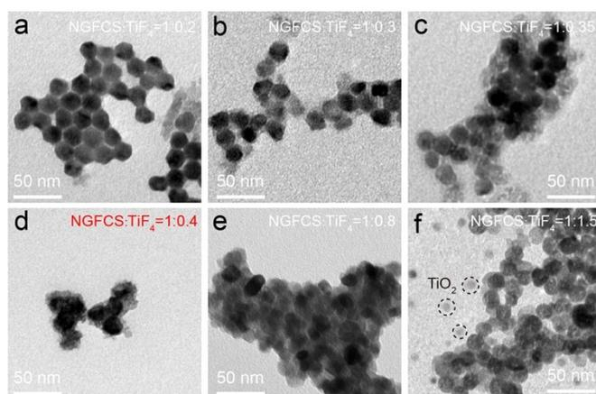
**Fig. S2** TEM images of  $\text{NaGdF}_4:\text{Yb}/\text{Tm}@ \text{NaGdF}_4@ \text{TiO}_2$  with different ratios of NGFCS to  $\text{TiF}_4$ . The molar ratio of NGFCS to  $\text{TiF}_4$  is (a) 1:0.2, (b) 1:0.3, (c) 1:0.35, (d) 1:0.4, (e) 1:0.8, (f) 1:1.5.
