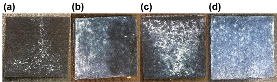
**Figure S1.** Optical images of the EPD deposited TiO<sub>2</sub> nanoparticles on the surface-treated polyester fabrics containing different number of LbL-assembled PDDA/PSS bilayers (fabric size: 50 mm × 50 mm): (a) 0 bilayer, (b) one bilayer, (c) two bilayers, and (d) three bilayers. It is found that increasing the number of PDDA/PSS bilayers on polyester fabric can provide sufficient electrostatic attraction for the subsequent TiO<sub>2</sub> nanoparticle deposition with uniform coverage.
