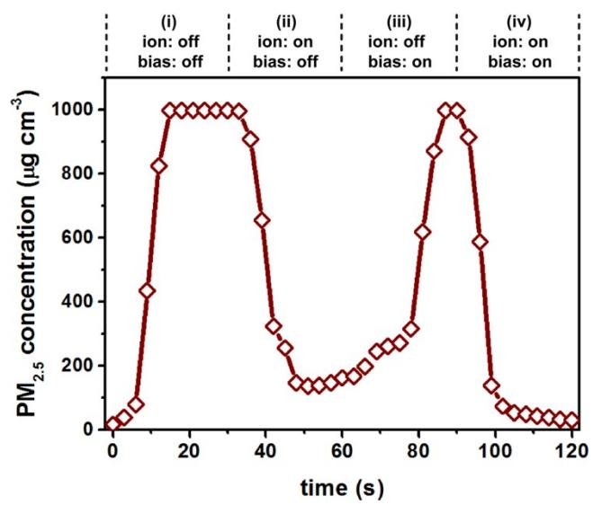
**Figure S4.** Transient evolution of  $\text{PM}_{2.5}$  concentration under different assessment conditions: (i) ionizer and filter bias both off, (ii) only ionizer on (-10 V), (iii) only filter bias on (500 V), and (iv) ionizer and filter bias both on.
