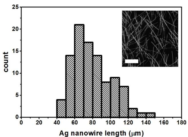
**Figure S3.** Histograms of length distribution of Ag nanowires. Inset: SEM image of as-prepared Ag nanowires with average length of  $\sim 70\text{--}80 \mu\text{m}$  and diameter of  $\sim 200 \text{ nm}$  (scale bar:  $50 \mu\text{m}$ ).
