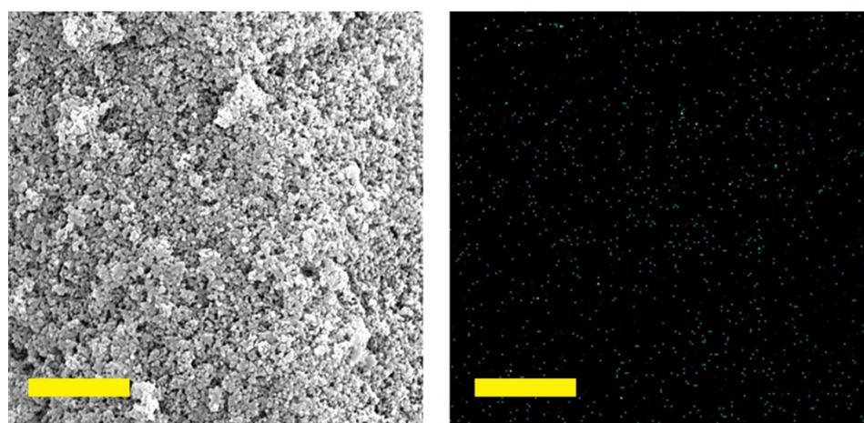
**Figure S2.** SEM image of the deposited photocatalyst TiO<sub>2</sub> nanoparticles on the PDDA/PSS-treated polyester fabrics and its corresponding energy-dispersive x-ray diffraction (EDX) mapping image of titanium element (scale bar: 2  $\mu\text{m}$ ).
